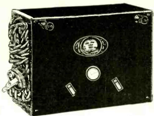
The new Bernard Universal Test Oscillator, fundamentals 132-380 kc, for lining up intermediate frequencies, 132 to 500 kc, and broadcast band, from a direct-reading dial. Special method permits calibrating short-wave frequencies.
