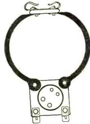
FIG. 3 This shows the essential construction of the one-tube ultra-short-wave oscillator of Lieut. Wenstrom. The heavy black lines are the plate and grid inductances.
