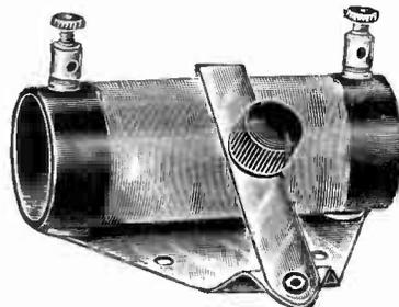
Remove aerial lead from set. Connect aerial instead to one of the binding posts of the Aerial Tuner. Connect the other binding post of the Aerial Tuner to antenna post of your set. Then move the lever of the Aerial Tuner until any weak station comes in loudest. The lever need not be moved for every different frequency tuned in. The Aerial Tuner acts as an antenna loading coil and puts the antenna's frequency at any frequency in the broadcast band that you desire to build up. Price, 85c.
