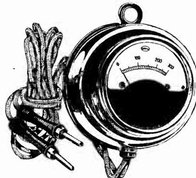
0-300 volts, at 200 ohms resistance per volt, 5 ma. drain at full-scale deflection. Accuracy, 2%. Case is full nickel finish. Long connecting cords have especially ornamental tip holders. Meter should be read in perpendicular position. Five-day money-back guaranty. Order Cat. F-300 @ \$2.59.
