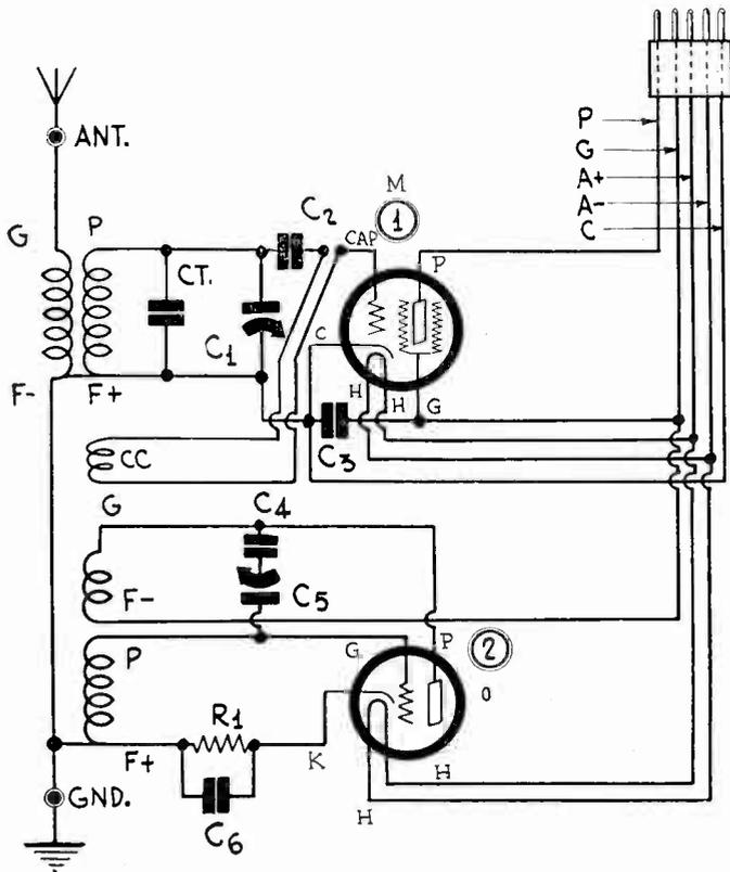
AN EXTRA COUPLING COIL, CC, IS SHOWN IN THIS SCHEMATIC DIAGRAM OF A SHORT-WAVE ADAPTER FOR AN AC SCREEN GRID RECEIVER.
