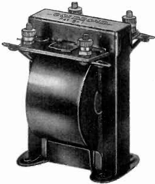
Audio frequency coupling transformers with high impedance primaries and secondaries are made in two models and two ratios of each model. At left is the "Gold Bond" shielded type, at right the "Universal" unshielded type for subpanel mounting, overall height 2 1/4". The ratios are 1-to-3 and 1-to-5, primary to secondary.
