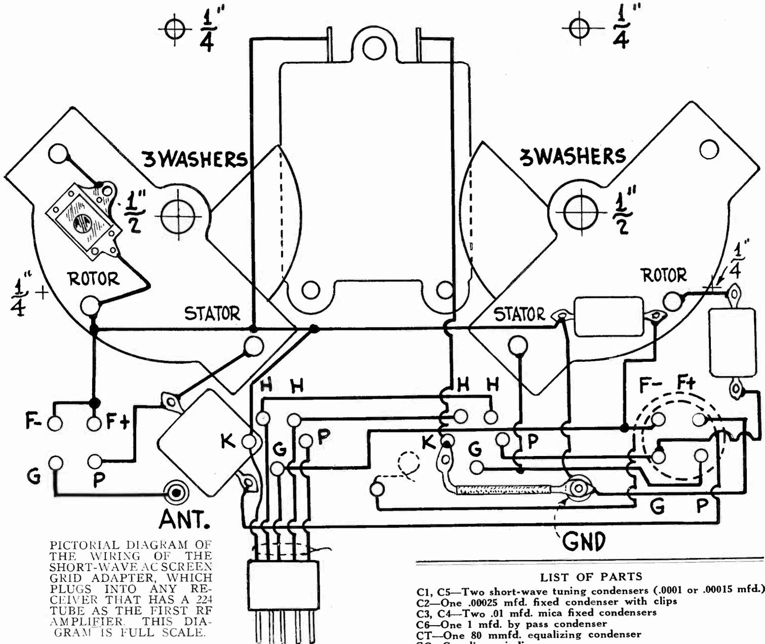
PICTORIAL DIAGRAM OF THE WIRING OF THE SHORT-WAVE AC SCREEN GRID ADAPTER, WHICH PLUGS INTO ANY RECEIVER THAT HAS A 224 TUBE AS THE FIRST AMPLIFIER. THIS DIAGRAM IS FULL SCALE.
