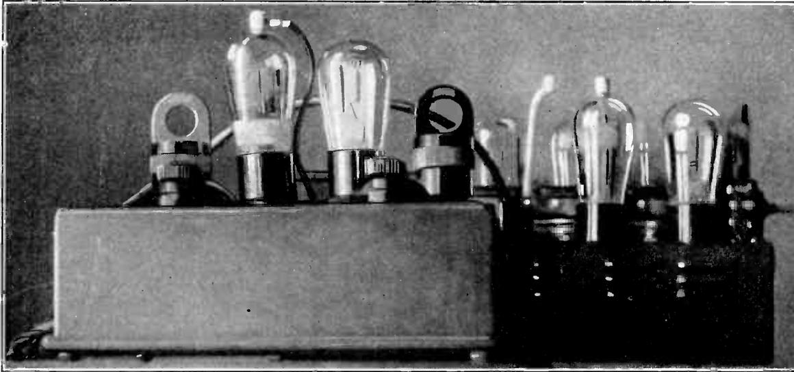
THE ADAPTER HOOKED UP TO A TWO-STAGE SCREEN GRID RF RECEIVER, THE 6-TUBE NJ-30 OF THE JACKSON LABORATORIES, ON WHICH IT WORKED FAIRLY WELL. THE SIXTH TUBE IS THE 280.
