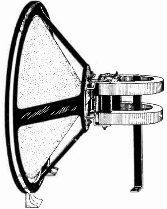
Farrand Inductor Chassis, consisting of the unit, cone, spider, bracket, assembled, but not in a cabinet.
