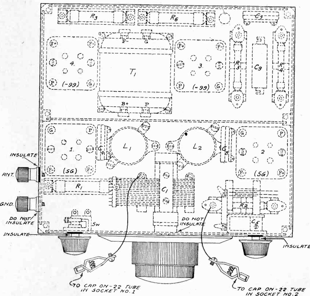
**THE FRONT AND THE LAYOUT OF PARTS OF THE DOUBLE SHIELD PORTABLE ARE SHOWN HALF-SCALE. THE RECEIVER, CONSISTING OF FOUR TUBES, IS IN ONE SHIELD. ANOTHER SHIELD (NOT SHOWN) CONTAINS THE BATTERIES.**
