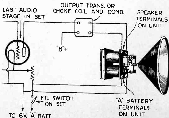
The method of connecting the A battery to the unit. If a trickle charger is used, the A battery terminals on the unit are connected to the charger instead of to the set switch.
