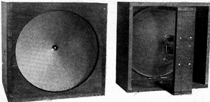
FRONT AND BACK VIEWS OF THE COMPLETED SPEAKER, SHOWING METHOD OF MOUNTING UNIT AND CONE. NOTE DEPTH OF BOX.
