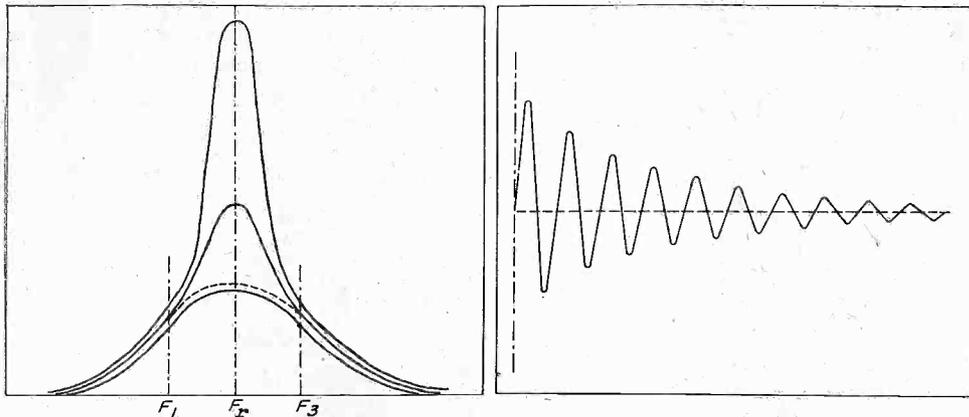
AT LEFT ARE THREE DIFFERENT RESONANCE CURVES, INDICATING THREE DEGREES OF SELECTIVITY. THE HIGHEST IS THE MOST SELECTIVE. THE DOTTED CURVE INDICATES THE LIMITED RESPONSE DUE TO DETECTOR OVERLOADING. AT RIGHT IS REPRESENTED A DAMPED WAVE PRODUCED BY THE DISCHARGE OF A CONDENSER IN A TUNED CIRCUIT. SUCH A WAVE WILL INDUCE OSCILLATION IN A TUNED CIRCUIT EVEN IF THAT CIRCUIT HAS NOT THE SAME RESONANT FREQUENCY AS THE WAVE.
