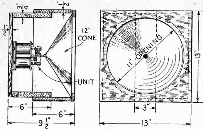
Diagram of baffle box construction, showing front and side views with exact measurements (at left).
