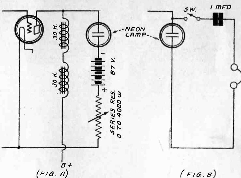
AT THE LEFT IS THE CIRCUIT DIAGRAM OF THE OUTPUT TUBE OF A RADIO RECEIVER, TO WHICH A NEON GLOW LAMP HAS BEEN CONNECTED FOR TELEVISION RECEPTION. AT RIGHT IS A DIAGRAM FOR AID IN TUNING IN A TELEVISION CARRIER. A LOUDSPEAKER OR HEADSET MAY BE CONNECTED ACROSS THE NEON LAMP FOR LISTENING TO THE CHARACTERISTIC FLUTTER.
