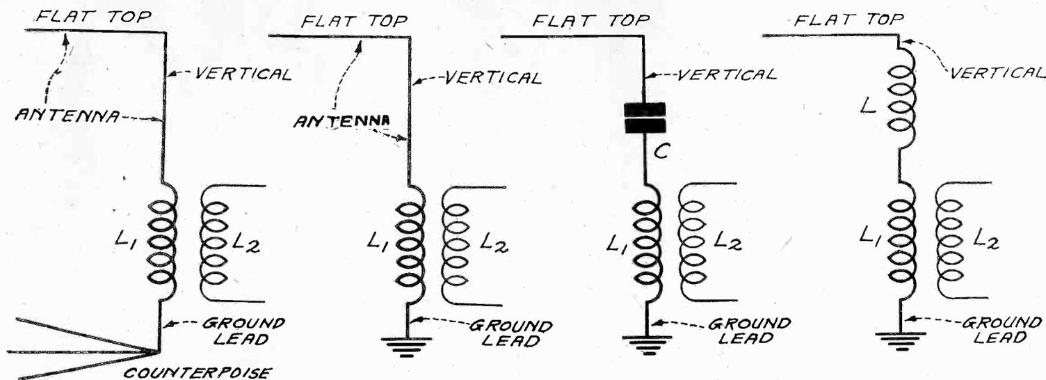
**FOUR DIFFERENT ANTENNA CIRCUITS. AT THE LEFT A REGULAR ANTENNA AND COUNTERPOISE ARE SHOWN. THIS IS PARTICULARLY SUITABLE FOR SHORT WAVES AND WHERE A GOOD GROUND IS NOT AVAILABLE. LEFT CENTER SHOWS THE REGULAR ANTENNA AND GROUND CIRCUIT. RIGHT CENTER THE SAME CONNECTION IS USED EXCEPT THAT A CONDENSER C IS INSERTED IN THE LEAD-IN TO MAKE THE CIRCUIT EFFICIENT ON SHORT BROADCAST WAVES. AT THE RIGHT THE SAME ANTENNA IS SHOWN WITH A LOADING COIL L IN THE LEAD-IN TO ADAPT CIRCUIT TO LONGER WAVES.**
