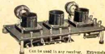
Can be used in any receiver. Extremely compact. Size 4 1/2 x 9 1/2. All strictly high class parts. Universal sockets. Distortionless transformers. Will handle the volume of any set. Only 4 connections necessary to hook up to any tuning apparatus. Color scheme binding posts, also switch and jack. Whenever a detector and two stages of audio are required you can use this splendidly made Welty Unit to decided advantage. It saves time in building. Price only \$19.50.
