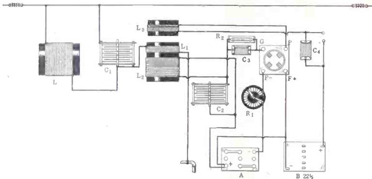
FIG. 2, the picture diagram of the receiver, which will be of material assistance to novices who desire to construct the voluminous DX set described in the accompanying article.
