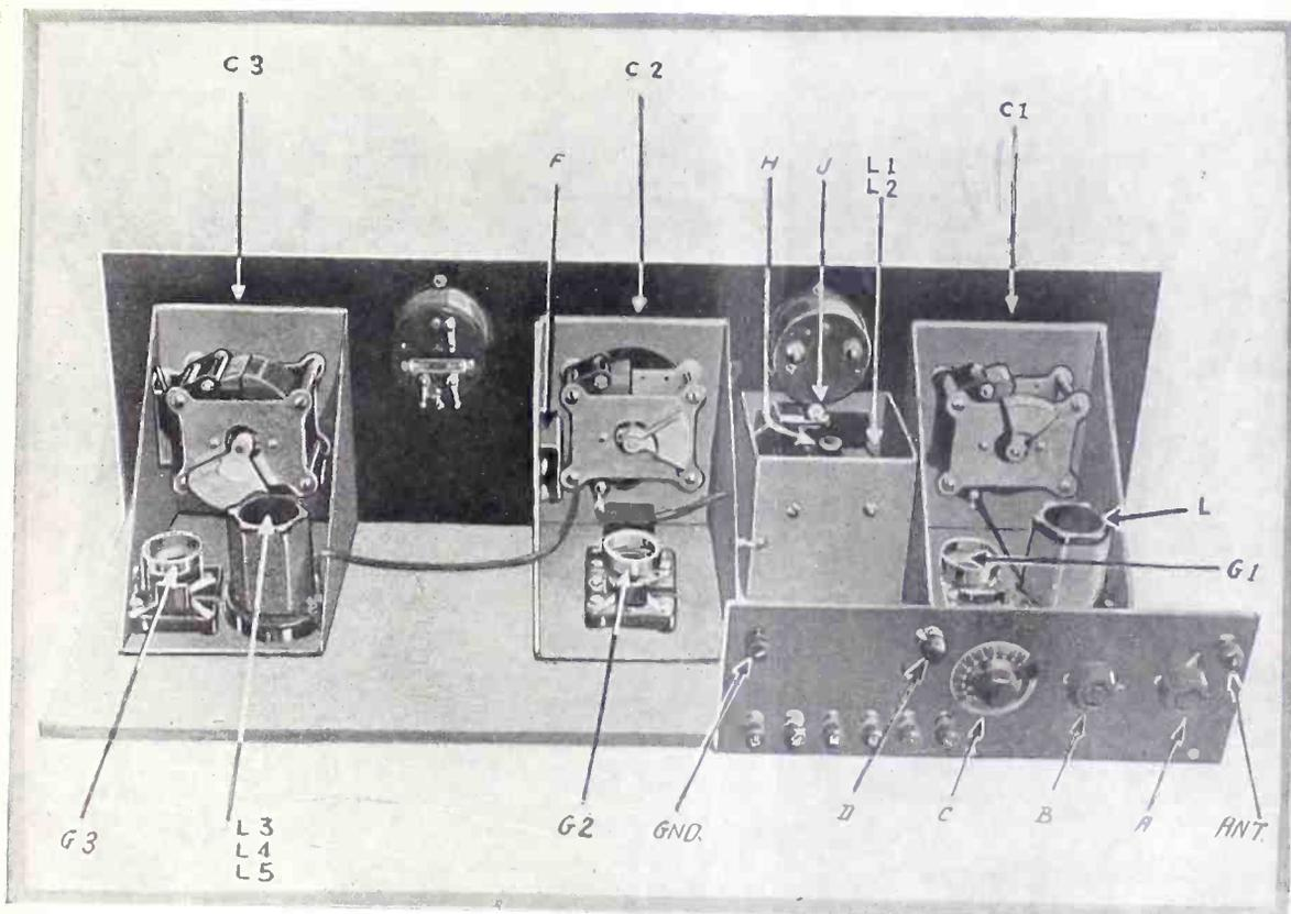
THE PARTS of the foundation unit, after assembly. The meters also are mounted.
