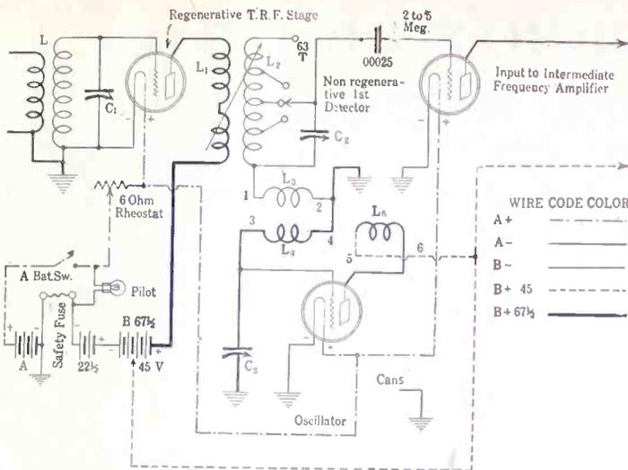
FIG. 1. The 2-to-5 meg. Leak goes from first detector grid to A+.
