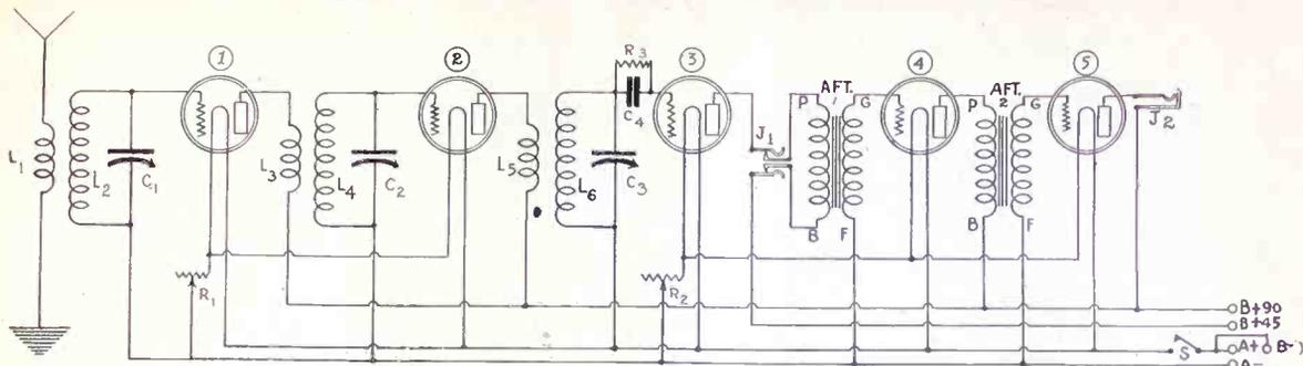
FIG. 256 showing the 5-tube TRF receiver.
