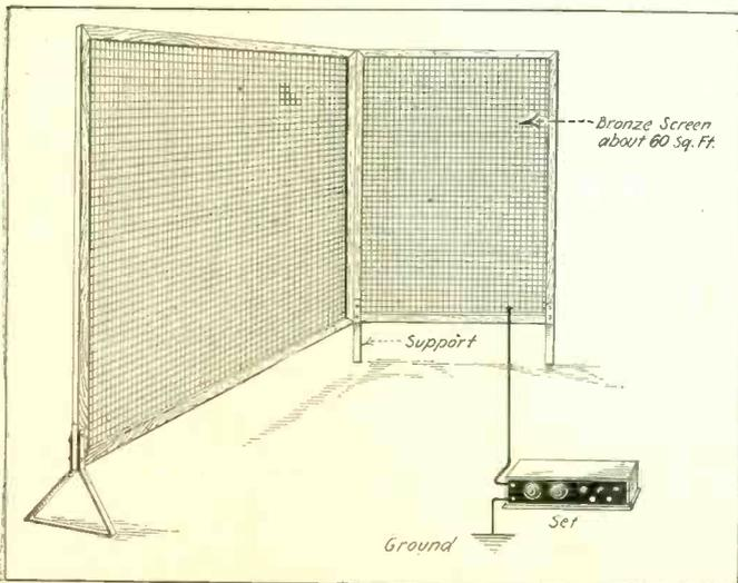
FIG. 7 is another adaptation of the condenser type of antenna. In summer, when screen doors and porches are in use, they may be wired together and connected to the receiving set. This system works very well with almost any type of receiving set.
