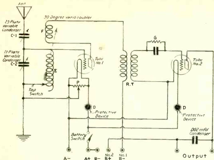
EXCELLENT DISTANCE is obtainable by this circuit, which precedes a single circuit with one stage of RF, multiplying the amplification six times.
