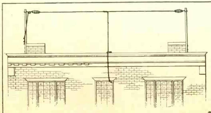
AT RIGHT—Fig. 18 shows how to use the loop antenna with a ground. The outside end is left free, and the connection to the set taken from the inside end. When used in this manner, the loop is not directional, but serves as a sort of coiled up antenna.
