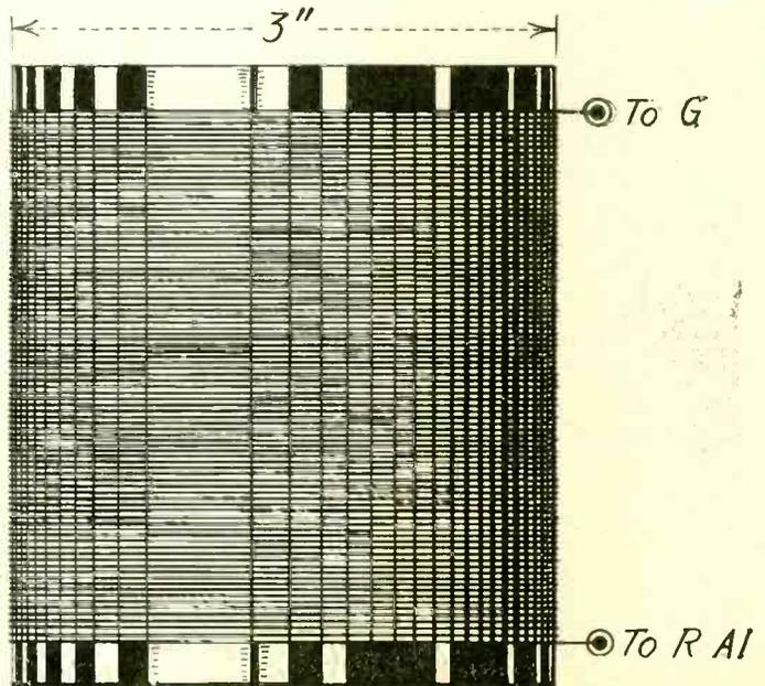
FIG. 3—The choke coil consist of 150 turns of 22 DSC wire, wound clockwise on a 3 inch tube. It is connected, one end to post G of transformer AT1 and the other end to the grid connection of socket RA1 (designated R2A1 in the diagram, Fig. 1.)
