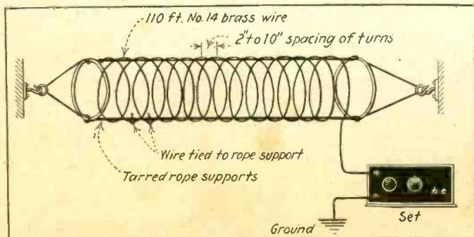
FIG. 3 is the Jeffries spiral antenna, constructed of a large coil of spring wire. This type is used in apartments where it is inconvenient to run wires to the roof. It also is popular with portable set users.
