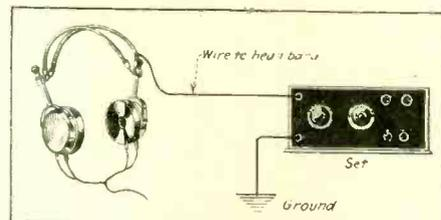
FIG. 16—Flexible wire attached to the metal headband of earphones serves as a capacity antenna. The wire to headband is indicated by the arrow. By this method the human body is used as an antenna.
