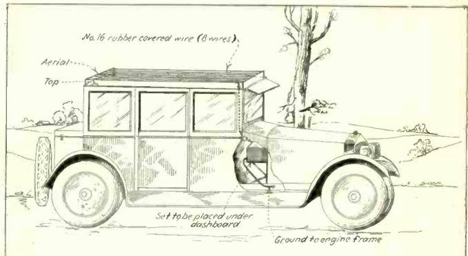
FIG. 8 shows an aerial strung on supporting insulators on the top of an auto. The ground is made to a bolt on the body of the car, which must be scraped clean to insure good contact.
