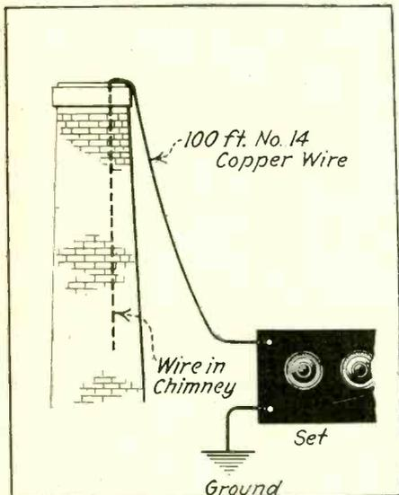
FIG. 12 pictures an arrangement which might be used in an emergency, where a high smokestack is available. This is another modification of the vertical antenna shown in Fig. 1. The top end may also be fastened to the top of the chimney. It is advisable to run the aerial on a slight slant from the top to the ground, so as to keep the wire away from the chimney to avoid absorption or obstruction to the radio waves striking the antenna.
