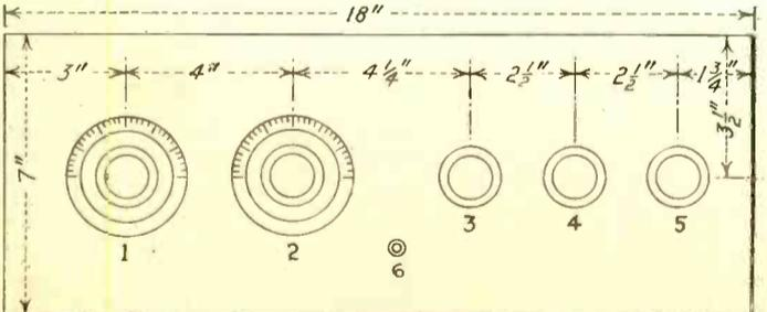
FIG. 4—Panel layout for 4-tube Super-Heterodyne.
