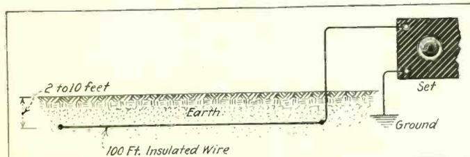
FIG. 14 illustrates a directional underground antenna. A heavily insulated wire is buried in a straight line pointing away from the direction the best broadcasting comes from. Four wires of this type, running to all points of the compass, equipped with a change-over switch, aid greatly in getting best reception.
