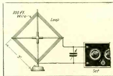
FIG. 17—Regulation 3-foot loop antenna and tuning condenser, which may be added to any regular receiving set. This arrangement works better with multi-tube outfits.
