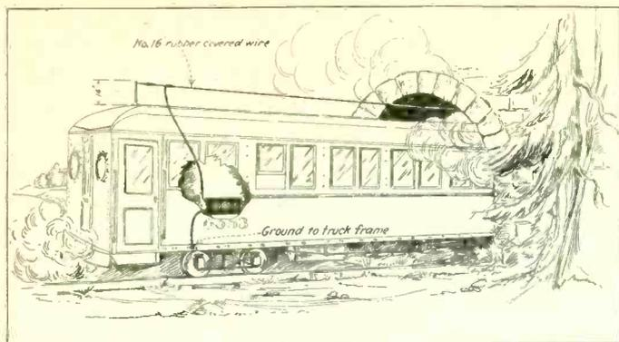
FIG. 10 is an efficient type of antenna, modifications of which are now in use on several railroad systems. Although this type has a pretty high capacity, remarkable results are obtained on sensitive sets.
