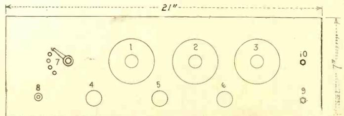
PANEL LAYOUT of the Ultra Reflex, keyed as follows: 1, first condenser, 23-plate; 2, variocoupler; 3, second condenser, 11-plate; 4, rheostat for RF tube; 5, rheostat for T2A1 tube; 6, rheostat for A2 tube; 7, tap switch; 8, battery switch; 9, phone jack, and, 10, loud speaker jack. (Fig. 4.)
