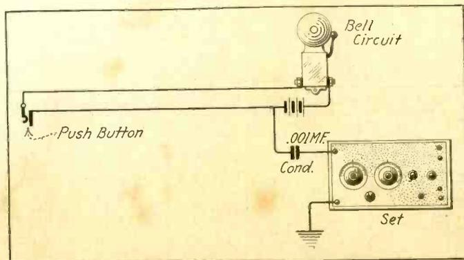
FIG. 4 shows the house bell wiring system used as an indoor antenna. The fixed condenser should always be used here in series with the antenna binding post. It does not matter to which side of the battery the wire is connected.
