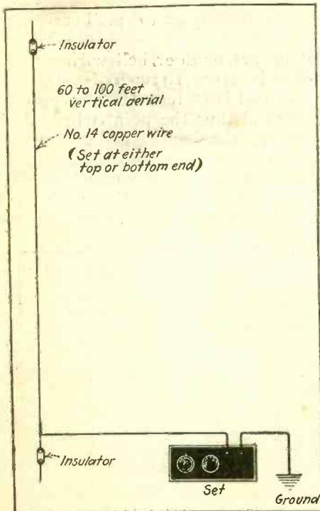
AT LEFT (Fig. 1), the vertical type of antenna. This type is not very convenient to erect in the city, unless the top of a flagpole is used to support the top aerial end. The bottom insulator should be placed about five feet from the ground to avoid absorption.
