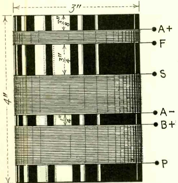
FIG. 3—Oscillator coil. C1 is the pick-up coil, 10 turns double silk-covered No. 24 wire. C2, 35 turns of the same wire spaced 3/4" from pickup coil. C3 also 35 turns of No. 24 wire spaced 1/4" from grid coil C2. The plate coil, C3, must be connected to the B+ and the plate. All coils are wound on the same 3" tube.
