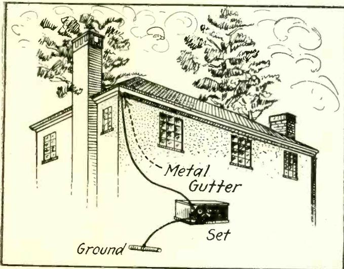
FIG. 6 utilizes the metal rain gutter which is on every house of this type. Care should be taken that the drain spout does not touch the ground, as this would short circuit the gutter antenna.
