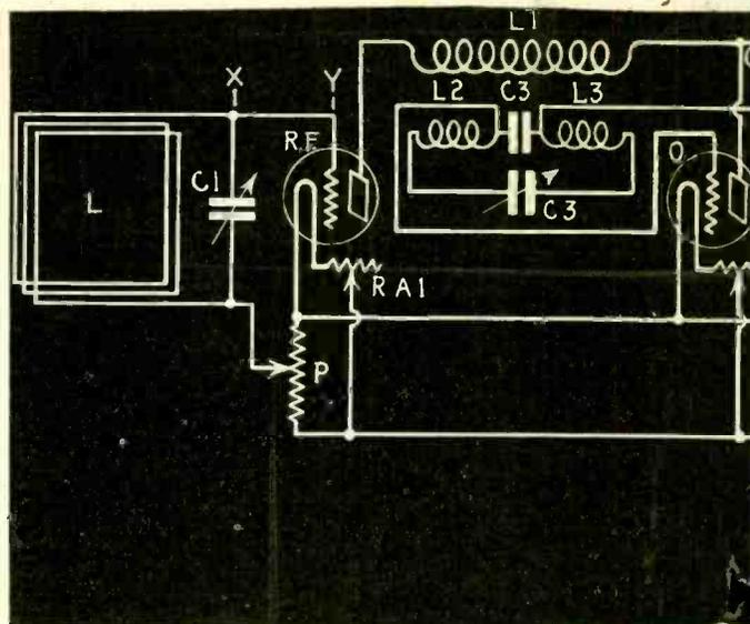
THE WIRING OF the Four-Tube Super-Heterodyne (Fig. 1), shows the... greater distance; C1, 17-plate variable condenser; RF, radio-frequency tube; C3, .001 fixed condenser; O, oscillator tube; R2, RA2, rheostats; AFT, audio-frequency transformer; J1, double
