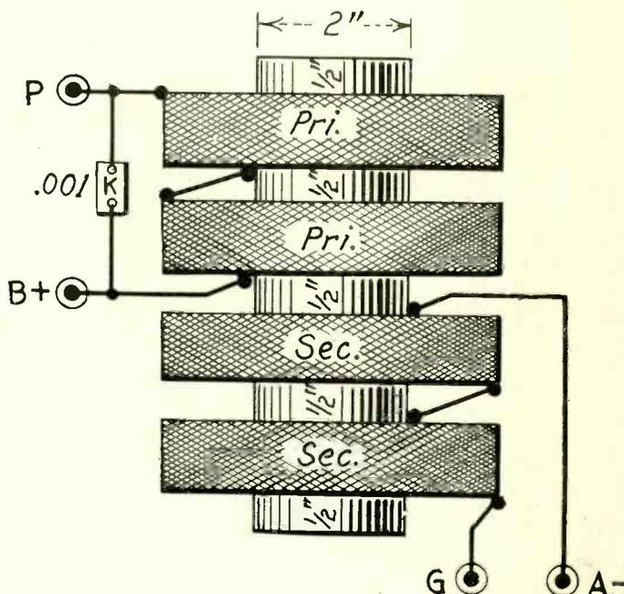
FIG 2—Honeycomb coil for B. J. Bongart's remarkable Super-Heterodyne. It consists of four 1,500-turn HC coils, the two primary coils interconnected and shunted with a .001 fixed condenser. The secondary coils also are connected in series. Each coil is 1/2" from its neighbor. The tube is 2" wide.
