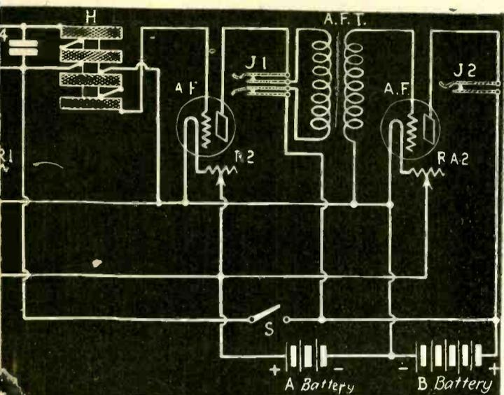
Diagram showing: L, loop; XY, lead, in which optional variometer may be inserted for regeneration; RA1, rheostat; P, potentiometer; L1, L2, L3, oscillator coil (see Fig. 3); C1, C2, C3, .001 fixed condensers; H, honeycomb coils (see Fig. 2); AF, audio-frequency transformer; J1, J2, circuit jacks; S, battery switch.
