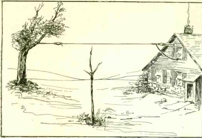
FIG. 5 is the typical type antenna used in the suburbs, running from the attic window to a tree in the back yard. Slack should be allowed for the swinging of the tree in a wind when erecting the aerial.
