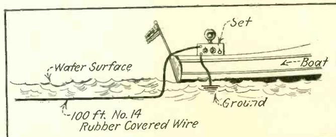
FIG. 15—An underwater aerial intercepts enough of the wave front to operate a radio-frequency set. The aerial wire is insulated water-tight. The water itself is used as a ground!
