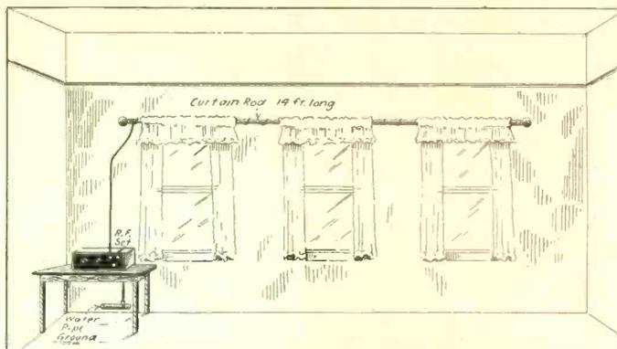
FIG. 11 shows how to use the curtain rods indoors as a substitute antenna. Many tuned radio-frequency sets work very well with only this small collector. Separate rods should be connected.
