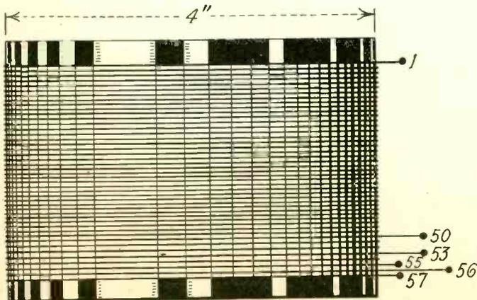
FIG. 2—Tuning coil, consisting of 57 turns of DSC wire wound clockwise on a 4-inch tube. Wind 50 turns, then tap at 50th turn. Tap also at the 53rd, 55th and 56th turns. The aerial must be connected to the binding post of the movable switch lever.
