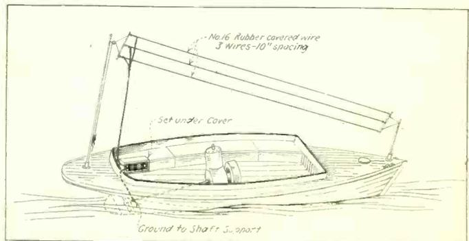
FIG. 9 is an L type of antenna, strung from bow to stern of a motor boat. One end should be at least eight feet above the deck, and the other four feet high. Ground is made to the propeller shaft.
