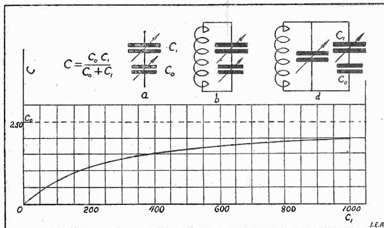
Diagrams illustrating Mr. Anderson's methods of obtaining vernier control with a 43-plate condenser.
