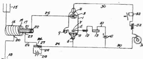
Diagram showing Pierce's method of electric current control.
