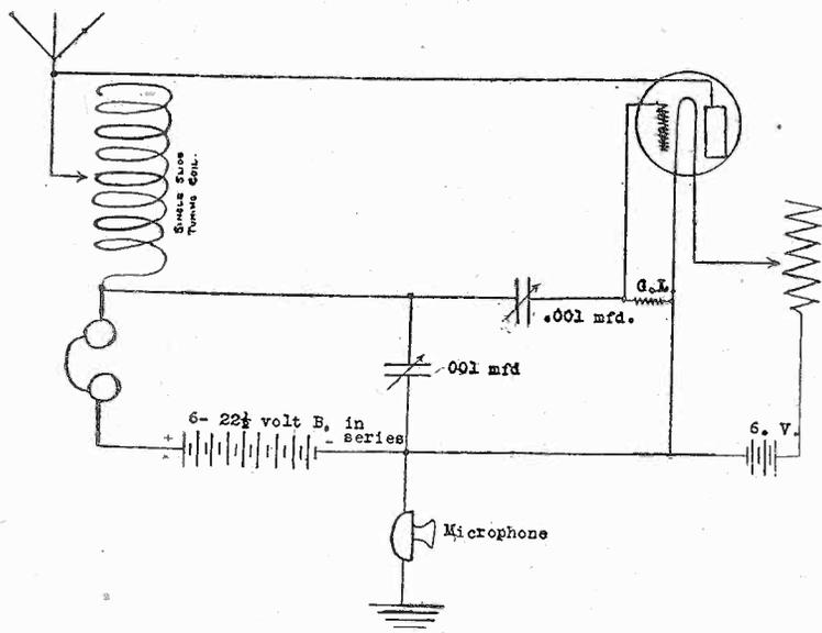
Fig. 1—Circuit diagram for a combined receiver and transmitter. When constructing this set it is best to use either a five-watt tube or one of the hard tubes, as better results will be secured.
