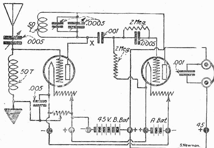
Two-tube circuit designed by A. D. Turnbull. It is one stage of tuned radio-frequency, in combination with a single circuit regenerative, and is remarkably selective and sensitive.
