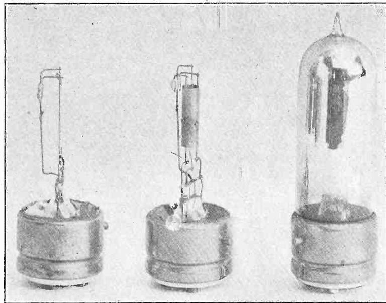
Details of new and efficient tube which operates from a flashlight battery.
