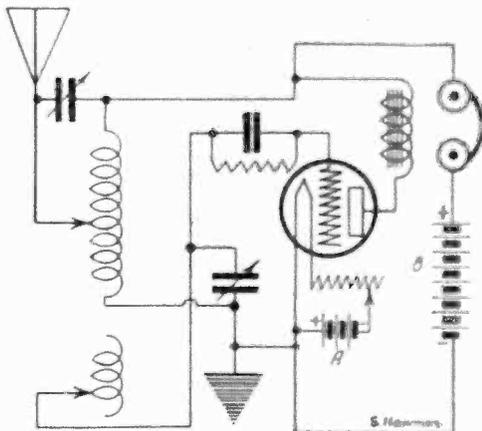
Diagram of improved Reinartz circuit as used by J. M. Freedman. The choke coil in the plate circuit is something radical in receiving circuits.
