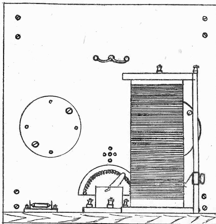
Fig. 2—Front and rear views of the panel, showing layout. The tuner is set because when transmitting a certain wave length is desired. For receiving, fine tuning can be accomplished with the condensers.
