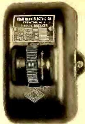
★ Magnetic circuit breakers for protecting tubes and amplifier equipment. Available in models for 50 milliamperes to 35 amps. Time-delay type trips in about 1/100 of a second on short circuit—5 seconds to 8 minutes on 125 per cent load. Instantaneous type may be adjusted for plus or minus 20 per cent of rating. Heinemann Electric Co., Trenton, N. J.—**RADIO TODAY**.
