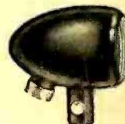
★ High-quality dynamic microphone with high or low impedance outputs. Permanent magnet excitation. Level approximately minus 55 DB. Immune to temperature changes—semi-directional. Close or distant pick-up. Weight 1½ pounds. Model D-5 50 ohms—list \$27.50. D-5-T 10,000 ohms—list \$32.50. American Microphone Co., 1915 S. Western Ave., Los Angeles, Calif.—**RADIO TODAY**—see also advt. p. 69
