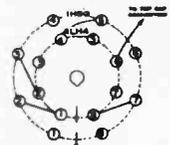
TYPE 7Y7 REPLACING TYPE 6BC7GT
