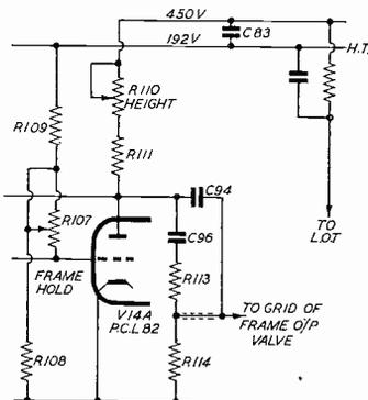
mer and is supplied via two resistors, one being the height control. This additional h.t. rail also feeds the first anode of the c.r.t. and should be about 450V.
