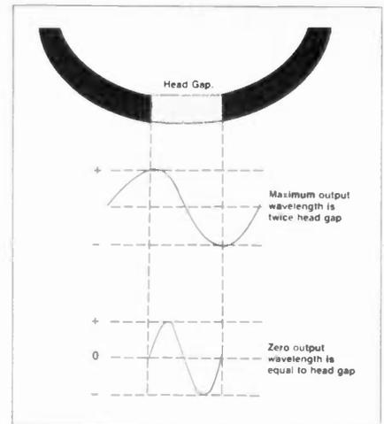
A head reaches its maximum record output and maximum playback pickup when the wavelength is twice as wide as the head-gap. Head output and pickup drop to zero when the wavelength is equal to the head-gap width. Frequencies having wavelengths longer than the head-gap width are attenuated at a 6dB per octave rate. Frequencies with wavelengths shorter than the head-gap width are attenuated from full output to zero in one octave.
