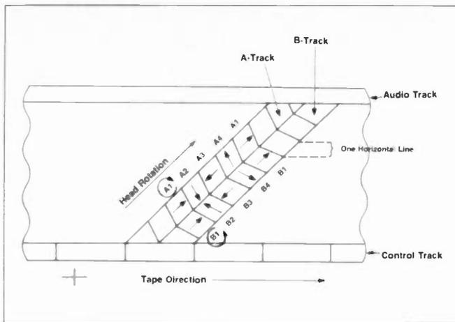
The VHS recording format eliminates crosstalk between adjacent video tracks by shifting the phase of each horizontal line. The lines of the A-track are shifted clockwise in 90° increments; those of the B-track are shifted counterclockwise in 90° increments. During playback, after the original phase relationships are reestablished, the signals are delayed by one horizontal line and fed into a comb filter which compares and eliminates the crosstalk.
