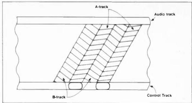
Both the VHS and Betamax formats slant the azimuths of the A- and B-heads in opposite directions. This slanting of the video heads means that the material recorded by one head is separated from the material recorded by the other by several degrees (Betamax by  $14^\circ$  and VHS by  $12^\circ$ ). This makes it less likely that the A-head will pick up anything recorded by the B-head.
