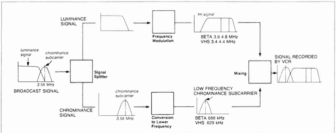
To record the broadcast television signals at the frequency response of the video heads, the VCR separates the luminance and chroma signals. There it frequency modulates the luminance signal and converts the chrominance signal down to a lower frequency. Azimuth recording prevents luminance crosstalk. During recording the initial steps are taken for the elimination of chrominance crosstalk.
