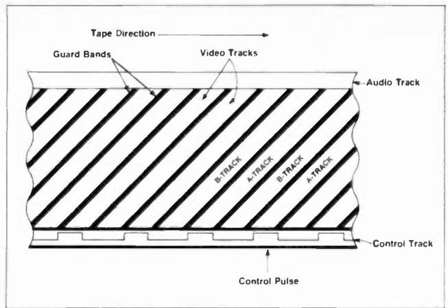
The stationary control head records a control pulse on the control track corresponding to every other video track. The VCR can then use these pulses as reference signals to align the A-head with the tracks it previously recorded.
