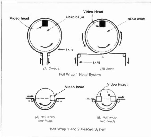
The helical scan video recording system uses either one or two video heads, and wraps tape around the head drum in one of several ways. (VHS and Beta systems use the two-headed half-wrap system or a variation of it.)
