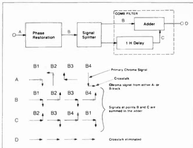
In a VHS recorder, the chroma signals that were rotated 90° clockwise or counterclockwise during recording are restored to their original phase relationships during playback. This phase restoration also changes the phase of the crosstalk. After the phase restoration, the information from the video track is split and delayed by one horizontal line. Then, when these two signals are summed in the adder, crosstalk is eliminated from the comb filter output.
