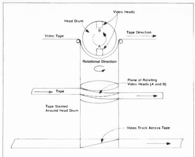
The helical scan system places two heads 180° apart on a rotating drum. The heads rotate so that one head is always in contact with the tape. Instead of longitudinal recording, however, the helical scan VCR record signals obliquely across the width of the tape. (Note: If the tape crosses the head drum from low to high, the video track recorded will be slanted the opposite of that shown in the diagram.)
