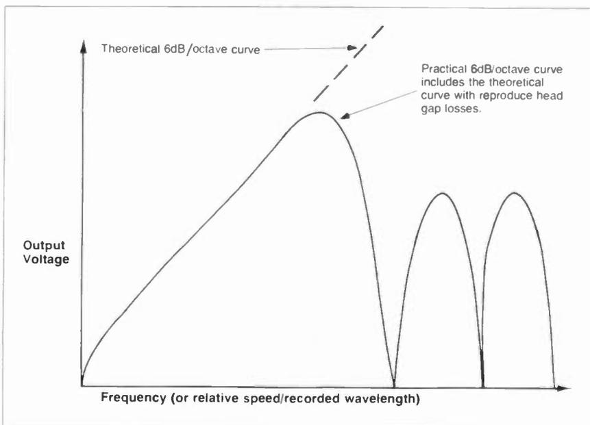
This simplified output of the 6dB/octave slope shows the rapid drop off of output signal due to head gap loss. The frequency response of any magnetic tape reproducing system is a function of the ratio of the head-gap width to the wavelength.
