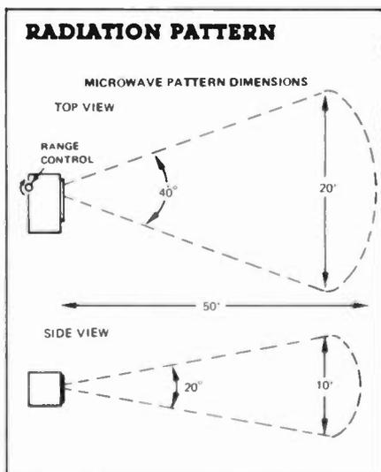
Fig. 2. The microwave pattern dimensions for the intrusion detection system.
