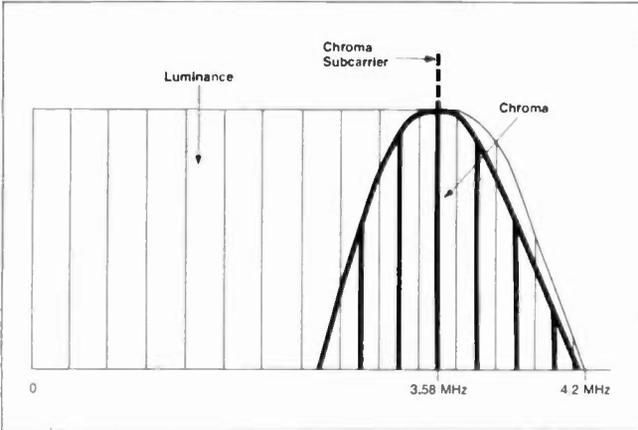
We think of the luminance and chrominance spectrums as being continuous blocks of frequency. In reality, these blocks are made up of a series of individual spikes. Frequency interleaving, the process of dovetailing these spikes, makes possible a multiplexed transmission. When a television or a VCR receiver receives the two dovetailed signals, it must separate them and independently process the luminance and chroma signals.
