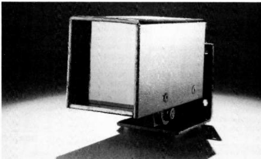
Fig. 5. The Defender D-8 microwave intrusion detector.
