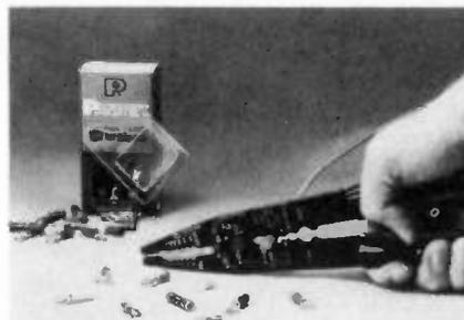
and strips wires and cuts and rethreads screws for both U.S. and metric sizes. Another feature is the plier nose for light duty use. The design of the CT-160 tool reportedly provides low crimping forces and has cushioned handles.
