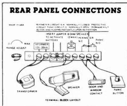
Fig. 4. A typical terminal block layout.
