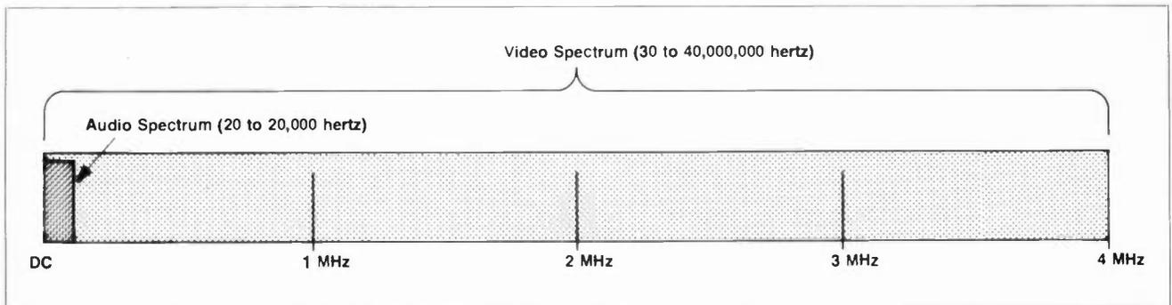
The audio spectrum is much narrower (about 20 to 20,000 hertz) than the video spectrum (about 30 to 4,000,000 hertz). The highest video frequency is about 200 times higher than the highest audio frequency.
