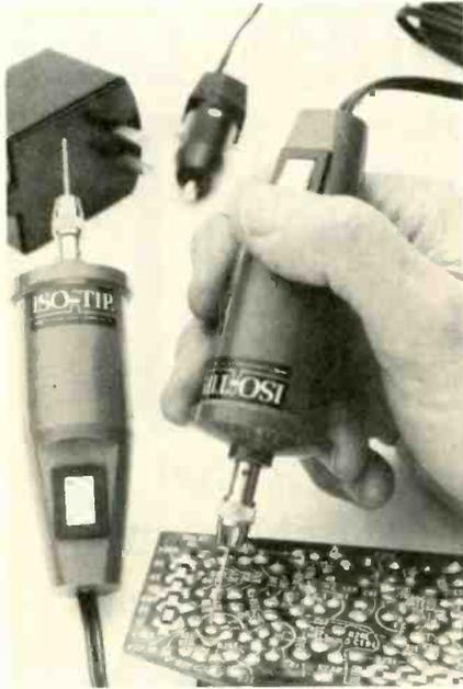
fined areas and within cabinetry. It is lightweight and has an extra-long 10 foot cord. On/off switch provides both "intermittent-on" and "locked-on" positions. It operates at approximately 9,000 RPM.
