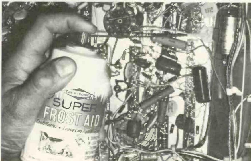
Fig. 1—The law requires that high-pressure aerosol cans, required for really fast circuit cooling, be made without seams.
