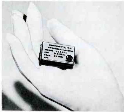
PC board mounting, the model JKTC-XO-4 is available with any output frequency between 6 and 20MHz over a temperature range of -55°C to +85°C at stability of  $1 \times 10^{-5}$ , the manufacturer says. The temperature compensating circuit is said to eliminate the need for a crystal oven — reducing warm-up time to zero and lowering input power to 100mw maximum @ 12vdc. Size is 1.5 x 1.0 x .40in. max. CTS Knights.
