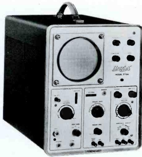
Fig. 5 — Hickok model 770A scope.
