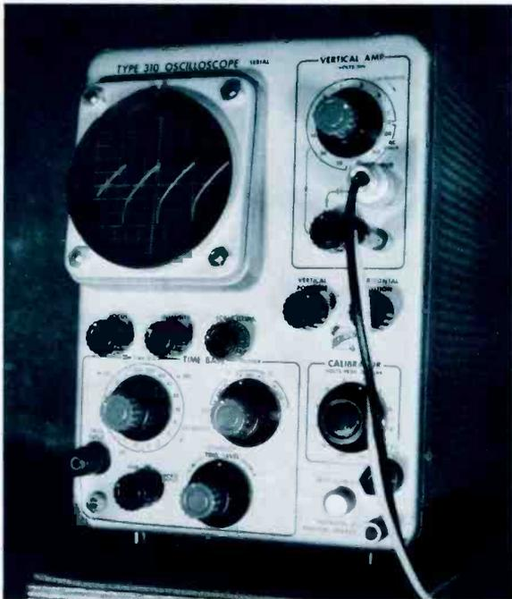
Fig. 4 — Tektronix type 310 single-channel triggered scope.
