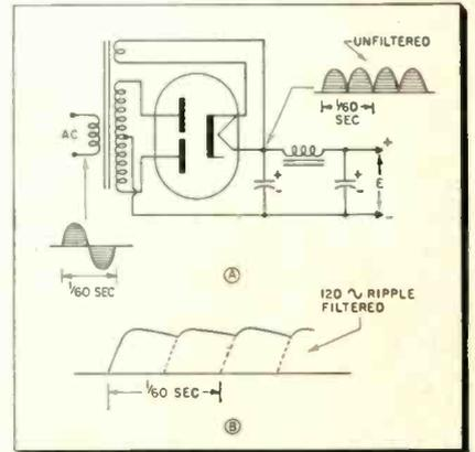
Fig. 5—Full-wave rectifier, 120 cps ripple.
