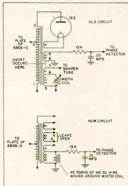
width coil, and connect the two ends of this coil between ground and phase detector input. If the picture is found to be out of phase, reverse the two coil leads, and you're back in business. There is now much less danger of subsequent break-down of the unit, because it is no longer exposed to pulse voltages as high as in the original set-up.—*John Burisin, McKees Rocks, Pa.*
