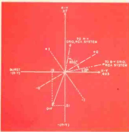
Fig. 1—The phase diagram shows how G-Y signal can be developed from R-Y and B-Y.
