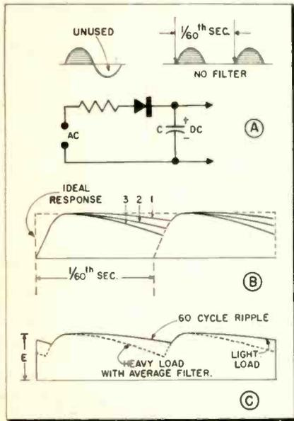
Fig. 4—Ripple filtering, half-wave rectifier.
