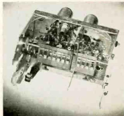
Fig. 3—Inside view of the tuner with the turret drum removed to expose the spring contacts.
