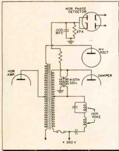
Portion of sweep-afc circuit, showing how hor. sweep signal is applied to phase detector.
