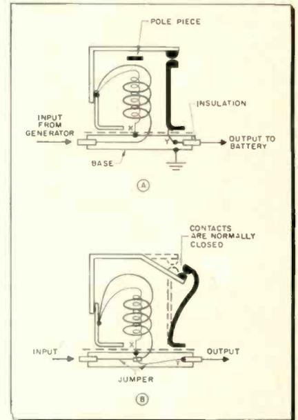
Fig. 2A—Sketch of cut-out as it originally looks. B—How cut-out looks after alteration. Note what has been done to the contacts. (A photographic view of the altered contacts is shown in Fig. 1). Note also the jumper wire that is connected between points X & Y.
