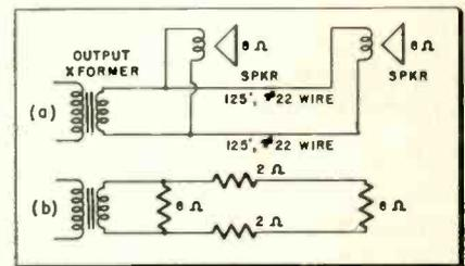
Fig. 3—Mismatch, power loss in long wires.
