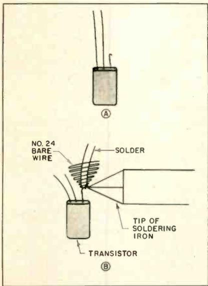
Fig. 1A—Transistor with broken lead. B—Set-up for safe additions of lead wire.
