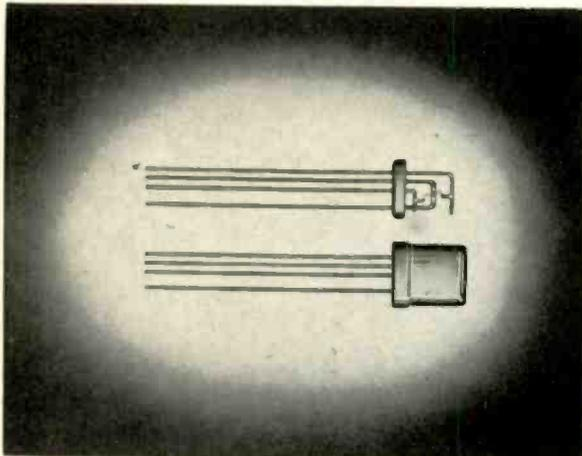
Tetrode type transistor manufactured by Germanium Products Corp.
