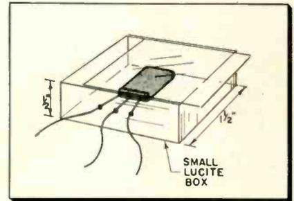
Fig. 2—Protective housing for transistors.
