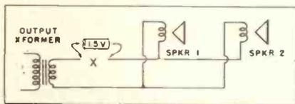
Fig. 1—Phasing speakers with flashlight cell.
