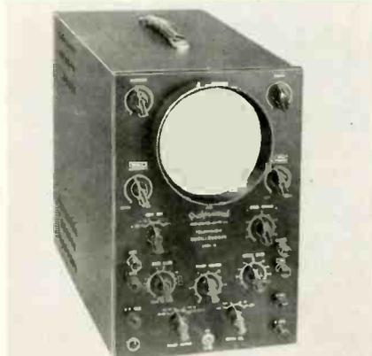
response is flat from 10 cps to 4.5 mc,  $\pm 3$ db. Four-step frequency-compensated vertical attenuator is calibrated for direct peak-to-peak voltage measurement. Sensitivity is .014 v. (rms) /in; linear sweep range 10 cps to 100 kc. Average vertical amp. input impedance is 2 meg, and 25 mmf. Price —\$147.50. Four probe accessory kit available at \$14.95. Supply Div., National Radio Institute, 16th & You Sts., NW, Washington 9, D. C.—TECHNICIAN (Ask for No. 3-43)
