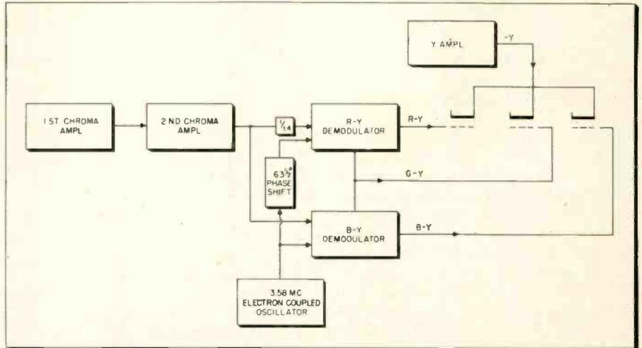
Fig. 3—Simplified block diagram of the demodulator section in the RCA receiver.
