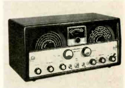
mc. Features include calibrated bandspread, "S" meter, low drift and five steps of selectivity.
