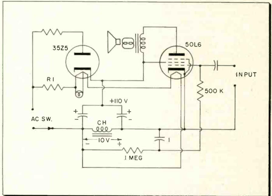
Fig. 2—Alternate circuit for single-stage phono amplifier, showing negative voltage source.
