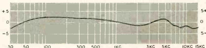
Response to new industrywide RIAA characteristic shows how 1P ceramic cartridge *self-equalizes*, because it works on "amplitude" rather than "velocity" principle. Here's startlingly improved performance for your customers' phonos!
