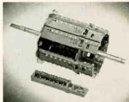
Fig. 4—New turret holds single-strip inserts for each channel with spring contact and slot.
