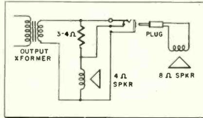
Fig. 2—Matching connection, added speaker.
