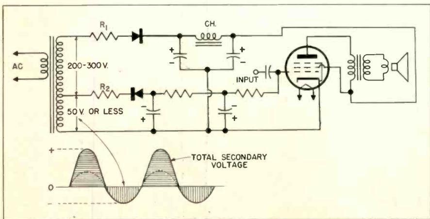
operate this tube than a comparable selenium rectifier. In addition, there are losses due to the plate-to-cathode drop in voltage.
