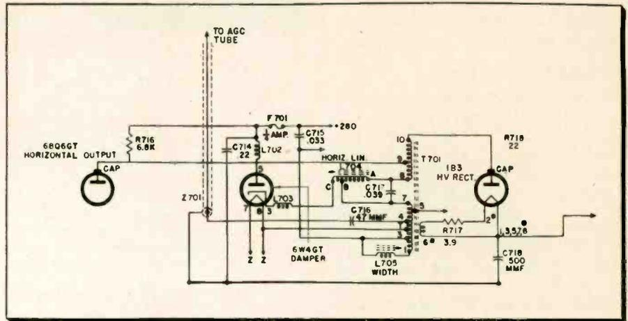
Partial schematic of Hoffman 196 chassis. Intermittent open in C-716 upset hor. sync.
