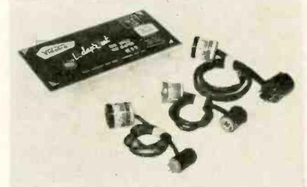
Model AT-1 is for octal tubes, model AT-2 for 7-pin miniature, and model AT-3 for 9-pin miniatures. Each unit has test points clearly numbered for easy identification. Leads are 20-in. long. Vidaire Electronics Mfg. Corp., 576 W. Merrick Rd., Lynbrook, N. Y.—TECHNICIAN (Ask for No. 3-22)
