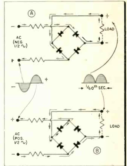
Fig. 6—Full-wave bridge rectifier circuit.
