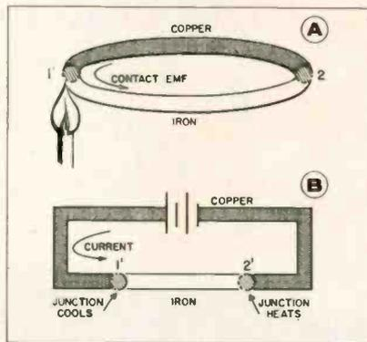
A—Seebeck effect. B—Peltier effect, with emf through metals producing cooling action.
