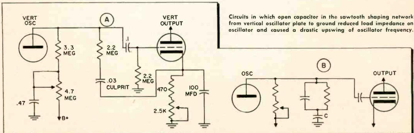
Circuits in which open capacitor in the sawtooth shaping network from vertical oscillator plate to ground reduced load impedance on oscillator and caused a drastic upswing of oscillator frequency.
