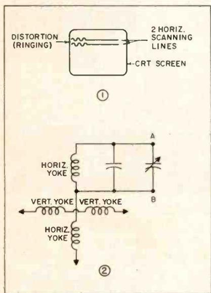
We found the solution to the problem consisted of bringing a pair of leads (A and B in sketch 2) out from the yoke coils, and connecting them to a variable condenser. This trimmer was adjusted until the rings disappeared; the amount of capacitance now present in the circuit was measured, and a condenser of that value installed in place of C-1, to cure the trouble.—Harry J. Miller, Phila. 3, Pa.
