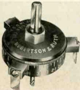
cutting blades adjust simultaneously to the size desired by rotating the dial. The dial is calibrated in standard pipe and conduit sizes, in addition to  $\frac{1}{8}$  in. spacings. Rust-proof black finish; high alloy shaft,  $\frac{3}{8}$ -in. round, with 3 flats milled for chuck mounting. Complete with 3 sets of blades for various materials. \$14.95. Robertson & Ruth, Box 534, Elmhurst, Ill.—TECHNICIAN (Ask for No. 3-44)
