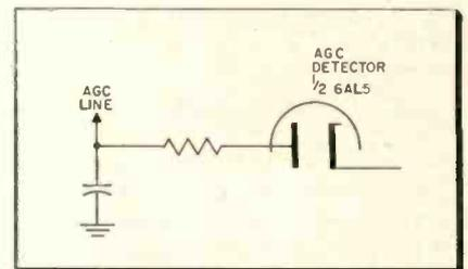
Check on each side of resistor shows fault.
