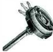
**CONTROLS**—Low power wire wound controls and rheostats are made in all needed ranges up to 10,000 ohms. They are equipped with "Silent Spiral Connector" which provides positive, continuous contact between rotor arm and end terminal. Power dissipation is 2 watts. Units are available with or without switch, and with complete assortment of shaft variations for any manufacturing or service replacement requirement. Diameter 1/4 in. by 1/8 in. depth of case.
