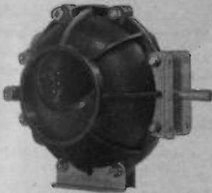
Fig. 1. Variometers Are Usually Molded in Halves
