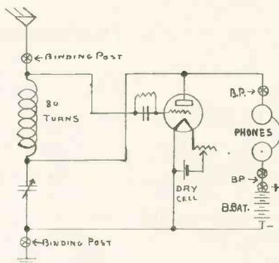
Fig. 3. Easily Made Hook-up
