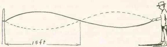
Fig. 2. Rope Oscillates as Second Harmonic
