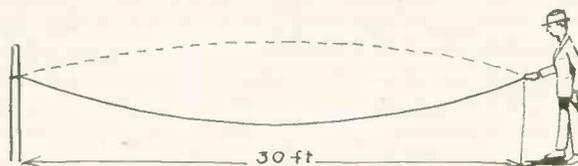
Fig. 1. Rope Vibrates as Fundamental
