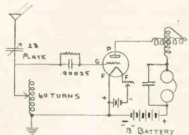
This set can be made up very cheaply and has only two controls to accomplish tuning. It will have a range of 1,000 miles, if used with a good aerial and ground. If desired, one or two audio amplifiers could be added instead of the telephone and good loud speaker action will be had.
