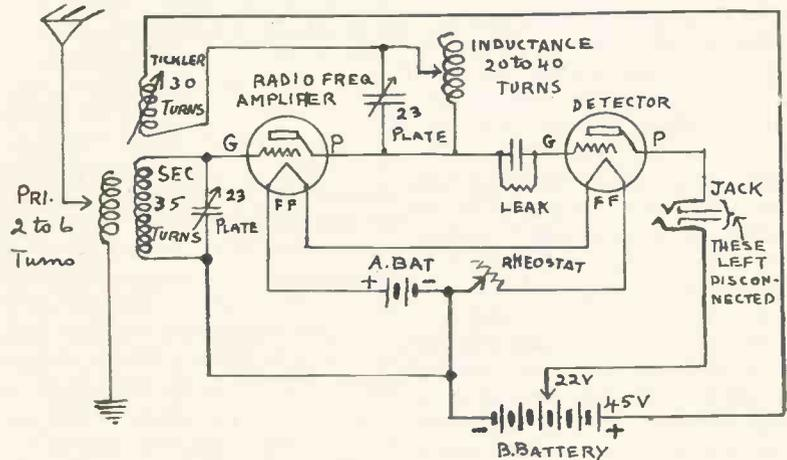
Radio Frequency Hook-up—No Transformer
