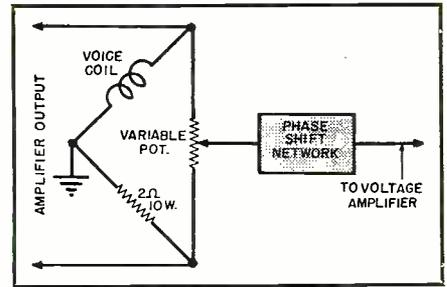
Fig. 1. Diagram of basic bridge circuit that may be incorporated in existing equipment. Care should be taken to maintain the proper phase relations throughout the circuit.
