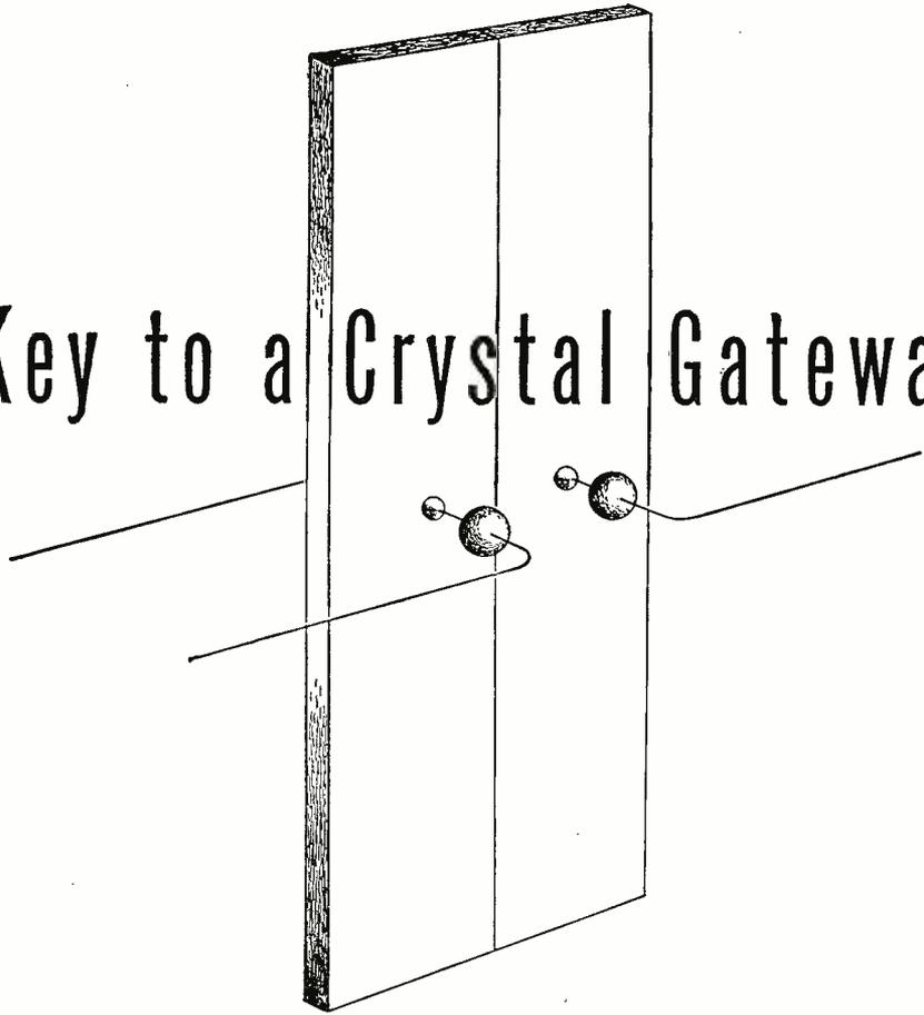
How would you solder a wire to a crystal? This must be done for most of those wafer-thin plates of quartz used in electrical circuits. They play a big part in the myriad-channel telephone system that utilizes coaxial cables.
