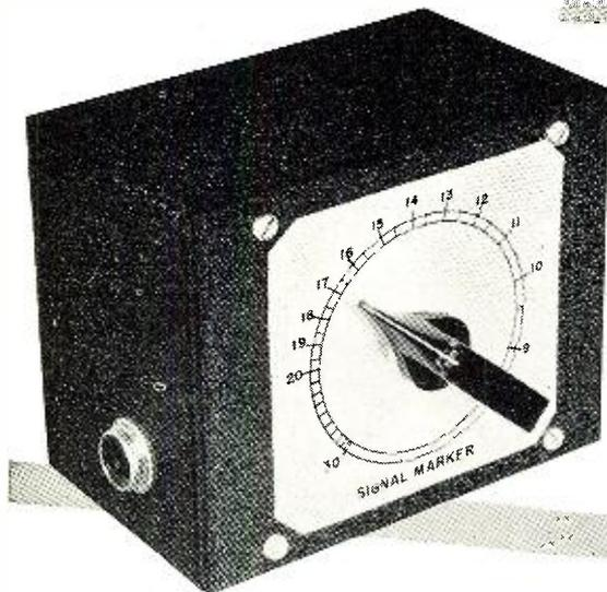
Fig. 1. External view of the completed unit. Coaxial input and output jacks are provided. The frequency dial reads from right to left in this particular unit.
