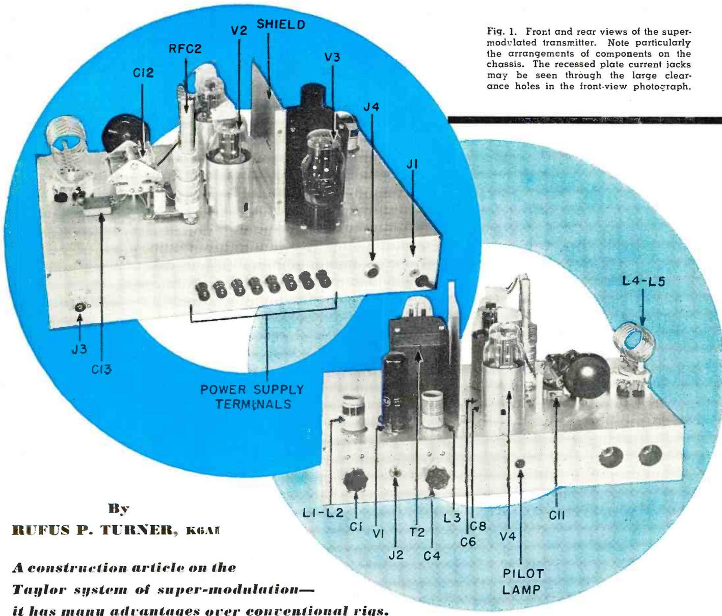
Fig. 1. Front and rear views of the super-modulated transmitter. Note particularly the arrangements of components on the chassis. The recessed plate current jacks may be seen through the large clearance holes in the front-view photograph.
