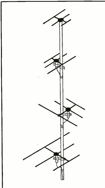
Fig. 3. A multiple-channel array which will permit reception on as many as ten channels.
