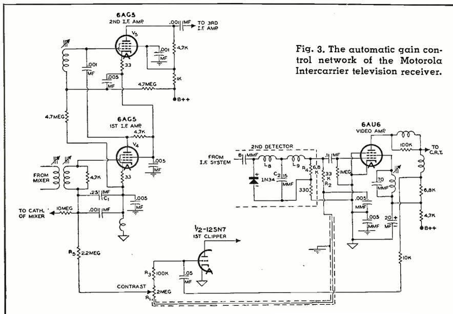
Fig. 3. The automatic gain control network of the Motorola Intercarrier television receiver.
