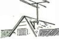
Base mounts easily on pitched surfaces... full adjustment for erecting mast and orienting antenna. NO GUY WIRES.
