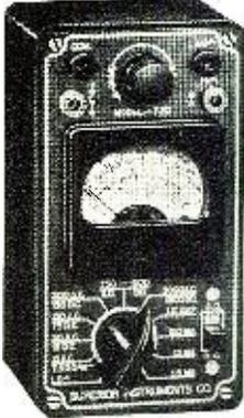
Sensitivity: 1000 ohms per v. Compact: only 3 1/4" x 5 7/8" x 2 1/4". 2% acc. 1 ma. meter. Zero adj. holds for BOTH resistance ranges. Handsome black bakelite case and etched panel. Measures the following: 6 AC ranges from 0-3,000 v. 6 DC ranges from 0-1,500 v. 4 DC current ranges 0-1.5 amps. 2 resistance ranges 0-500 ohms and 0-1 meg. Complete with test leads, batteries and operating inst., this is A BUY at only \$13.90.
