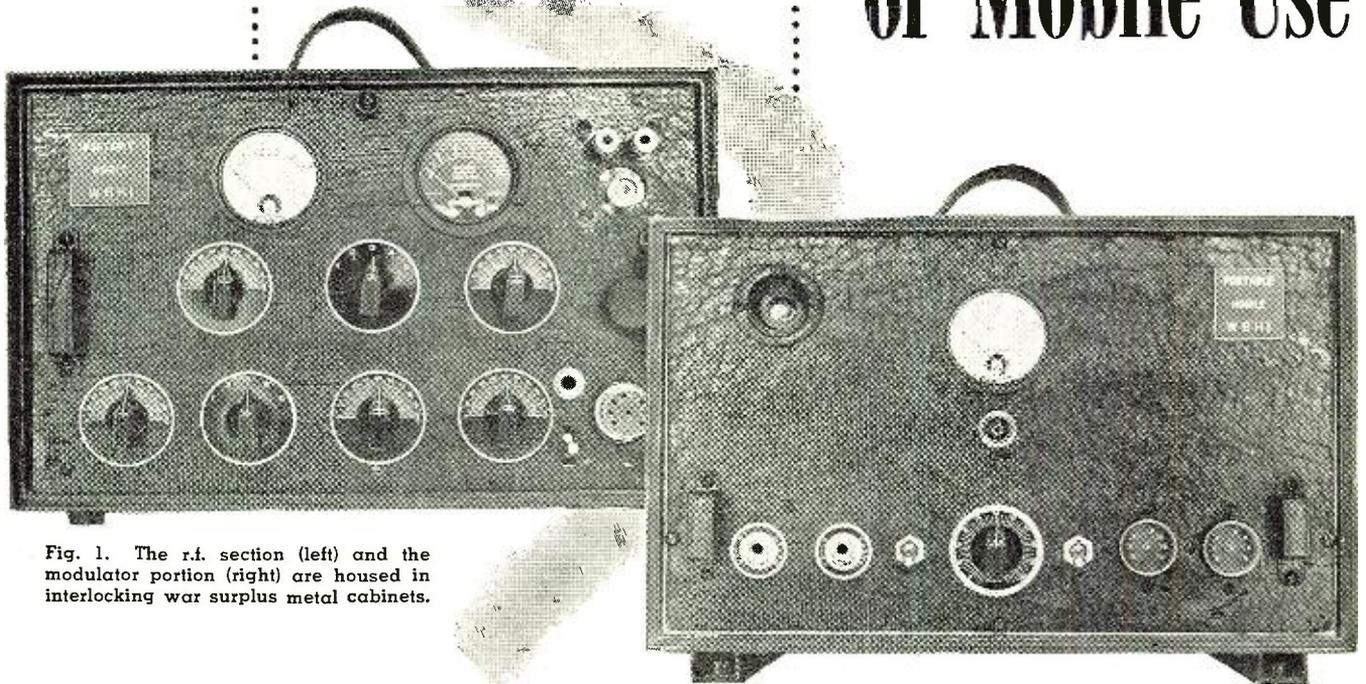
Fig. 1. The r.f. section (left) and the modulator portion (right) are housed in interlocking war surplus metal cabinets.
