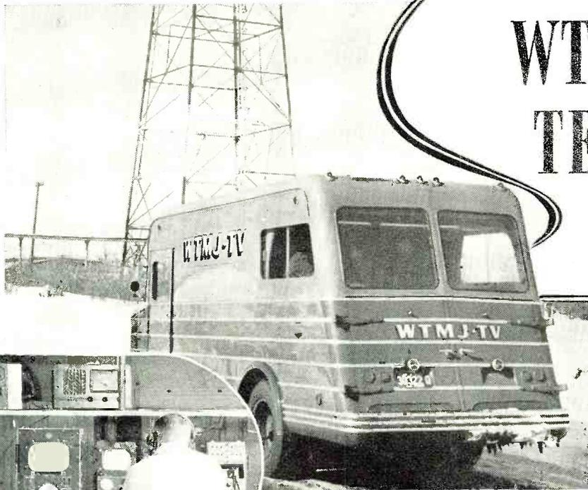
Mobile TV truck, costing \$10,000, houses all equipment necessary for remote pickups. (Left) The rear part of the truck is a complete television control room.
