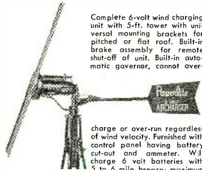
Complete 6-volt wind charging unit with 5-ft. tower with universal mounting brackets for pitched or flat roof. Built-in brake assembly for remote shut-off of unit. Built-in automatic governor, cannot over-
