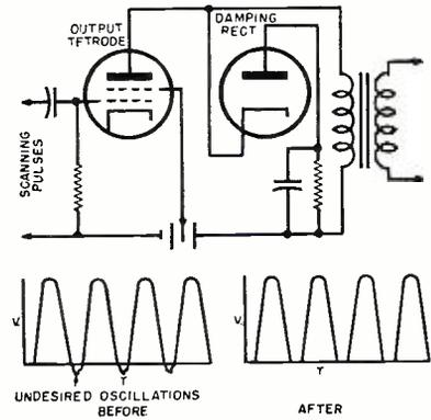
a very low impedance to the portion of the oscillation which makes its anode positive, and this energy is
