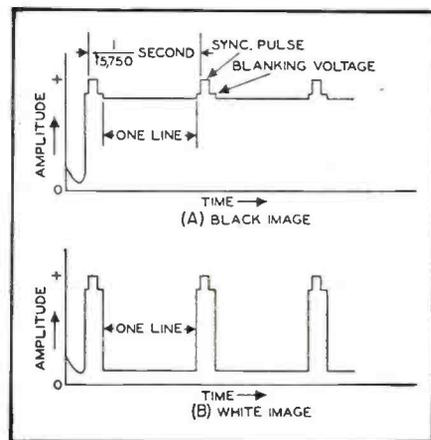
Fig. 4. The average voltage of a video signal varies with its modulation.
