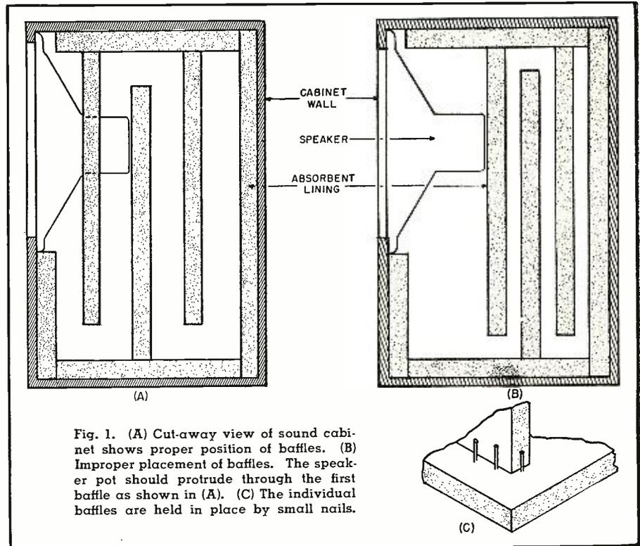
the front of the speaker diaphragm is the only sound source. A six or eight-inch speaker is entirely unsatisfactory for this type of baffle. A twelve-inch speaker will do, and a fifteen-inch speaker is still better. The larger speaker is superior in having a lower resonant frequency as a rule, but the chief advantage is in the greater maximum undistorted sound output at low frequencies. This is particularly important, for high power output is most needed at low frequencies.
