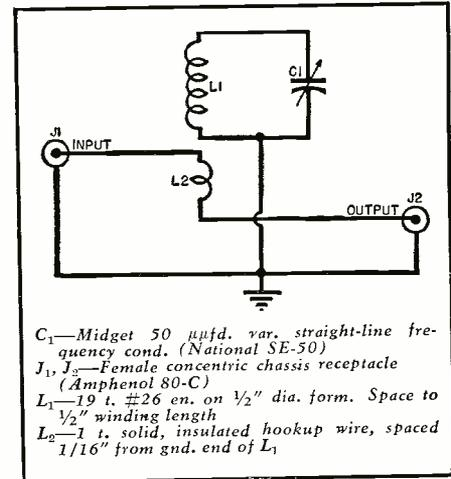
Fig. 4. Complete circuit of signal marker.
