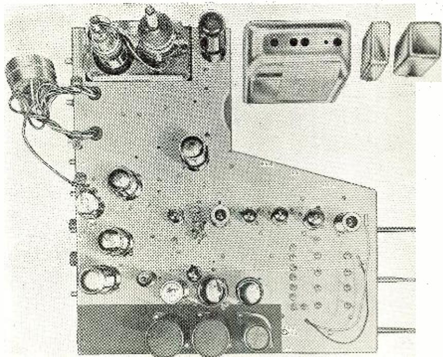
Photograph of 40-watt, dual channel amplifier incorporating wide-range volume expansion. Circuit is shown on page 146.
