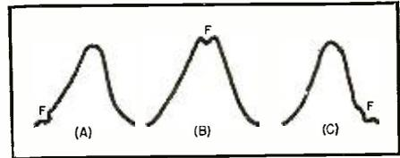
Fig. 3. Illustrating use of marker dip to determine frequencies along a typical visual alignment pattern. See text for details.
