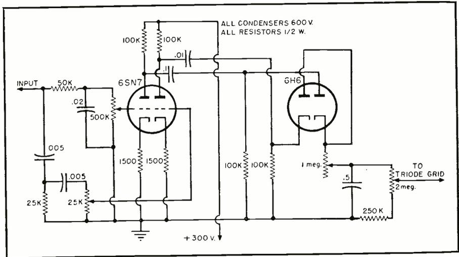
Fig. 2. Diagram of frequency discriminator system to be used in conjunction with an expander or compressor. Circuit can be used to expand highs or compress lows. Low-frequency expansion or high-frequency compression may be achieved by reversing the two diode sections. Unit also features variable attack and release controls.
