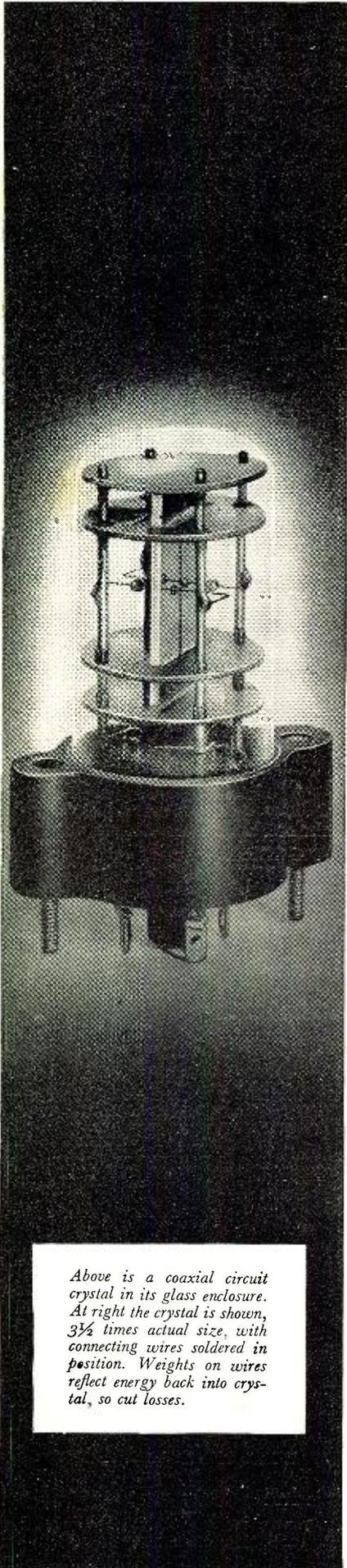
*Above is a coaxial circuit crystal in its glass enclosure. At right the crystal is shown, 3½ times actual size, with connecting wires soldered in position. Weights on wires reflect energy back into crystal, so cut losses.*
