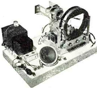
Here's the receiver chassis for your custom-made requirements. The T-64 comes complete with all parts assembled. It is the same unit as the 509 shown above with cabinet removed. T-64 has Dual Focus—your choice of a 56-inch rectangle or a 64-inch circular picture at a snap of a switch. Equipped with push button tuning. Chassis is completely assembled with all components, except CR tube.
