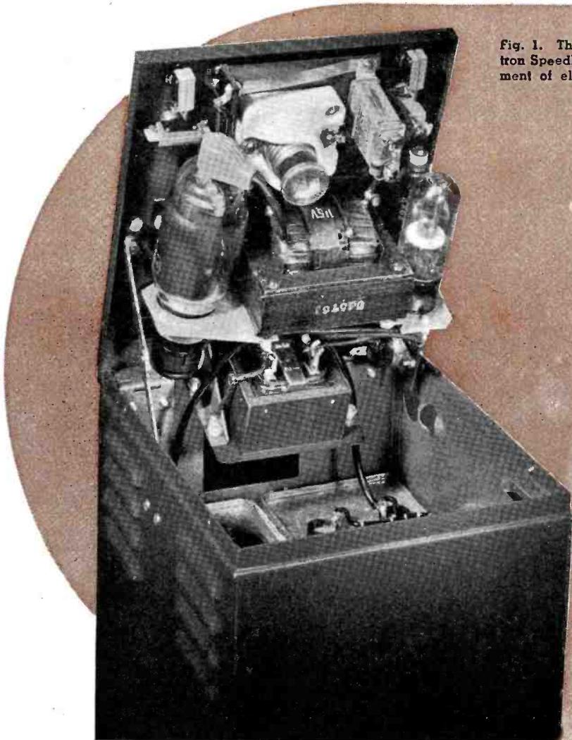
Fig. 1. The heart of the Kodatron Speedlamp, showing placement of electronic components.
