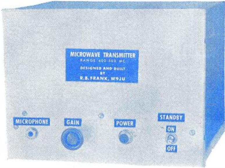
Fig. 1. Although operating at a fixed frequency, this unit may be adjusted to operate at any frequency between 400-500 mc.
