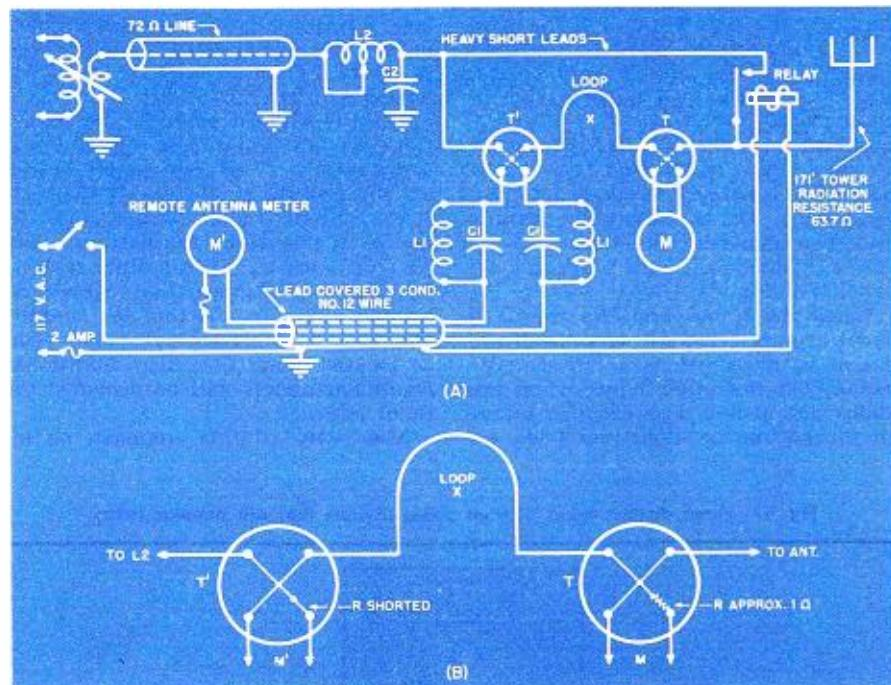
Fig. 1. Diagram showing method of wiring the remote antenna meter.
