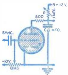
Fig. 6. Sweep circuit, using gas triode or discharge tube.
