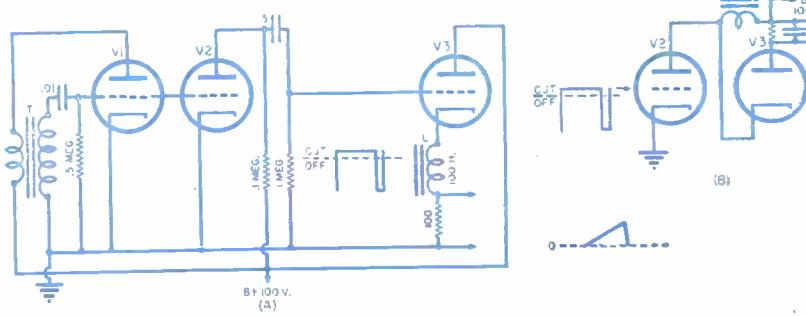
Fig. 11. (A) Blocking oscillator, amplifier, and sweep tube for linear sweep of coil current. (B) Sweep coil placed in plate circuit of V2 with damping diode.
