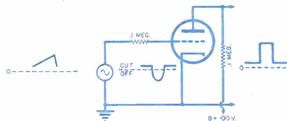
Fig. 5. Squarer circuit to substitute for first two stages of Fig. 4.
