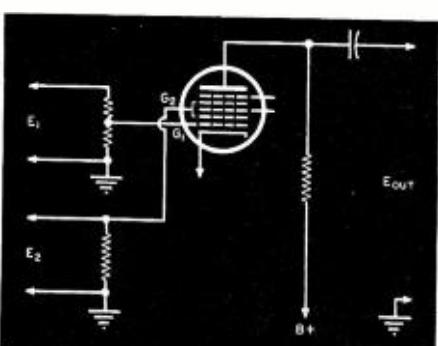
Fig. 4. Obtaining the product of two quantities.  $E_1E_2 = E_{out}$ , assuming that the gain of the tube for each input ( $G_1$  and  $G_2$ ) would be equal to one.
