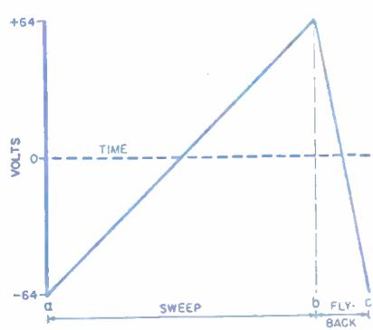
Fig. 10. Sweep voltage to horizontal plates.
