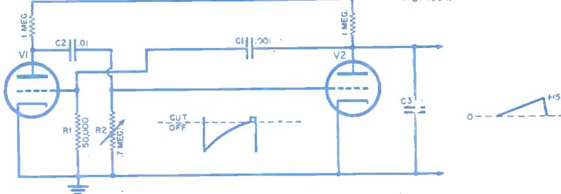
Fig. 7. Multivibrator sweep circuit showing voltage waveforms applied to grid of V2.
