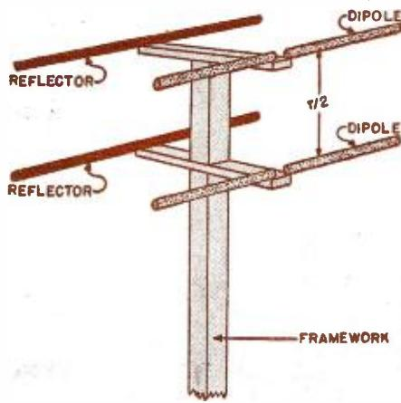
Fig. 1. Stacked array showing two dipole elements and their associated reflectors.
