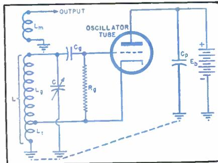
Fig. 3. Modified Hartley oscillator that enables the rotor of the tuning capacitor to be grounded.
