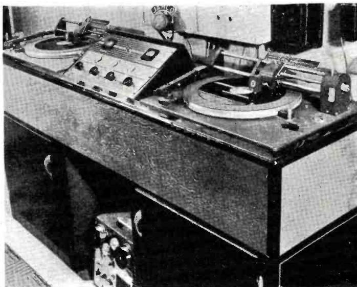
Simplified operation is the keynote of this assembly, employing two dual Radiotone recording units.
