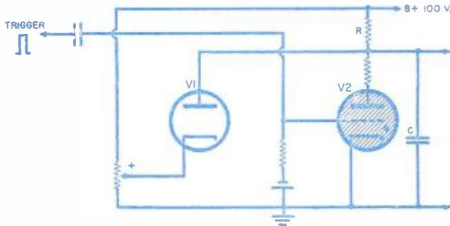
Fig. 8. Wiring diagram of gas triode single-sweep circuit.
