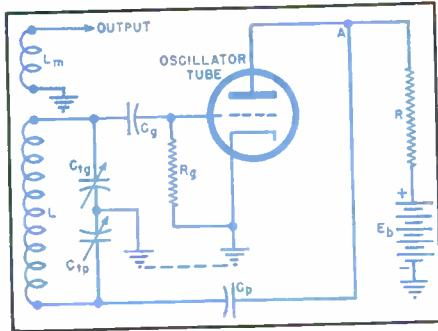
Fig. 4. Colpitts oscillator circuit in which the tank capacitance is tapped, dividing the grid and plate circuits. Capacitive feedback results.
