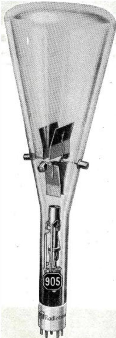
Fig. 1. An RCA five-inch high-vacuum cathode-ray tube.
