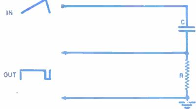
Fig. 2. Differentiating circuit to develop blanking pulse.
