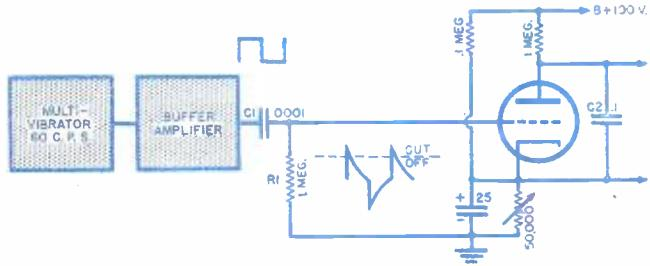
Fig. 4. Peaking circuit and biased triode for shortening fly-back time.
