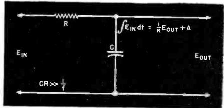
Fig. 6. Integrating circuit. In the above formula, K is a constant, depending on C, R, and frequency, while A is also a constant equal to the d.c. potential superimposed on  $E_{out}$ .
