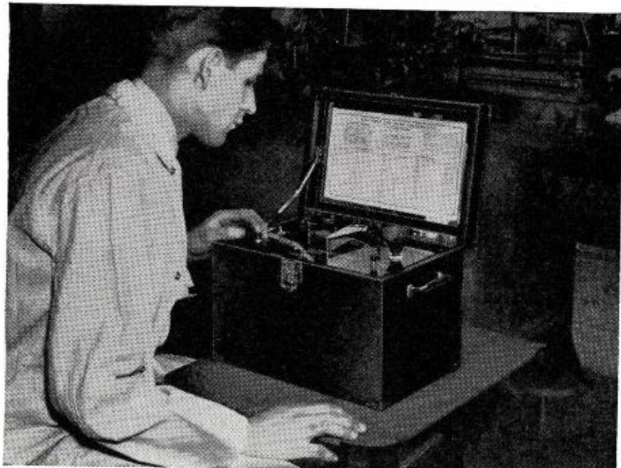
TIME-SAVING carbon content analyses of steel samples—from molten metal to report—take only five minutes with the portable, *battery-powered* Carbalyzer, produced by the Fisher Scientific Company. Leading steel firms employing open hearth or electric furnaces quickly make carbon determinations of each batch, achieving close control of quality.
