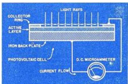
Fig. 6. Circuit of an exposure meter.
