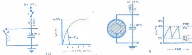
Fig. 3. (A) Mechanical switching circuit for sawtooth wave. (B) Electronic switching circuit using neon discharge tube.
