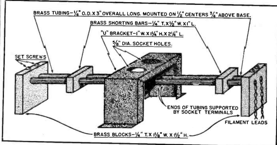
Fig. 5. Mechanical construction of the oscillator-tuning rods. The shorting bars may be varied to obtain any frequency between 400-500 megacycles.
