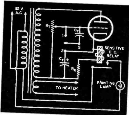
Fig. 9. Phototimer used for automatic control of lamps in enlargers and printing boxes.
