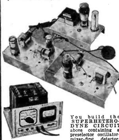
You build the SUPERHETERO-DYNE CIRCUIT above containing a preselector oscillator-mixer-first detector, i.f. stage, diode-detector-a.v.c. stage and audio stage. It will bring in local and distant stations. Get the thrill of learning at home evenings in spare time while you put the set through fascinating tests!
