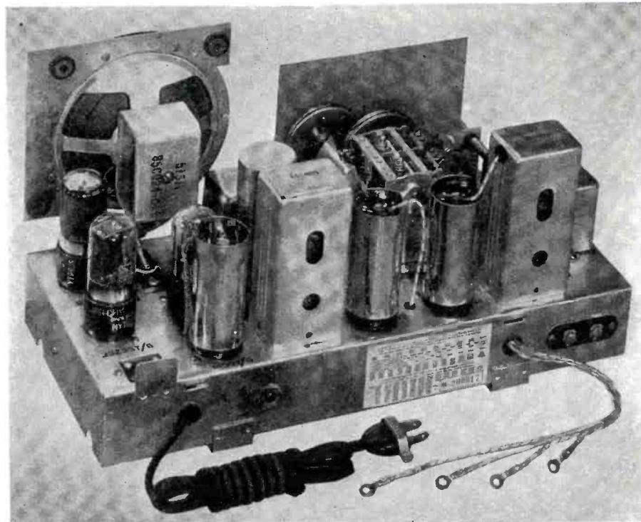
Rear view of chassis. Automatic switching from a.c.-d.c. to battery operation is accomplished by plugging the line cord into the socket at left end of chassis.
