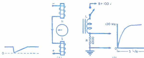
Fig. 9. (A) Position of horizontal deflection coils showing windings and current flow to deflect beam towards left. (B) Mechanical switching circuit and curve of current rise.
