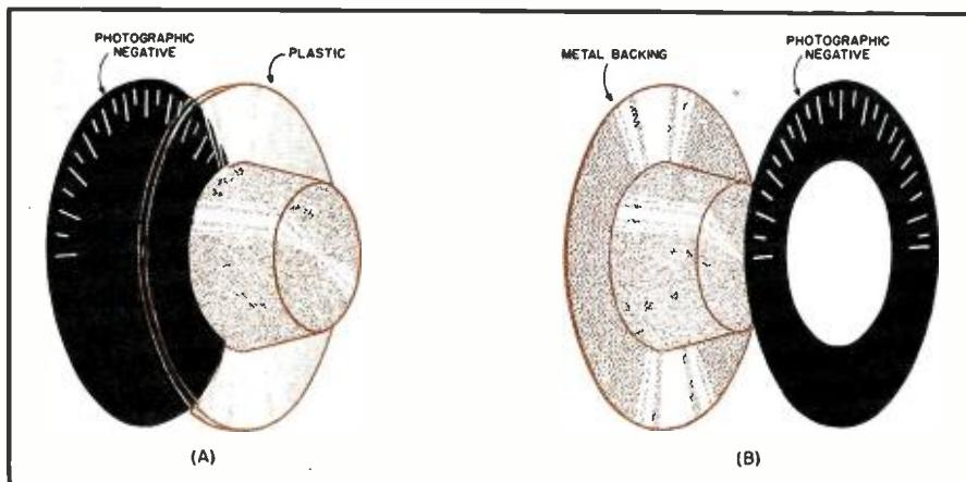
Fig. 2. Two methods of obtaining a professional-appearing calibration. (A) The photographic negative with the calibration marking appearing thereon is glued to the panel or to the back of the flange. A transparent plastic knob is used with this arrangement. (B) Photographic negative is glued directly to the knob flange.
