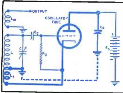
Fig. 1. A modification of the simple grid-tuned tickler-feedback circuit. Here the tickler winding is in the cathode circuit, and the tuning and feedback windings have been combined into a single-tapped coil. Feedback circuit shown by heavy lines.
