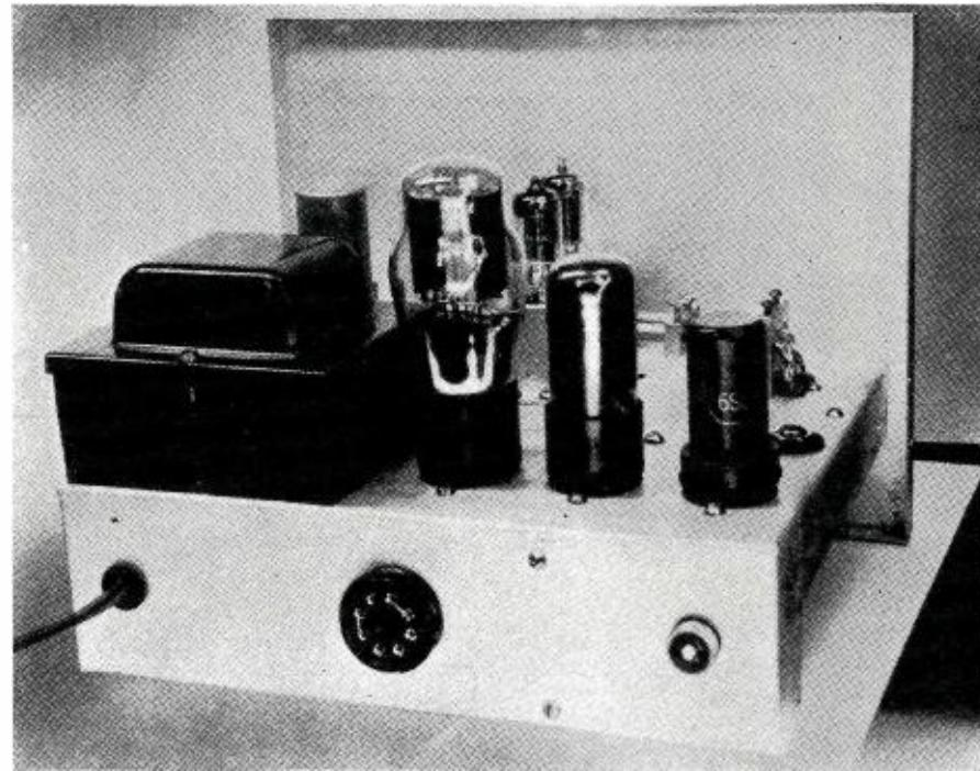
Fig. 3. Top-of-chassis view. Note the placement of the two 6C4 miniature tubes.
