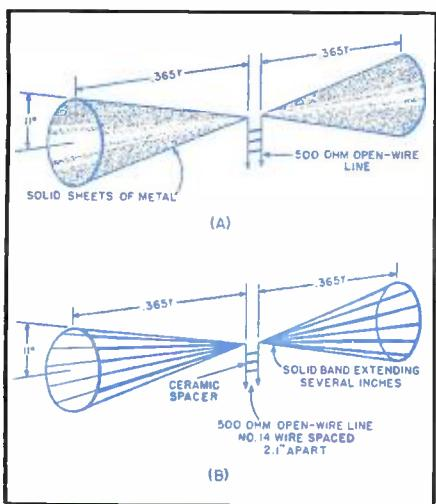
Fig. 5. Details of the conical antenna: (A) using solid sheet of metal and (B) employing twelve strands of equidistantly spaced No. 14 wire.
