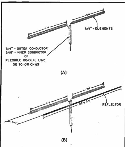
Fig. 10. Mechanical characteristics of a straight dipole antenna (A) and a dipole, including reflector (B).
