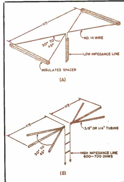
Fig. 3. Two popular types of antennas: (A) V antenna; and (B) fanned antenna.
