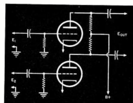
Fig. 2. Circuit for performing subtraction. A necessary requirement is that the two separate inputs be in phase. Circuits of Fig. 1 could similarly be used by employing a  $180^\circ$  phase shift between  $E_1$  and  $E_2$ .
