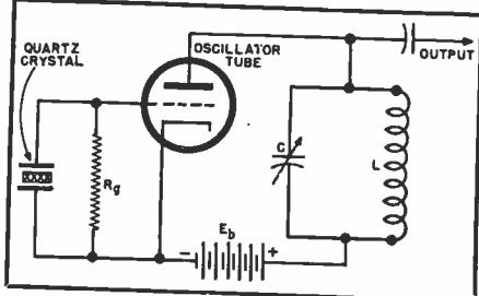
Fig. 9. A fixed-frequency quartz-crystal-controlled oscillator.
