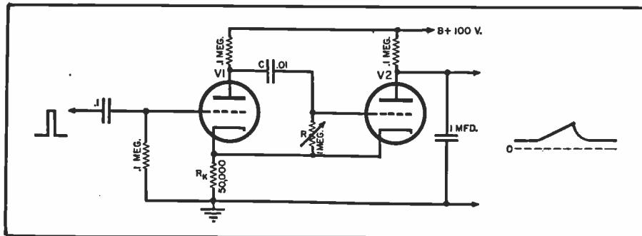
Fig. 12. Wiring diagram of a vacuum-tube single-sweep circuit.
