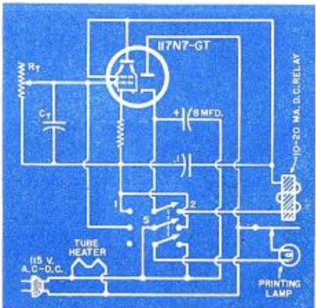
Fig. 5. Diagram of a phototimer.
