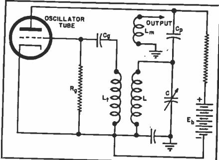
Fig. 7. A plate-tuned oscillator circuit that makes it possible to employ a tuning capacitor (C) having a grounded rotor.
