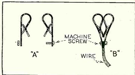
stripped two fahnestock clips from a discarded "B" battery, pressed the "faces" or spring sides together, as shown at "B" and held them in position by means of the machine screw.
