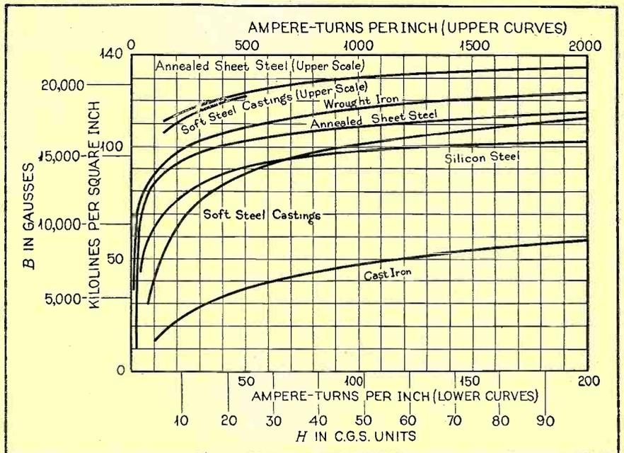
Fig. 2. “B-H” curves showing the relation between the magnetizing force H and the corresponding flux density B produced in various kinds of iron and steel. Fig. 3. Curves showing how the permeability of iron and steel varies when the magnetic flux density is varied
