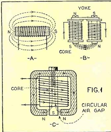
Fig. 1. Three different forms of electromagnets: (A) A straight bar electromagnet. (B) A form of horseshoe electromagnet. (C) An iron-clad electromagnet (coil completely enclosed by iron)
