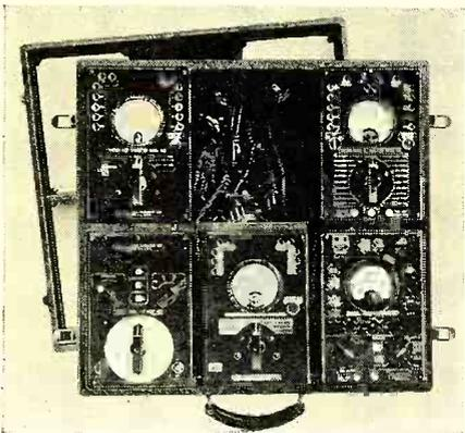
all makes of receivers. The tube checker, model 661, tests 4, 5, 6 and both the large and small-size 7-prong type tubes. It operates from 100 to 130 volts, 60-cycle a.c. line supply. The i.f. and r.f. test oscillator, model 662, is a self-modulated instrument with frequency ranges from 100 to 3000 kilocycles. The No. 663 volt-ohmmeter will indicate readings below 10 ohms to as low
