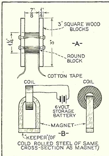
on either leg, not necessarily in the bow, as shown at (b), then bridge the piece of steel across the open end of the magnet. The purpose of this is to complete the path for the charging flux. Finally connect the two ends of the coil winding to the terminals of a 6-volt storage battery. The
