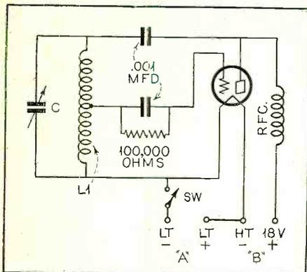
to the frequency range to be covered. The audio pitch can be varied by substituting different values for the grid leak. Higher values will provide a lower note, while lower resistor values will raise the pitch.
