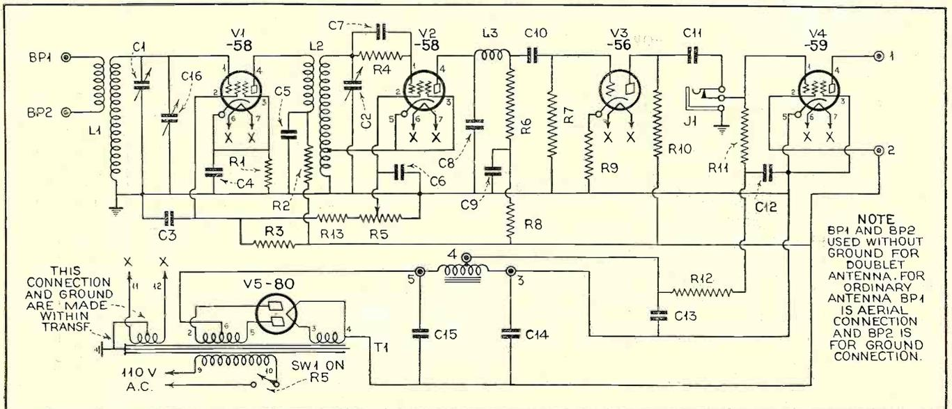
and V2 are put into place at the same time. The dual variable tuning condenser C1, C2 is equipped with stay bolts, so that the bolts can be slipped into the holes provided for them in the chassis and fastened securely. The condenser is mounted and then the dial. A single bolt on the front chassis wall holds the dial in place.
