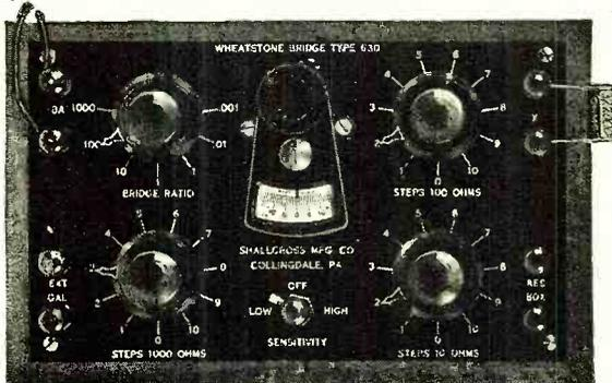
This inexpensive, rugged, and reliable instrument can be easily assembled by electrical technicians. Good accuracy is attained by employing a set of very accurate SHALLCROSS Resistors and a sensitive L & N Galvanometer.
