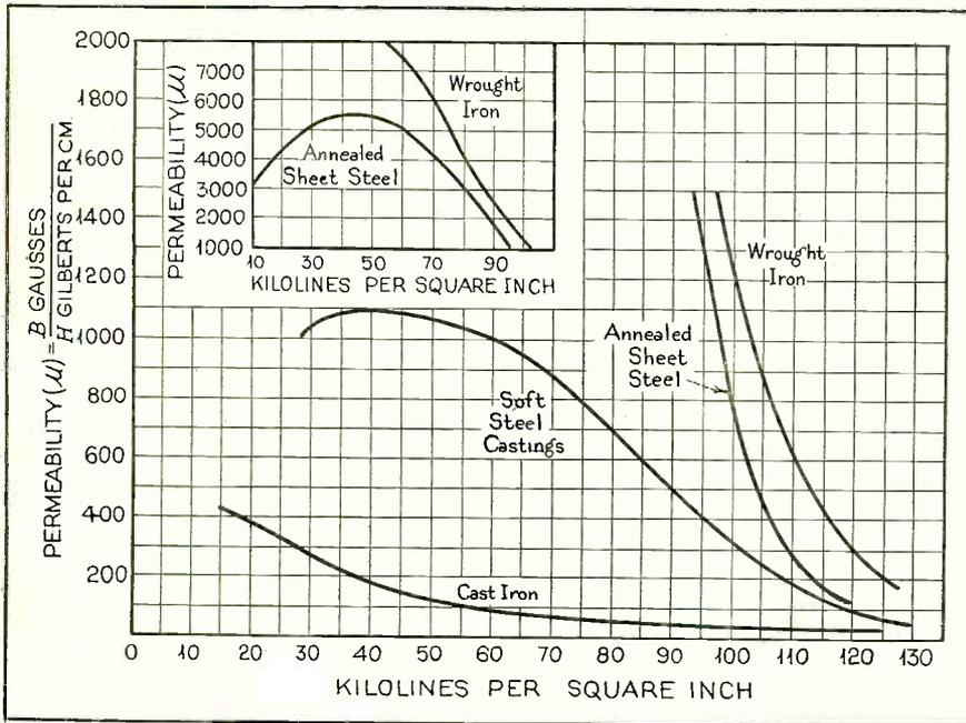
Figure 3. Curves showing how the permeability of iron and steel varies when the magnetic flux density is varied
