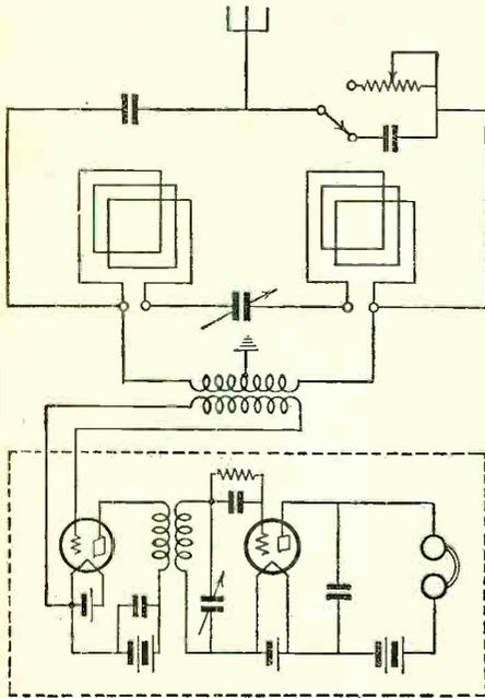
directional antenna and said non-directional antenna, and a coupling device associated with the circuits of said antennæ for transferring energy therefrom.
