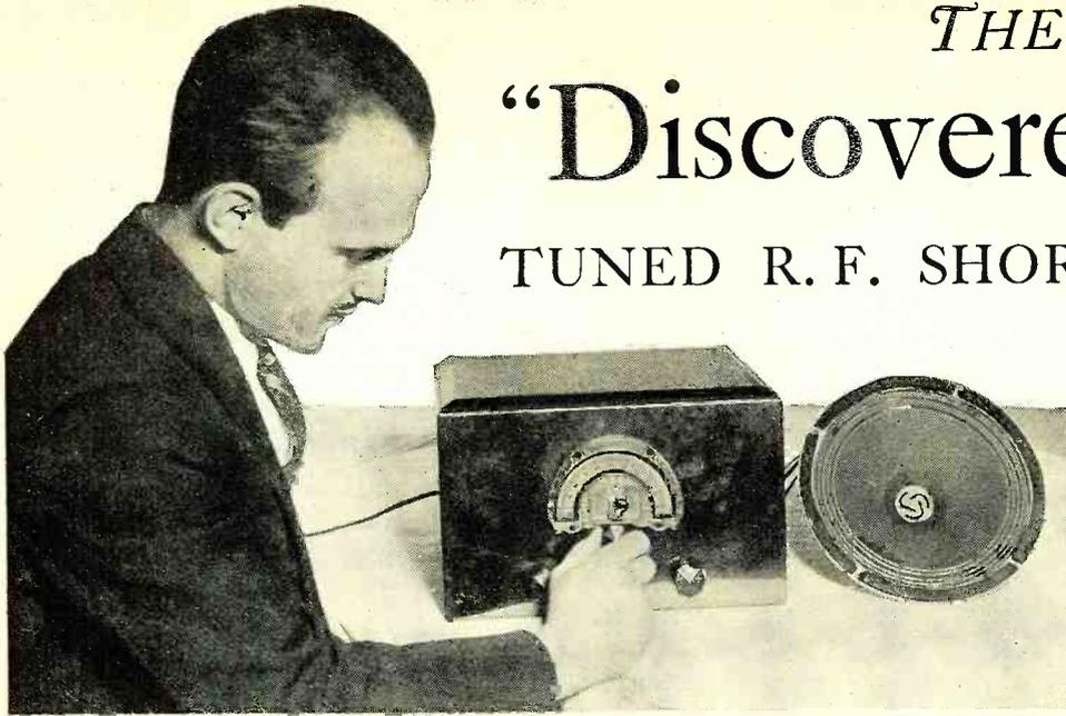
counting from the ground end. This type of regeneration gives smooth regenerative action, with full, even control. It also has a very important advantage that changing the position of the regeneration control does not detune the set. The variable resistor R5 controls regeneration by changing the detector screen-grid voltage.
