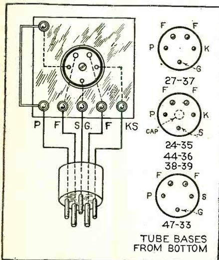
plainly marked. With all the terminals in a row on top, the filament, plate, or any of the grid voltages may be easily tested. An opening, which may be shorted, is left in
