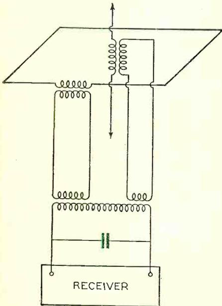
angles to each other, said antennæ being connected transmission lines with a joint radio-frequency circuit, one of said transmission lines being longer than the other by a length equivalent to one quarter of the communication wave whereby the oscillations of both antennæ are fed to said radio-frequency circuit with a 90° phase displacement.
