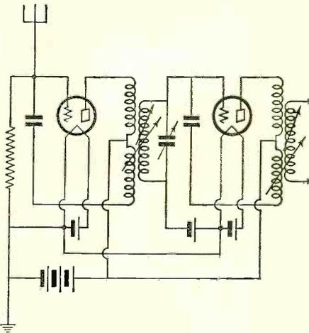
dary self-inductance, the mutual inductance and the ratio of secondary to mutual inductance of said transformer whereby the degree of amplification may be increased as the frequency to which the amplifier is tuned is decreased.
