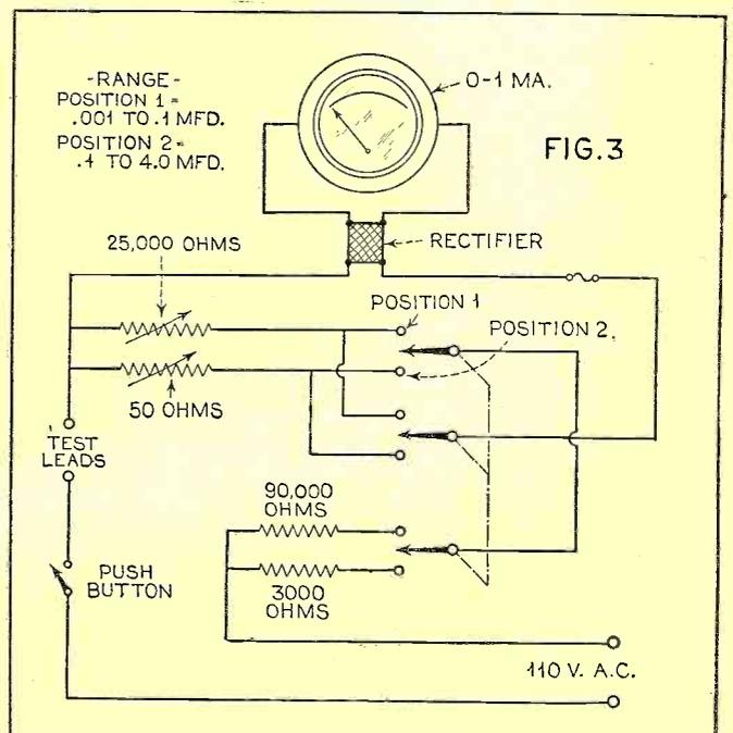
This type of a.c. meter indicates the average value instead of the r.m.s. value, and as a result, the range of the meter is a little larger than that of a d.c. meter with the same multiplier. The resistance of the rectifier varies slightly with the current flowing through it. (This is true of every rectifier-type a.c. meter.) For this reason, the scale is necessarily non-uniform.
