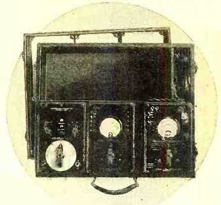
OSCILLATOR—VOLT-OHMMETER—CAPACITY METER in this compact kit
