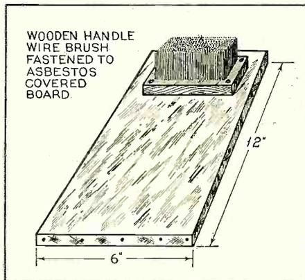
tured around when it is most needed. The broad asbestos surface of this support is hard to miss; and there is no danger of the hot iron burning through the layer of asbestos. The bristles of the wire brush are excellent for cleaning off the tip of the soldering iron. A wipe of the iron on the brush each time it is used will remove the corrosion and keep the point clean and shiny.
