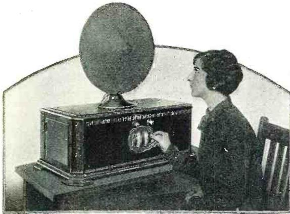
At the left is a view of the AC-operated Ultradyné, mounted in an attractive walnut cabinet. The drum dial is the wavelength control, the knob at the left the volume control, and the other a sensitivity adjustment.
