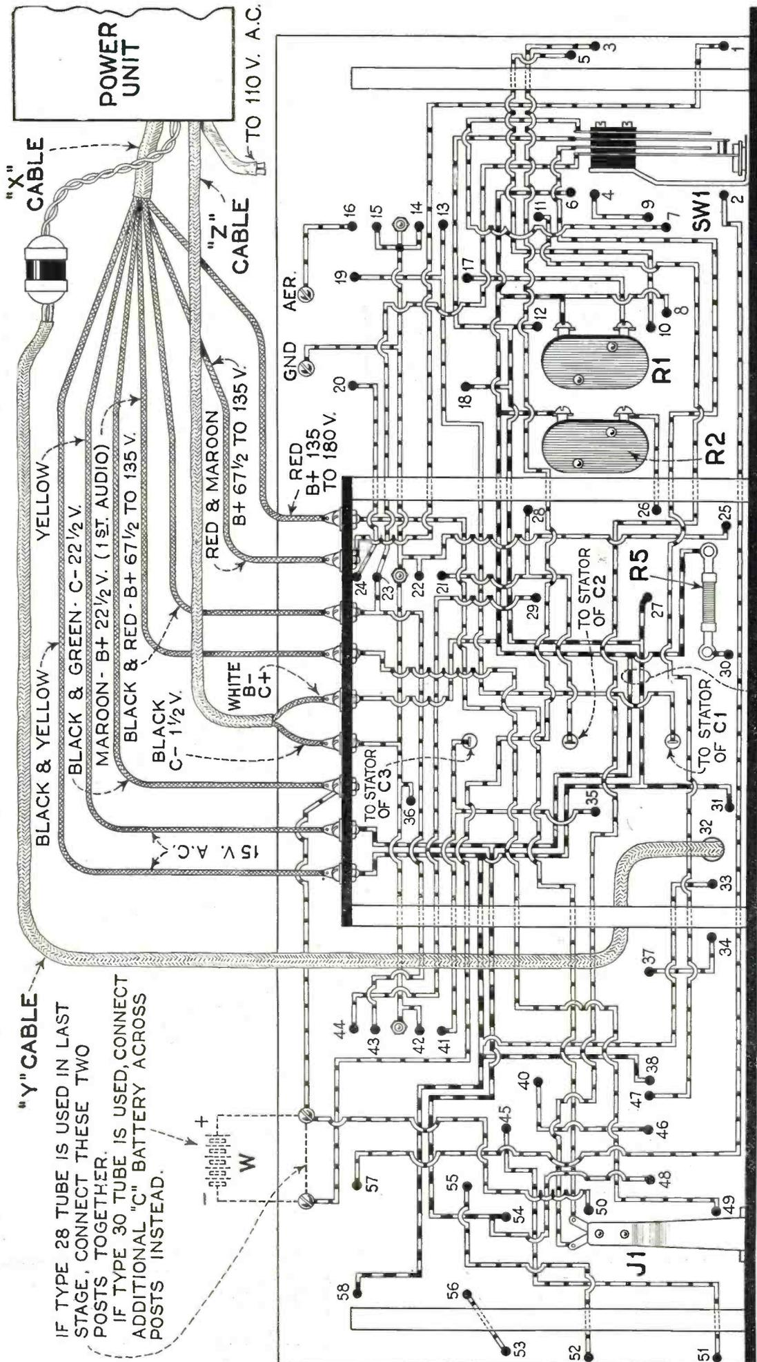
IF TYPE 28 TUBE IS USED IN LAST STAGE, CONNECT THESE TWO POSTS TOGETHER.
