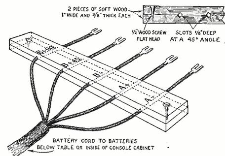
Complete details for building an inexpensive battery-cable separator are given in the above drawing.
