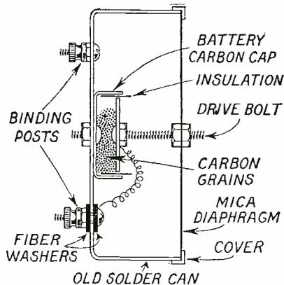
Fig. 1: Method of mounting the battery cap on the back of the can.
