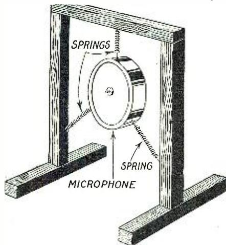
Fig. 2: By suspending the microphone from springs, as shown, results can be greatly improved.
