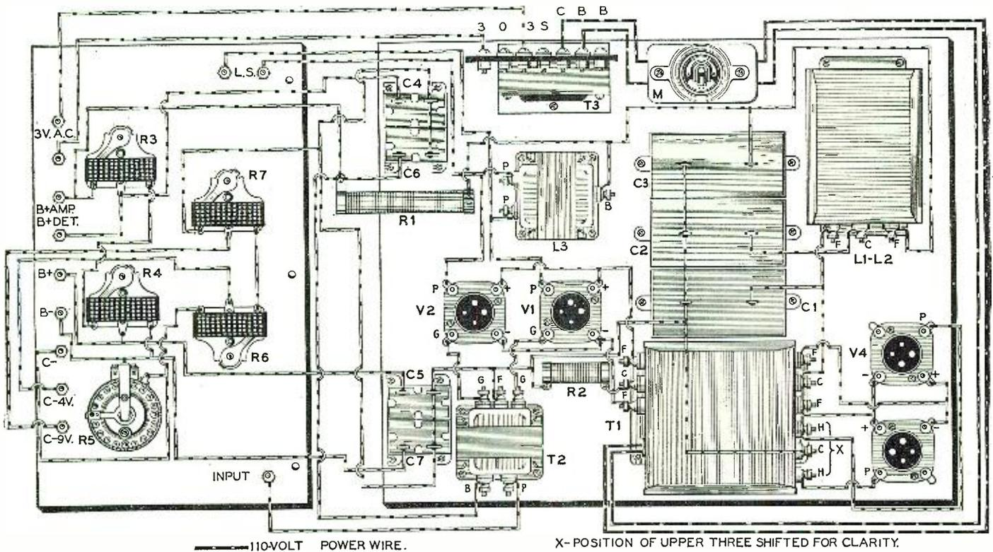
This diagram shows in pictorial form all necessary connections in the "A, B and C" power unit. The front panel has been tipped forward to show the connections to the resistors more clearly.
