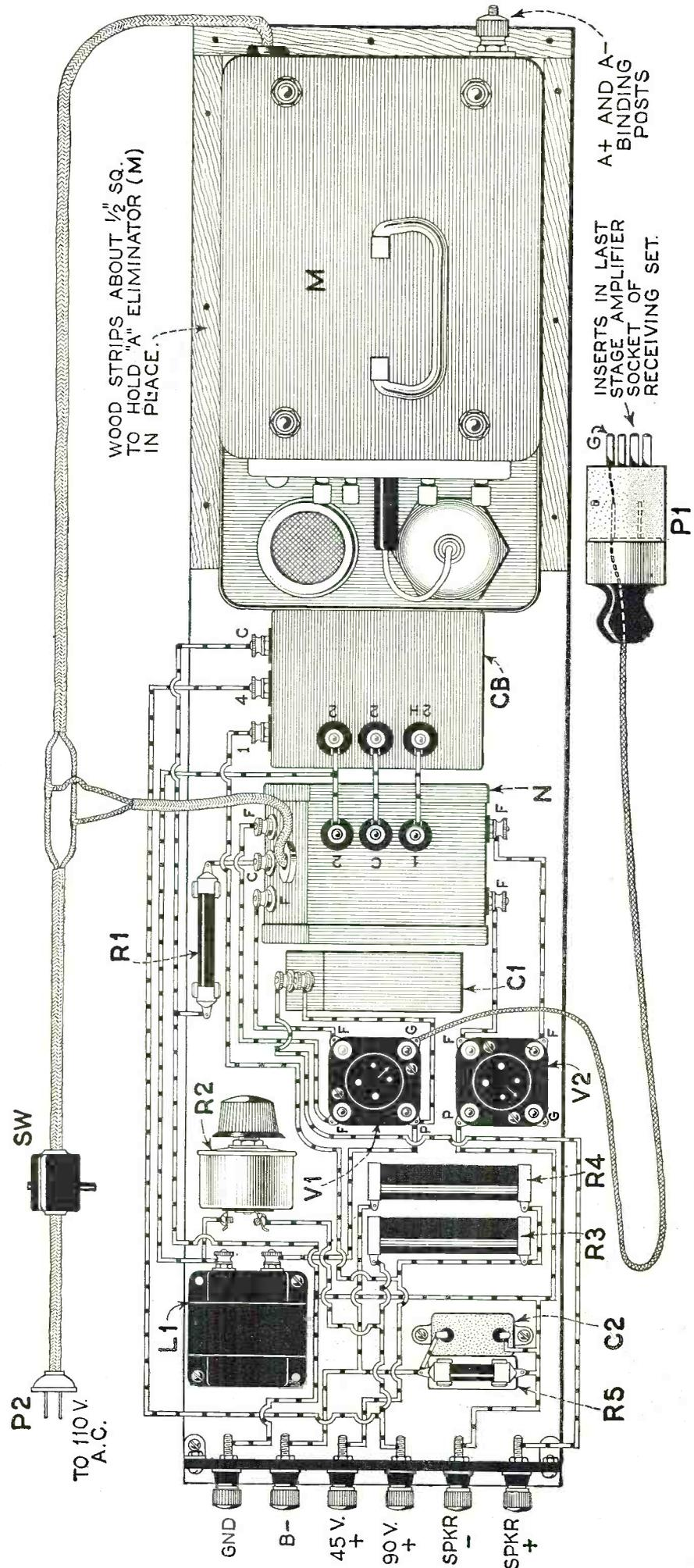
The wiring diagram of the "A, B and C" power unit and power amplifier. The schematic diagram, location diagram and list of parts will be found on pages 954 and 955.
