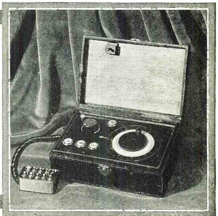
The remote-control box, attached to which is the plug which fits into outlets located in different parts of the house. By means of this the receiver may be tuned to different wavelengths.
