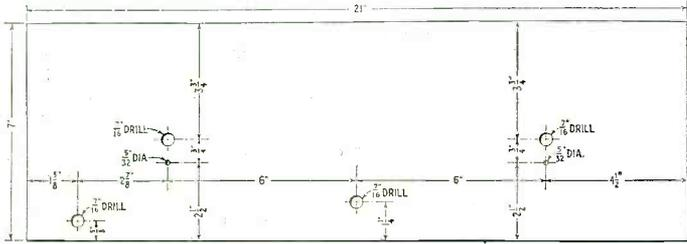
This drilling layout for the front panel of the Silver Shielded-Grid Six shows the position of the various holes required for mounting the tuning controls and securing the panel to the chassis.
