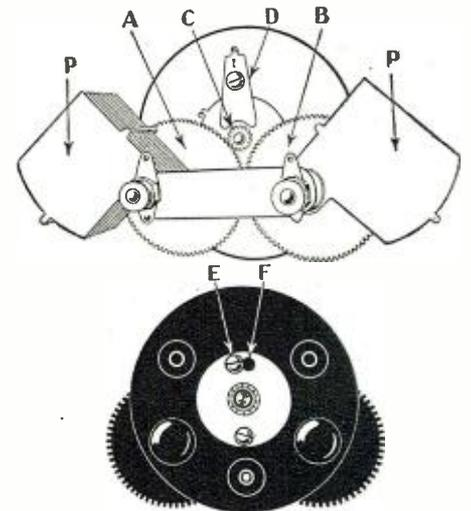
*New twin rotor condenser, which may be adjusted for either a clockwise or a counter-clockwise reading. Illustration courtesy Gray and Danielson Mfg. Co.*
