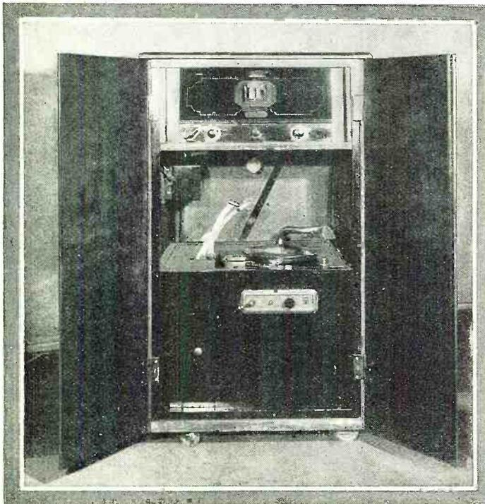
In the upper portion of the chassis is the radio receiver, beneath which is seen the automatic talking machine. In the case under the turn-table is the powerful amplifier.
