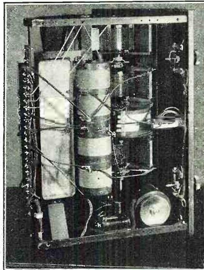
The rear view of the radio receiver, showing in the lower right corner the motor for driving the condensers.
