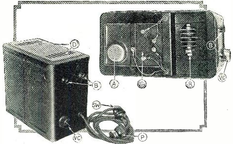
Two views of a new power unit which delivers 3 amperes at a potential of 6 volts. This device uses a dry electrolytic rectifier R, and an electrolytic condenser (C), and a heavy-duty choke as a filter.
