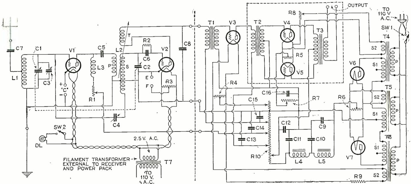
The complete schematic wiring diagram of the new two-tube Browning Drake receiver is shown at the left of the dotted line in the above illustration. The apparatus and wiring on the right of the dotted line is a power amplifier and plate-supply unit. Illustrations courtesy Browning-Drake Corporation
