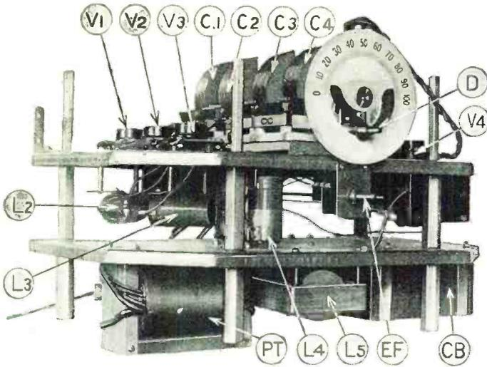
Modern two-deck construction is clearly illustrated in this general view of the receiver chassis removed from the cabinet.
