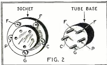
Diagram shows arrangement of terminals on a standard UY socket and tube base of the type used for a battery-cable plug.
