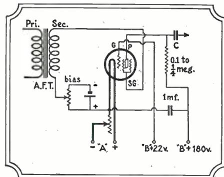
Fig. 9: In an A.F. circuit the normal control grid G is used as a space-charge element; the screen-grid (SG) now acting as the control-grid.
