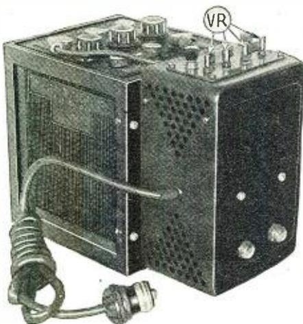
External appearance of the "A" power unit: the four posts marked VR are for regulating the rate of charge which the battery receives.
