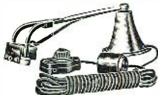
molded in the bakelite housing, a coil and a soft-iron armature with an aluminum attachment to carry a phonograph needle. This attachment is held in its position by two small soft rubber plates. The soft-iron armature moves freely, without touching the center of the coil; its lower end extends into the air gap between the two pole-pieces.
