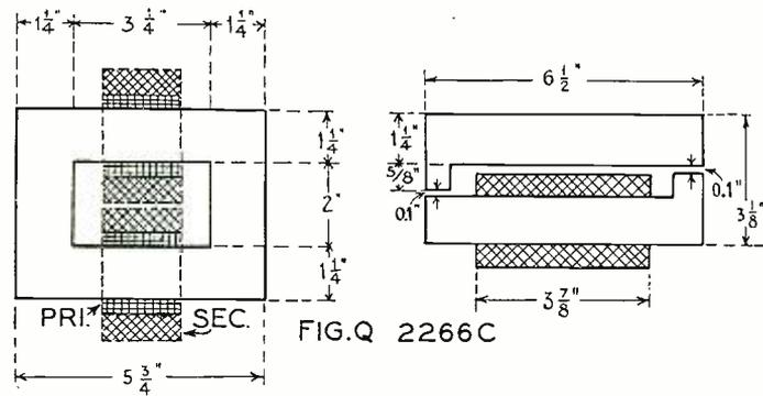
The specifications of the cores for the transformer and choke coils are shown here. It will be noticed that two air-gaps of 0.1 inch are left in the opposite sides of the choke coil, in order to reduce eddy currents, which would reduce the inductance, and consequently the efficiency of the choking action.
