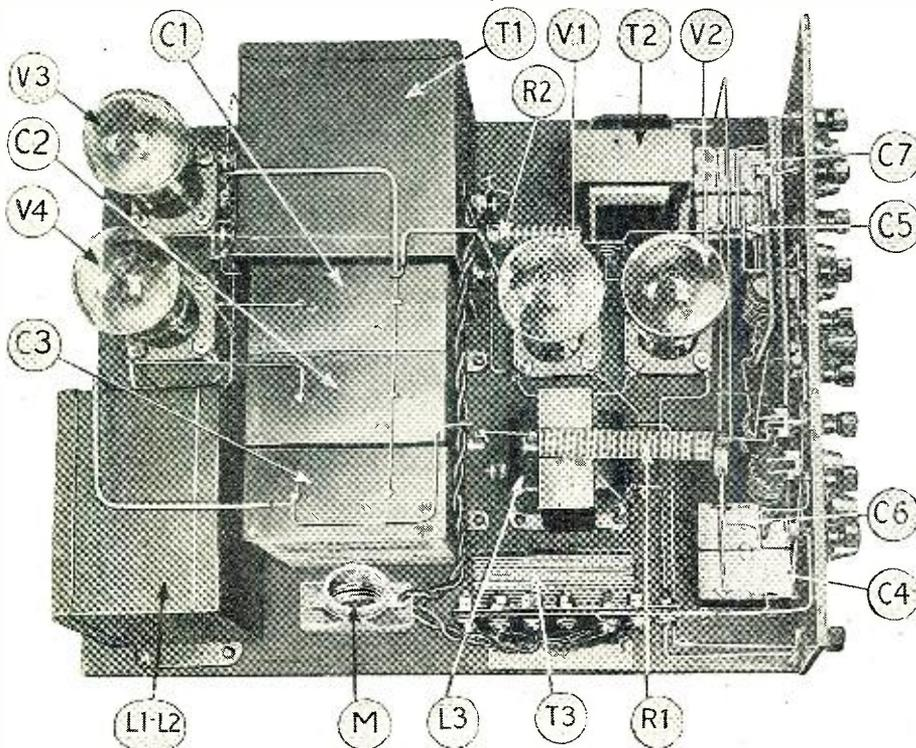
*Another view of the power unit designed especially for the operation of the Electric Nine receiver. When operating the power unit the 110-volt receptacle (M) is connected by a cord to a lamp socket, at which the set is turned on and off.*
