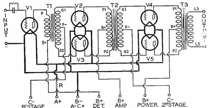
The unit illustrated on the left is a new-type push-pull transformer with center-tapped primary and secondary windings. It makes possible the use of the amplifier circuit shown. Illustrations courtesy Samson Electric Company
