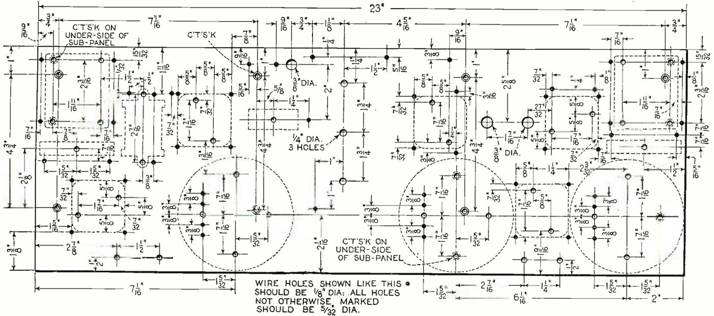
Drilling layout for the sub-panel of the Electrified Peridyne. The parts are indicated by the dotted outlines. The layout for the power unit and its case will be found on page 962.
