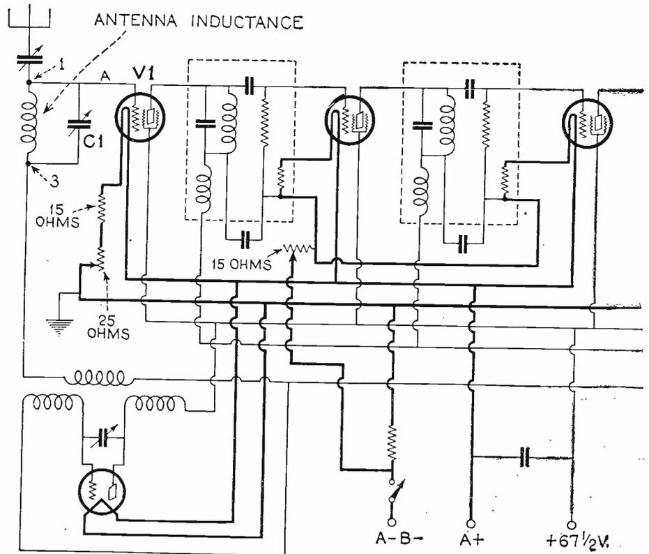
The schematic diagram of the first portion of the Tyrman Shielded-Grid Seven, using the 222-type tubes. This set, originally designed for loop operation, is shown here adapted to aerial operation.
