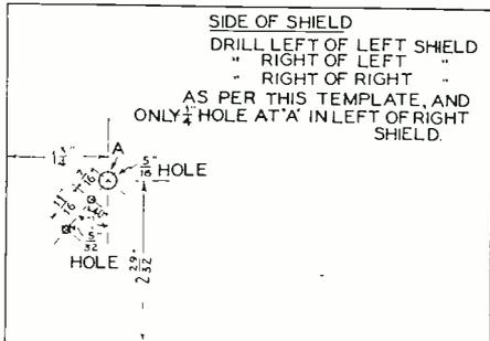
The above drawing shows the exact position for the condenser mounting holes in the shields.
