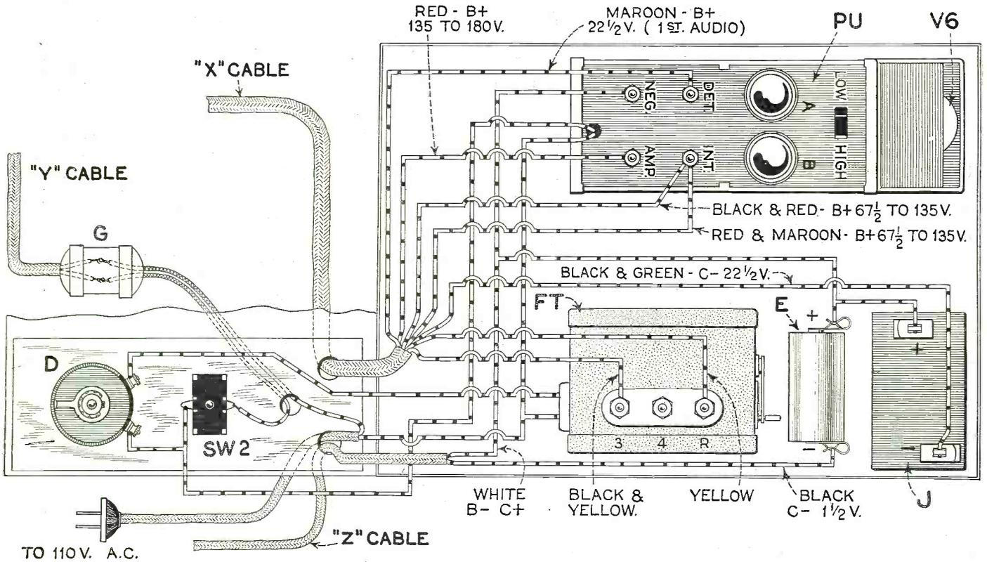
Wiring diagram of the power unit for operating the Electrified Peridyne. The schematic diagram of this unit will be found on page 962.
