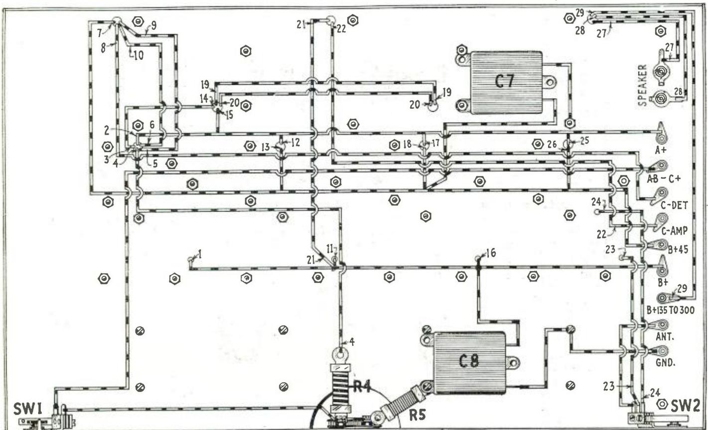
In this pictorial wiring diagram the wires under the chassis are clearly shown. Where one passes through a hole in the chassis, it is marked with a number by which it may be identified in the diagram on the opposite page. The two fixed-resistor strips shown at R4 and R5 are mounted directly on the binding post of the rheostat R6.
