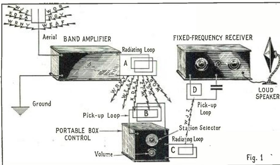
Signals from all stations within the receiver's range are amplified in the band amplifier, and the one to which it is desired to listen is tuned in by the station selector and transmitted on a new wavelength to the fixed-frequency receiver.
