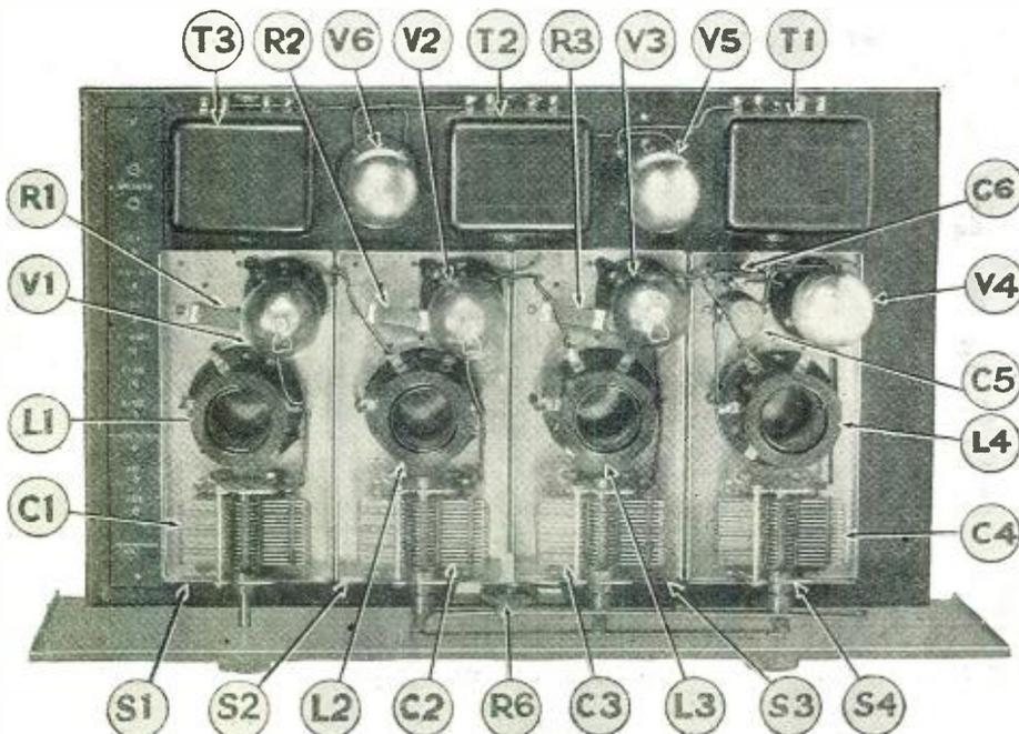
*This picture shows the appearance of the Shielded-Grid Six receiver with the shielding cans removed. The three shielded-grid tubes are shown at T1, T2 and T3; and the special R.F. transformers which have been designed for these tubes are indicated at L1, L2, L3 and L4. The new tubes are used in the three R.F. circuits. V4 is the detector tube, and V5 and V6 are the two audio tubes, semi-power and power.*
