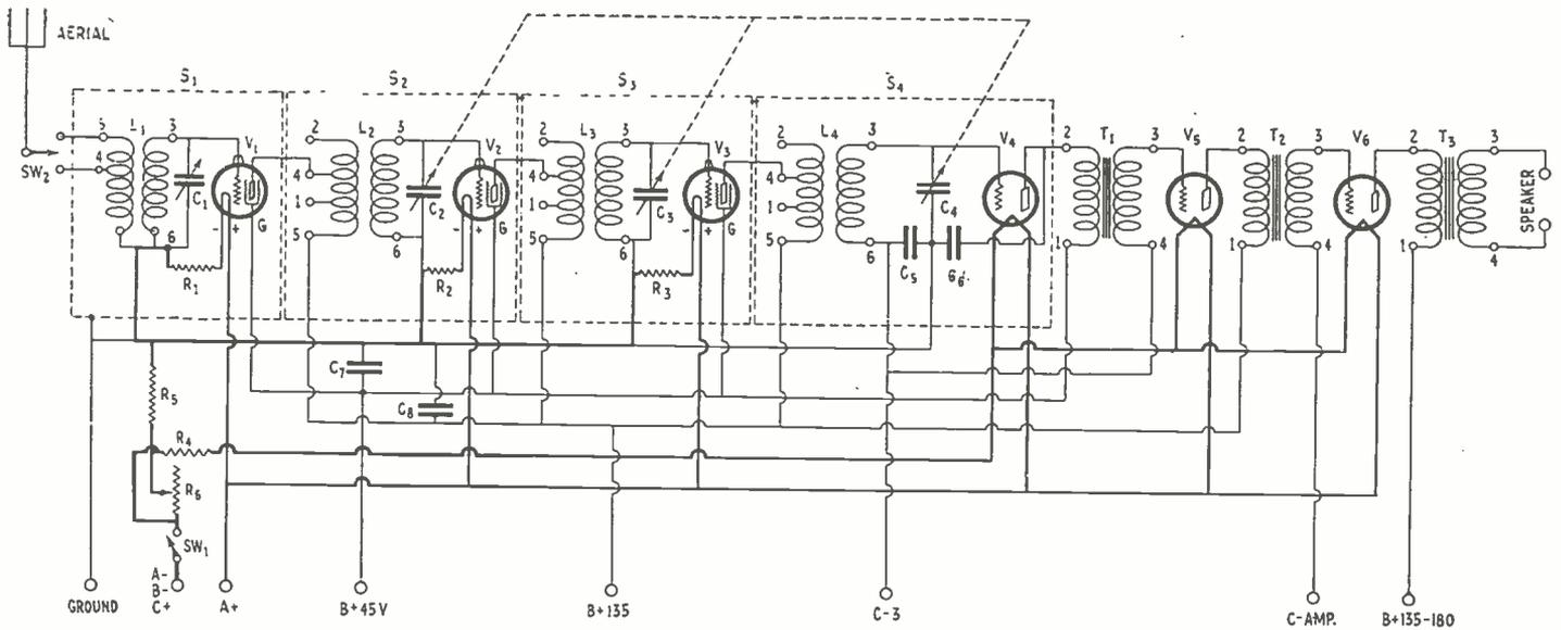
In this schematic wiring diagram of the Silver Shielded-Grid Six, dotted lines show the enclosure of parts and wiring within the stage shields, as well as the connection of the variable condensers by the link motion. In the detector circuit a biasing voltage is used on the grid to prevent overloading.
