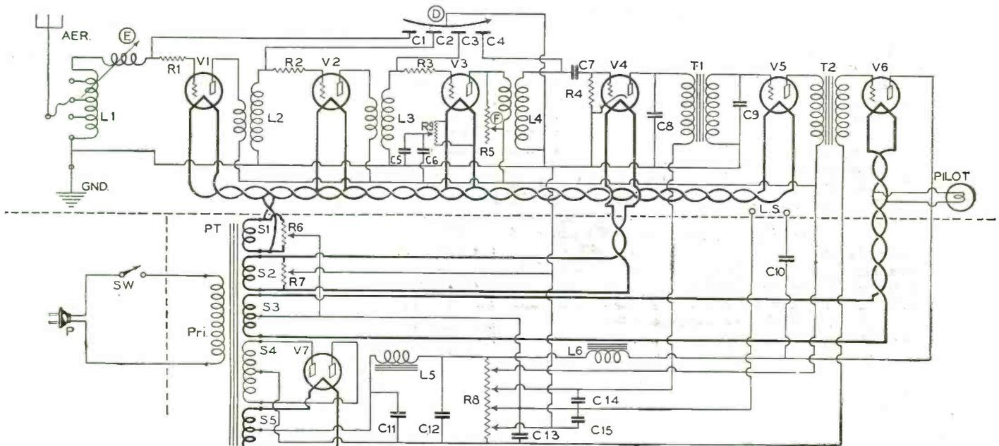
The complete circuit of the six-tube electrified receiver described on this page; parts and wiring shown below the line are in the power-supply circuit.
