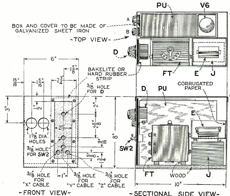
The constructional details of the power unit of the Electrified Peridyne, with all necessary drilling instructions and dimensions.
