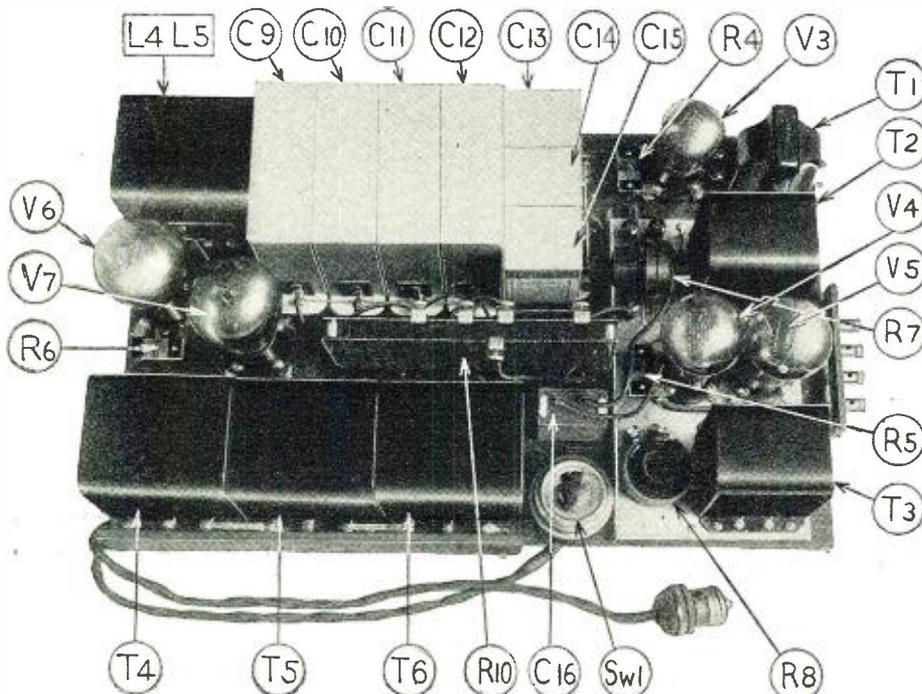
*General view of two-stage power amplifier and plate-supply unit. Illustration courtesy General Radio Co.*
