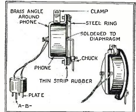
An electric phonograph pick-up unit may be made of an old sound box and a loud-speaker unit as shown.
