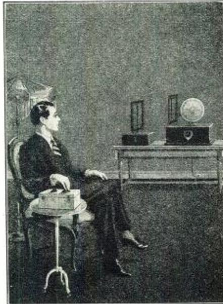
The loops in the station selector (on the small table) are concealed within the box; the left-hand cabinet on the table contains the band amplifier; and the fixed-frequency receiver is on the right.
