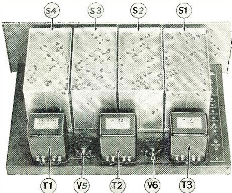
View of receiver with shielding compartments in place. S1, S2 and S3 are the first, second and third R.F. stages, respectively; S4, detector stage; T1 and T2, audio transformers; T3, output transformer; V5 and V6, audio-stage sockets.
