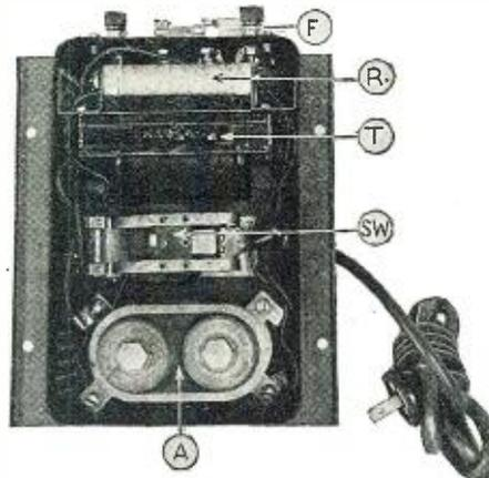
Arrangement of apparatus inside the power unit: A, rectifier unit; F, fuse; R, resistor; Sw, relay switch; T, transformer.
