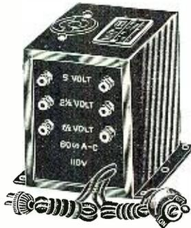
supplies the necessary low voltages for heating the filaments of all the tubes in radio receivers using raw A.C. It operates from the 110-volt 60-cycle house lighting line, and supplies 1½ volts, 2½ volts and 5 volts, the latter for power tubes of the UX-171 type. This transformer is enclosed in a black japanned sheet-iron shell, and is mechanically and electrically very well designed. It is provided with two cords, one 8 feet long with a plug to fit into the receptacle of
