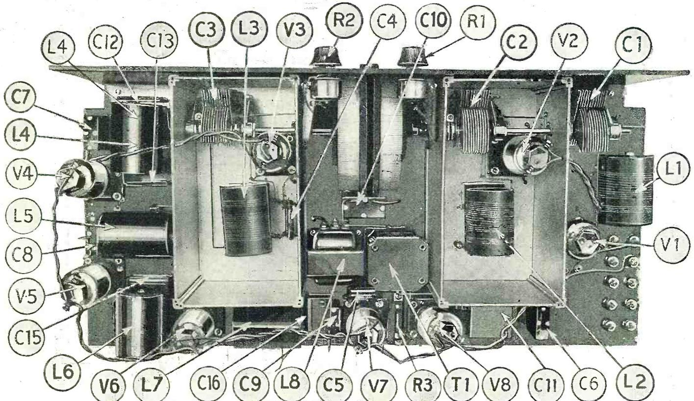
This view of the "All-Wave Electric 9" shows the exact location of all parts used in its construction. L1 and L2, R.F. transformers; L3, oscillator coupler; L4, L5, L6, and L7, intermediate-fre-
