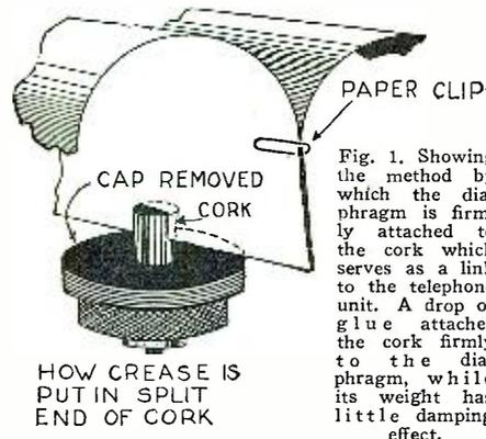
Fig. 1. Showing the method by which the diaphragm is firmly attached to the cork which serves as a link to the telephone unit. A drop of glue attaches the cork firmly to the diaphragm, while its weight has little damping effect.
