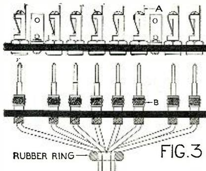
The strips supporting the plugs and jacks are here shown. By spacing unevenly the end plugs it is made impossible to insert them the wrong way.
