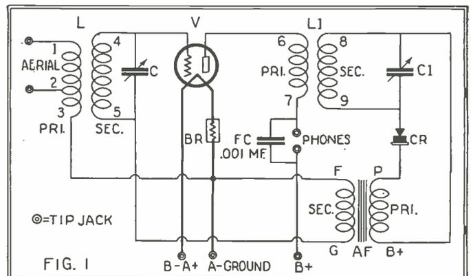
Above, in Fig. 1, is shown the schematic diagram of the one-tube reflex circuit used in this portable set.
