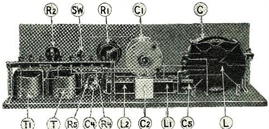
Back view of the receiver. The variable inductor L hides the variable condenser C, to whose end it is attached. R1 is the combination rheostat-potentiometer, R2 the rheostat which controls the current to the filament of the last tube. This illustration shows how the binding-post strip at the left is raised above the tops of the transformer T and the resistance-capacity-impedance unit T1.
