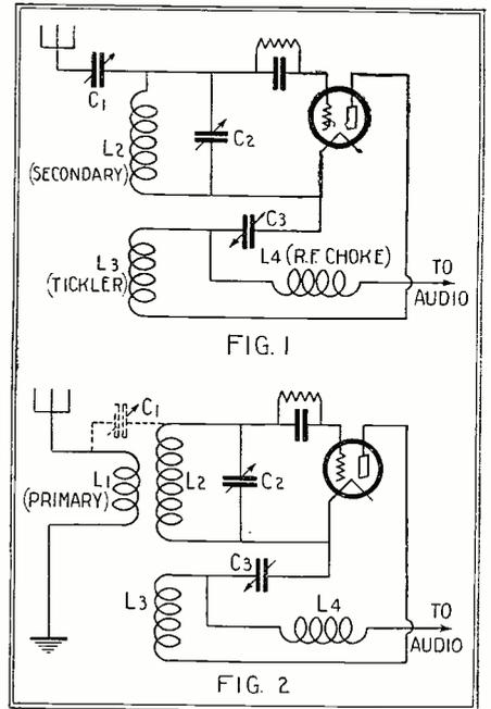
In Fig. 1 is shown the receiving circuit used for short waves, and in Fig. 2 that for wavelengths up to 1,500 meters.
