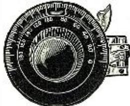
The "Precision" Condenser Vernier shown, is in its main features identical in construction to the plain-type condenser described above. It differs only in that it is equipped with a vernier arrangement of the friction type, having a ratio of 30:1, and that there is a pigtail connection between the rotor and end plates. Both condensers are of the one-hole mounting type.
