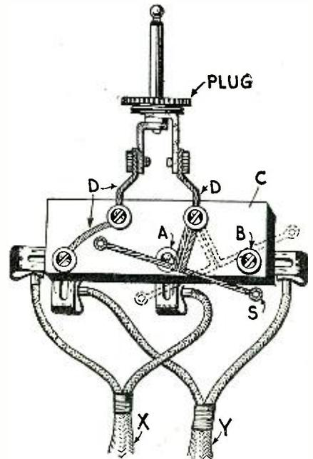
By throwing the bus-bar switch, S, from A to B (switchpoints) a second speaker can be heard almost instantaneously. C, insulating panel; D, bus-bar; and X and Y, speaker connections.
