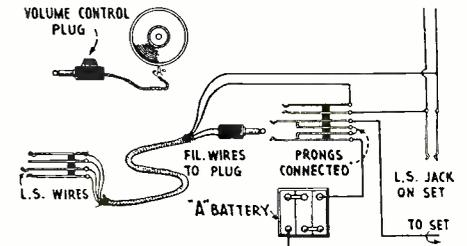
How the filament circuit can be controlled from a distant point.
