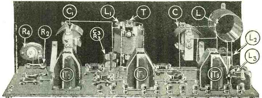
(Q. 2201). A top view of the Samson Dual T.C. receiver. A power tube is employed in the last audio stage to enhance the quality of reproduction obtained. A 500,000-ohm variable resistance to obtain volume control is also incorporated, and is indicated as R-4 in this view.
