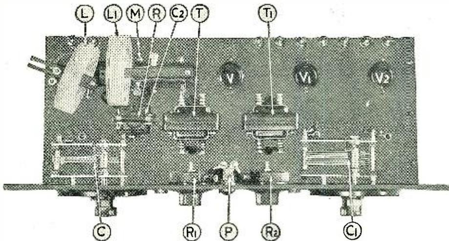
Looking down on the sub-panel. C is the tuning condenser; M, the coil mounting; V, V1, and V2 are the detector and two A.F. tubes; C2 and R, grid condenser and leak respectively.
