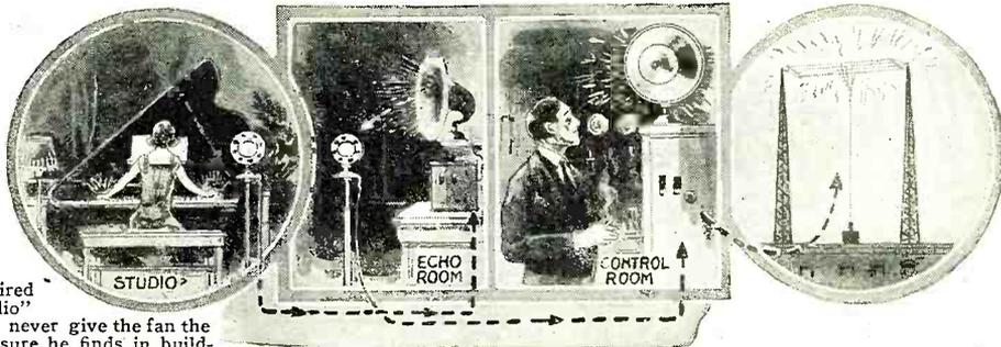
Station 2LO, London, has an "echo room," which is bare of the usual heavy studio drapery. Here a loud speaker reproduces the program, and a microphone collects the reverberations and adds them to the modulation of the music. This effect is never used with the voice of a speaker.
