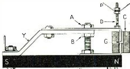
Side view of the loud-speaker unit, showing the details of driving mechanism.
