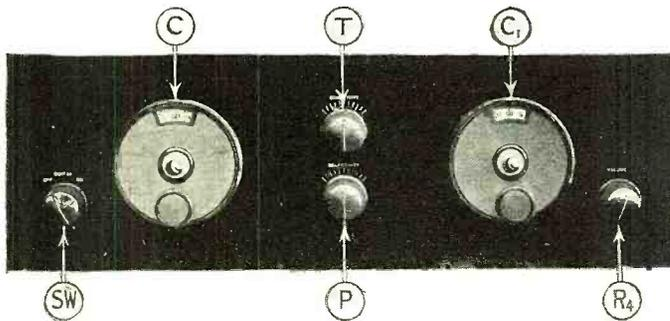
The panel view of the Dual T.C. receiver shows a neat and symmetrical appearance. The knob T controls the tickler, shown above; the knob P the primary, which is similarly wound on a rotatable form and may be varied in its relationship to the secondary. This primary knob on this receiver is marked "selectivity."
