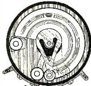
Back view of the resistor-switch, showing the arrangement of the flexible spring plunger, rotating arm and contact points.
