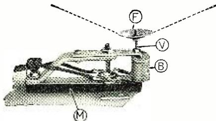
General view of the loud-speaker unit. M is the permanent magnet, B the bobbin, V the vibrating armature and driving screw, F the small metal cone for holding the large paper cone in place. The position of the paper cone is indicated by the dotted lines.
