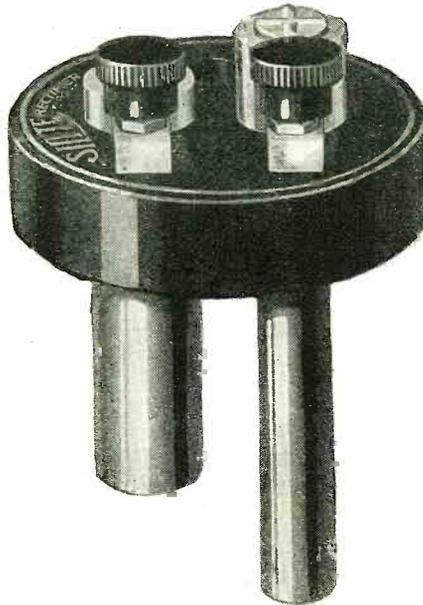
This is the assembled cap and electrodes, that on the left being lead and the longer one, silite. These caps are used with jars, in which common battery electrolyte is placed, and serve as rectifiers in various types of chargers.
