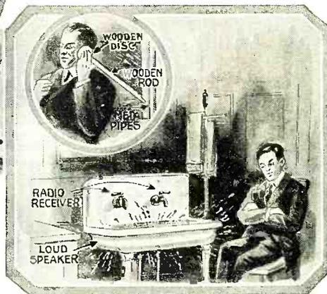
Toronto, Ont., radio men are puzzling over a common metal sink which has taken upon itself the duties of a loud speaker, according to press reports. The programs broadcast from CFCA, in the same building, without apparent electrical or mechanical connection, are reproduced with moderate volume. The sound appears to be carried by the water pipes, in some unknown way.
