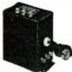
The complete power amplifier foundation unit. Contains (1) a power supply transformer, (2) a center tapped filament supply for the power tube, (3) two 30 henry filter chokes, (4) two buffer condensers of 0.1 Mfd. each.—all in one com-
