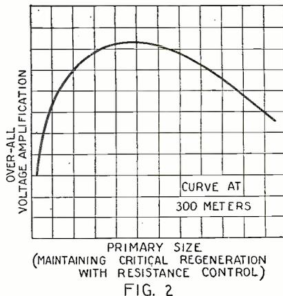
A curve showing the variation in over-all amplification with the number of primary turns at critical regeneration.
