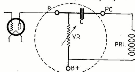
This diagram shows how the phase-shifting instrument, consisting of the fixed condenser, C, and the variable resistance, VR, is connected in the plate circuit of an R.F. amplifier stage. The posts marked P, PC, and B+ represent its three external connections.
