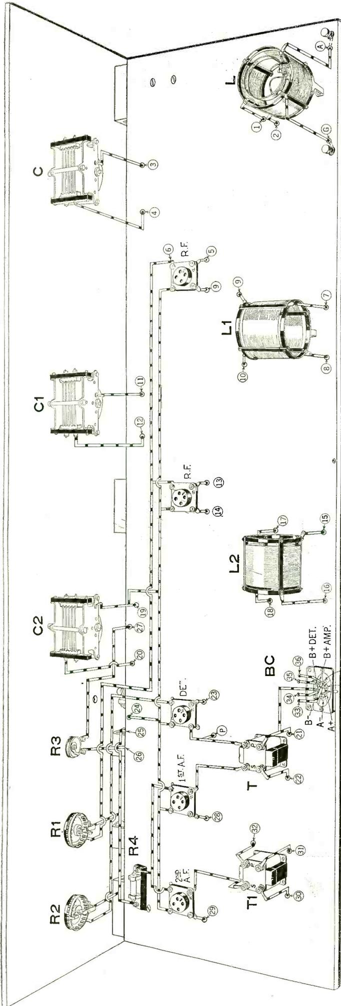
A perspective layout and wiring diagram of the Aero-Dyne receiver. The only portion of the wiring that might present some difficulty is that in the vicinity of the variable resistance, R3, where the leads pass down between the panel and the sub-base. However, if the lower drawing is consulted, the wires can be traced through the numbers in circles which are identical, for each lead, above and below the sub-base.
