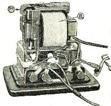
The charger with the case removed. The bobbin, B, holds the transformer windings. PR is the polarized relay. The primary circuit relay is hidden beneath the bobbin and is not visible in this view.
