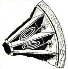
Two English loud speakers. That at the left is a cone-type with amplifier, complete in the cabinet. Above is the "Donotone" cone speaker, which has radial baffles and springs, as shown in the lower sketch.
