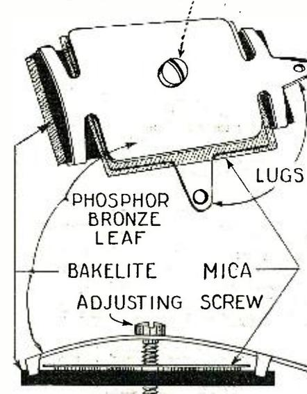
These perspective and side views of the midget condenser show its simple construction plainly.
