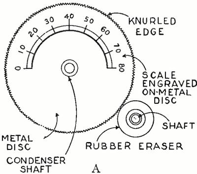
Details of the vernier knob and dial. A rubber eraser is used as the friction contact.
