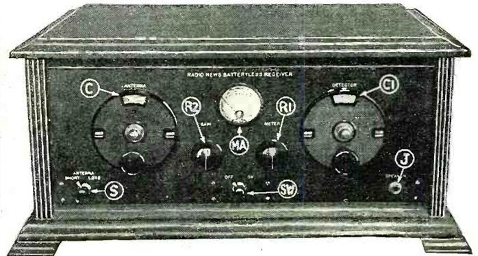
THE RADIO NEWS Batteryless Receiver consists of two units, the first being the receiver proper and the second its power-supply unit, designed to furnish power for the operation of the receiver directly from a 110-volt, 60-cycle lighting circuit.
