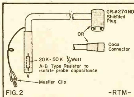
Hum-reducing leads for oscilloscope probes.
