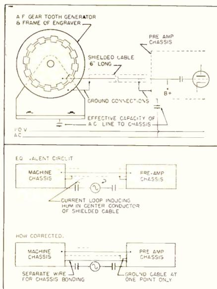
Partial block diagrams illustrating the hum problems encountered in service of the electronic photo-engraver. A ground loop was found to cause hum, which ruined the engravings.
