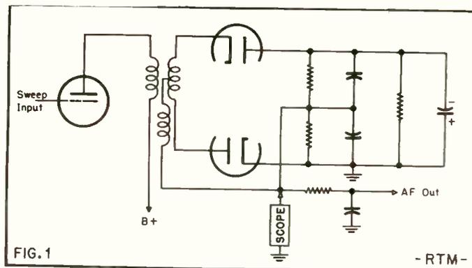
Basic ratio detector circuit. Note symmetrical networks across the diodes, large capacitor (shown polarized) across the networks, scope connections.
