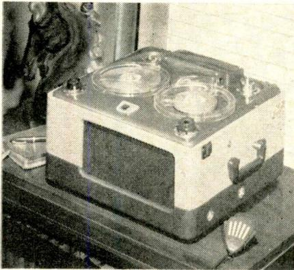
forward and reverse positions, the tape mechanism will record up to two hours on one reel, without turning the reel over, the company reports.
