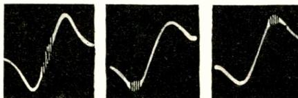
Response curve of ratio detector, as obtained from hookup shown in Fig. 1. Marker signal is shown at center frequency, or IF value, in first picture, and at the two limits of the band pass of the detector in the second and third pictures. (Courtesy John F. Rider, Publisher)
