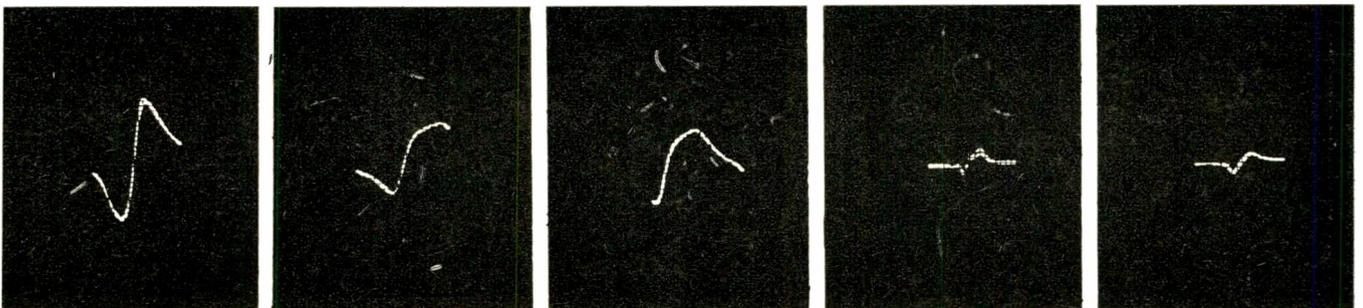
From left: 1. Normal "S" curve of properly adjusted discriminator. 2. Pattern of detuned discriminator primary. 3. Result of detuned discriminator secondary or bad oscillator tracking. 4. Reverse limiting,
