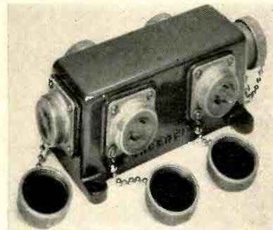
Input to the unit handles 6000 watts, while the five outputs will each handle 1500 watts. Sockets fit standard two-prong 110 v. plugs.
