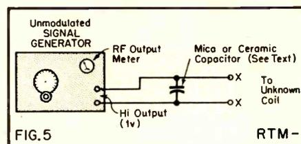
generator output circuit, effectively is in parallel with the tuned circuit under test and will influence the resonant frequency of the latter. Therefore, the measured frequency will be somewhat lower than the true resonant frequency unless care is taken to keep all stray capacitance low with respect to the circuit capacitance.
