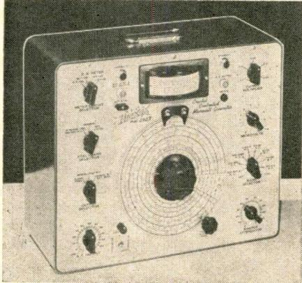
The signal may also be externally modulated from 15 to 10,000 cps, the maker states, with audio output variable from zero to two volts at 400 cycles. A Db meter indicates reference level.
