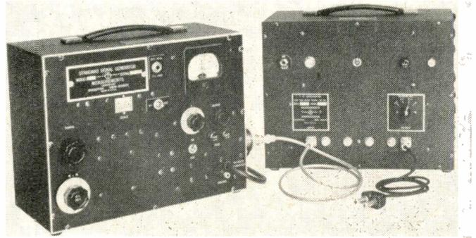
Measurements Corp. FM signal generator, covering 88-108 Mc band, and IF converter, which produces 4.5 Mc, 10.7 Mc, and 21.7 Mc signals.
