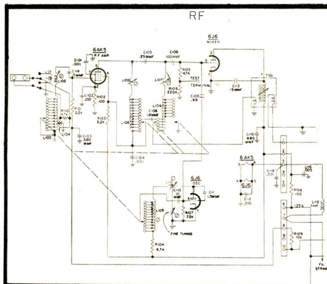
RF section of the Westinghouse V-2158-1A chassis—a typical inter-carrier system receiver.
