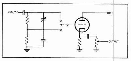
Fig. 2 Input circuit using cathode follower. This circuit minimizes frequency discrimination with changes in input signal attenuation, uses two-position cuenuator
