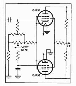
Fig. 5 Schematic of push-pull deflection amplifier. This circuit is a combination of phase inverter and amplifier
