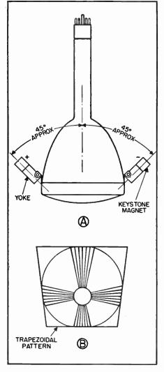
Fig. I (A) Projection tube of the Philco system, with magnets, (B) Keystone pattern
