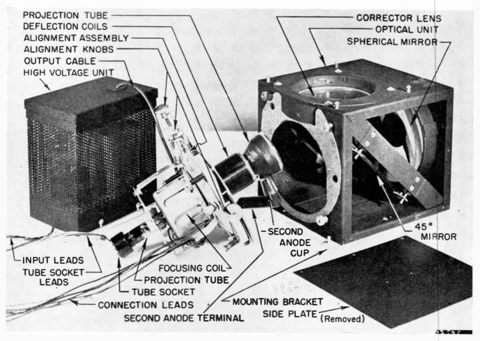
Fig. 2 Components of Protelgram television system. At the left is the 25 kv power unit, in the center the projection tube assembly
