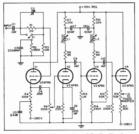
Fig. 3 Vertical deflection amplifier as used in the DuMont Type 208 oscillograph. Peaking coils are employed in plate circuits to extend the upper frequency response limits
