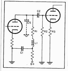
Fig. 4 Resistance-coupled amplifier; Cs represents interelectrode capacitance, and capacitance between leads and components
