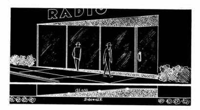
Fig. I Beveling the glass at an angle in plan reduces reflections and makes for a much-more attractive window. It's becoming increasingly popular
