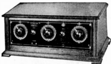
Trade Name—"Torodyne"; Type—Tuned Radio Frequency; Tubes—5; Battery—"A" Storage; "B" 90 Volts dry (Contained in Cabinet or the New A. C. Tubes); Controls—Tuning, 3; Tube, 2; Dim.—28½ x 12½ x 9½; Wt.—20 lbs.; Price—$100.00.
