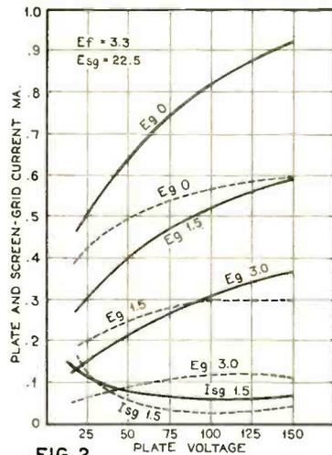
FIG. 2 Plate and screen-grid current, at 22½ volts.
