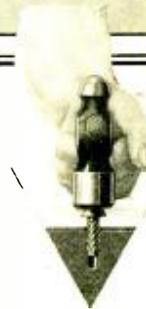
**A** HAMMER and some Hardened Metallic Drive Screws are all you need to make permanent fastenings to iron, brass and aluminum castings, steel, Bakelite, etc. No taps or tapping machinery necessary. A Hardened Metallic Drive Screw is its own tap—cuts a thread as you hammer it into a drilled hole.
