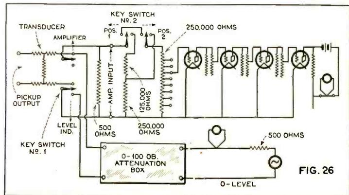
Illustrating function of key switch in relation to resistance network.
