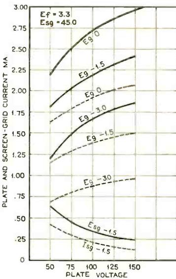
FIG. 3 Plate and screen-grid current at 45 volts.
