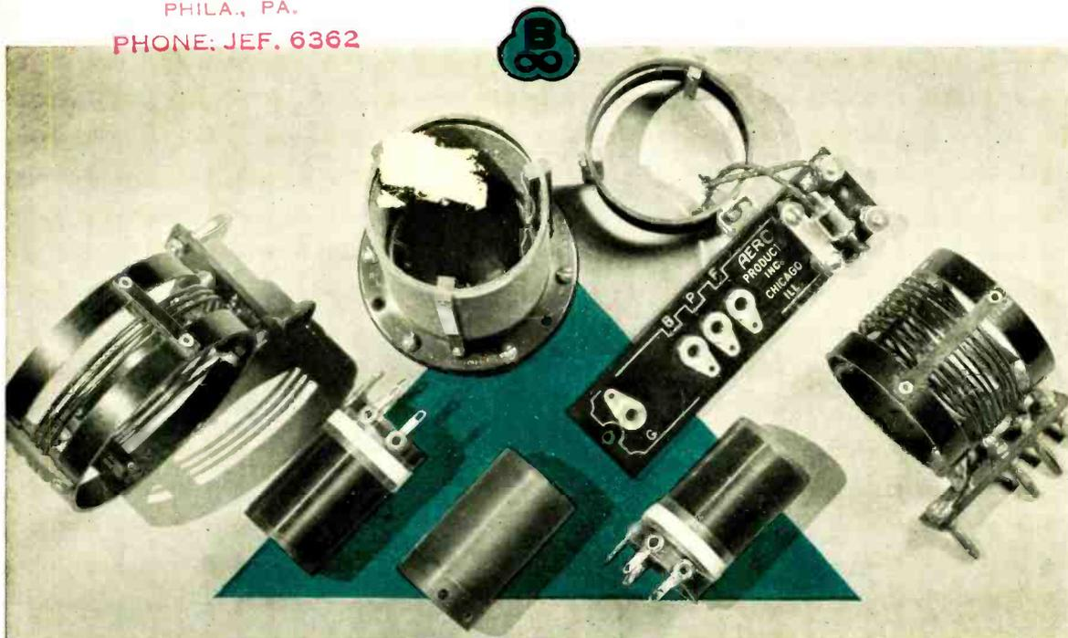
Radio Frequency Coils and threaded coil form of Bakelite Molded, made by Real Equity Shop, Chicago, Ill. Short and high wave coils of Bakelite Laminated, made by Aero Products, Inc., Chicago, Ill.
