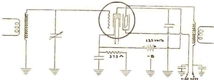
Connections of a-c. pentode used with separate battery for space charge grid
