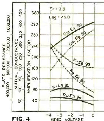
FIG. 4 Amplification constant, plate resistance and mutual conductance.
