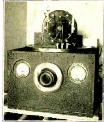
View of one oscillator unit—of the new radio "yardstick."
