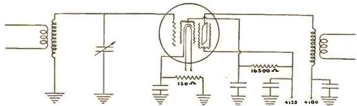
Connections of a-c. pentode providing space charge potential from power pack
