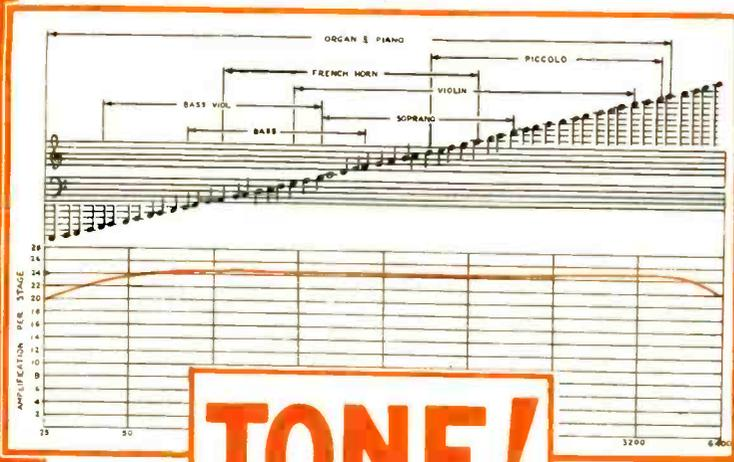
Curve of Type "A" Sangamo Straight Audio Transformer showing uniformity of amplification at all audible frequencies.
