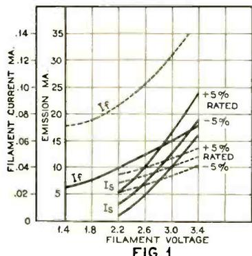
FIG. 1 Emission and filament current.
