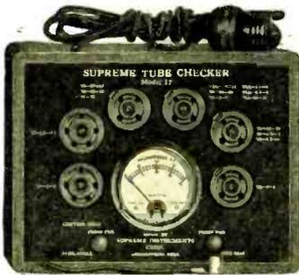
graved on the panel. There are no rheostats to regulate. Tests both types of type -80 rectifier tubes separately. It has a standard milliammeter, genuine D'Arsonval movement (either Jewell or Weston meter). It is housed in a moulded bakelite case with carrying strap.
