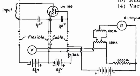
Figure 2—Vacuum Tube Voltmeter
