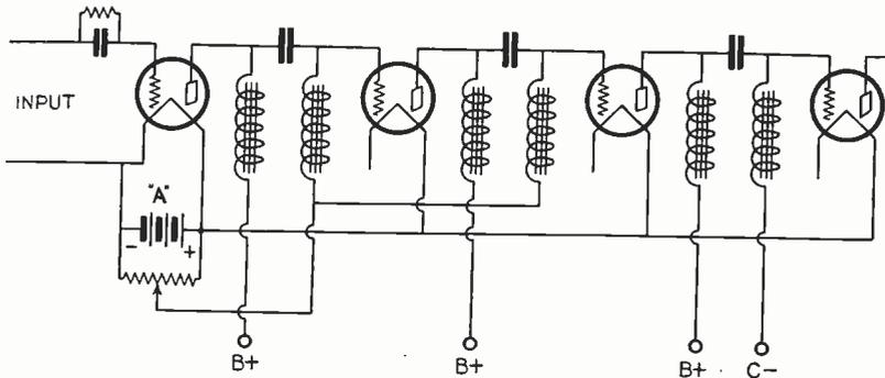
Fig. 7. Second harmonic distortion can be eliminated and the overall A. F. regeneration controlled by the use of a potentiometer for grid biasing.
