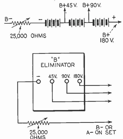
Fig. 9. A. F. regeneration can be promoted by inserting a variable resistance in the common "B" supply lead.
