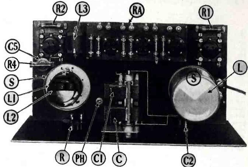
Top view of the Interbalanced Regenerative Receiver. The right-hand shield encloses the antenna coupler. The list of parts below provides the key to the symbols.
