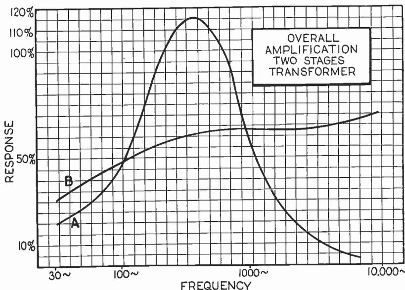
Fig. 1. Two curves obtained from a transformer coupled amplifier. Curve A shows the effect of audio frequency regeneration.
