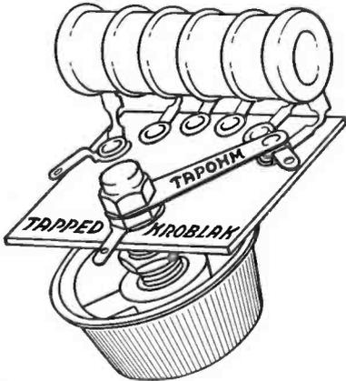
The Mountford tapped resistance unit designed expressly for "B" eliminators.
