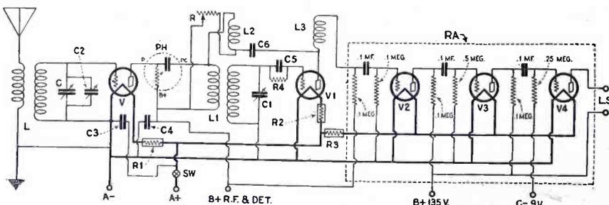
The schematic diagram of the Interbalanced Regenerative Receiver. Note that the radio frequency currents in the plate circuit of the detector tube are by-passed through the condenser C6.
