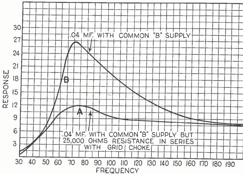
Fig. 2. Two frequency response curves obtained from a tuned double impedance amplifier. Curve B shows the effect of audio frequency regeneration.
