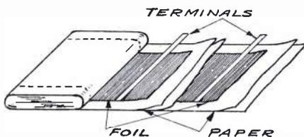
Fig. 1. The inductive type of condenser winding
