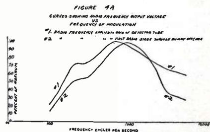
quency amplifier is too sharp the higher audio frequencies will not go through it, because the circuit will have very little response to: first, the frequency of the carrier plus the frequency of modulation; and second, the frequency of the carrier minus the frequency of modulation. The latter
