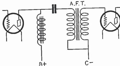
Fig. 5. An "engineered" transformer coupled stage which provides slightly better frequency characteristics.
