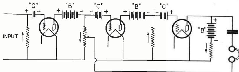
Fig. 8. Illustrating phase relations in the circuits of a non-reactive A. F. amplifier.
