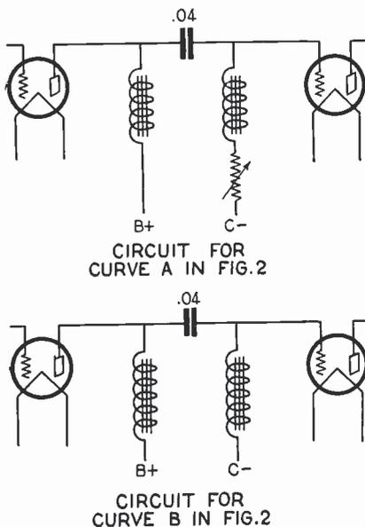
Fig. 6. A. F. regeneration can be controlled by inserting a variable resistance in the grid leg of the tube as shown in the first circuit.
