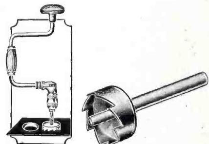
An efficient panel cutter for making bezel holes, etc. The cutters can be had in various sizes.
