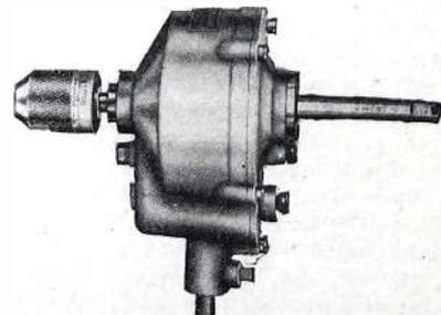
The Ettco electric driven, high speed tapping machine.
