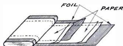
Fig. 2. The non-inductive type of condenser winding
