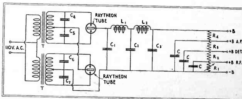
Schematic diagram of heavy duty plate supply unit
