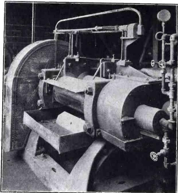
Huge rolls are used to insure the thorough incorporation of resin and filler in making molding powder.
