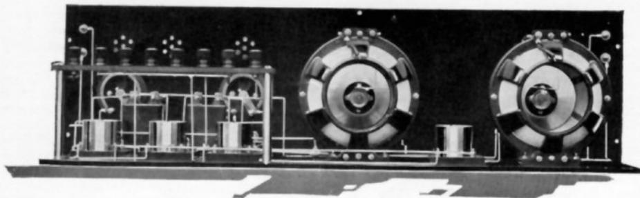
Fig. 2. The terminal panel at the rear carries the eight binding posts for connections to the batteries. You can see how the tuning units are arranged
