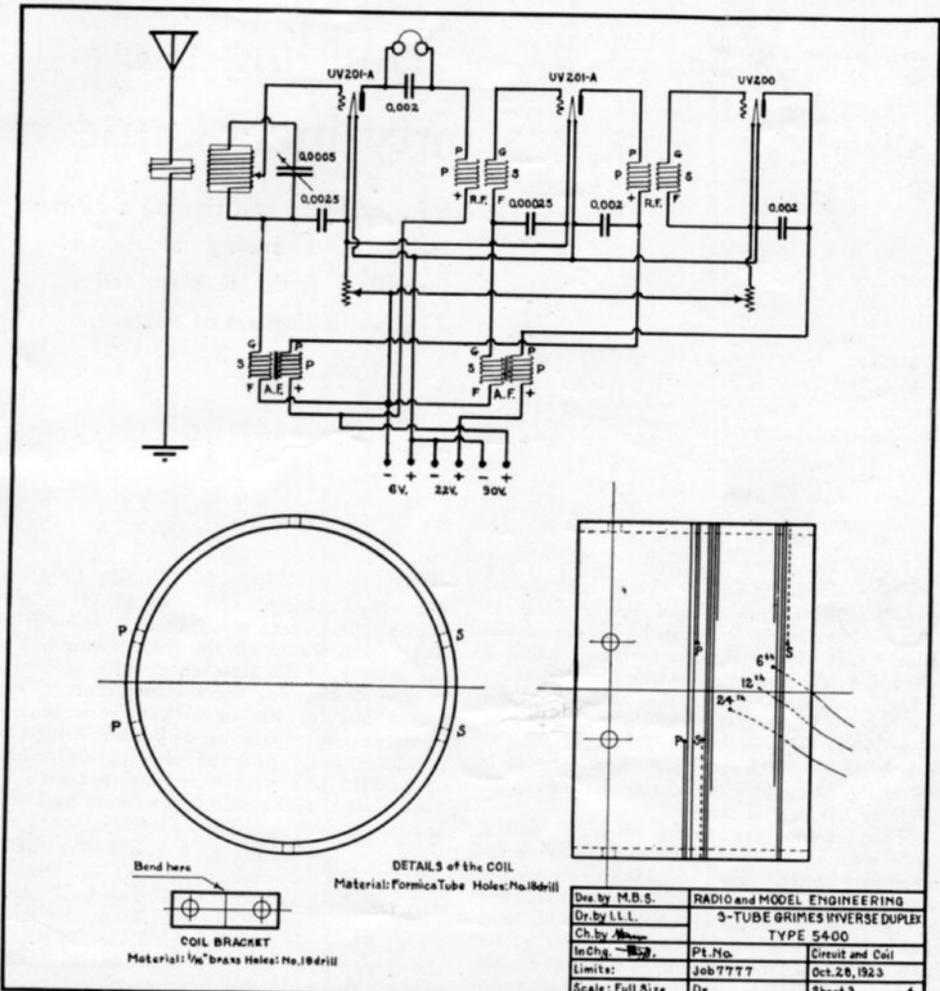
Fig. 7. Above, The Schematic wiring diagram of the three-tube Grimes Set, in which the latest improvements are incorporated. Below, details of the coil and coil brackets
