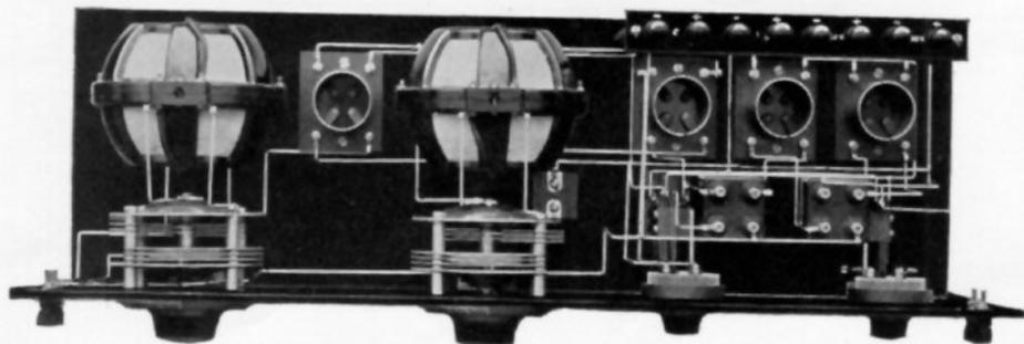
Fig. 1. Very attractive is the arrangement of this four-tube receiver, permitting the parts to be conveniently located while the leads are kept very short
