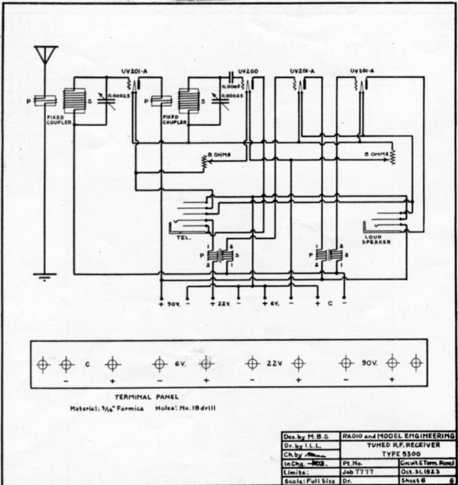
Fig. 9. Schematic wiring diagram of the set, illustrating the system of connections. The terminal panel is shown one-half size
