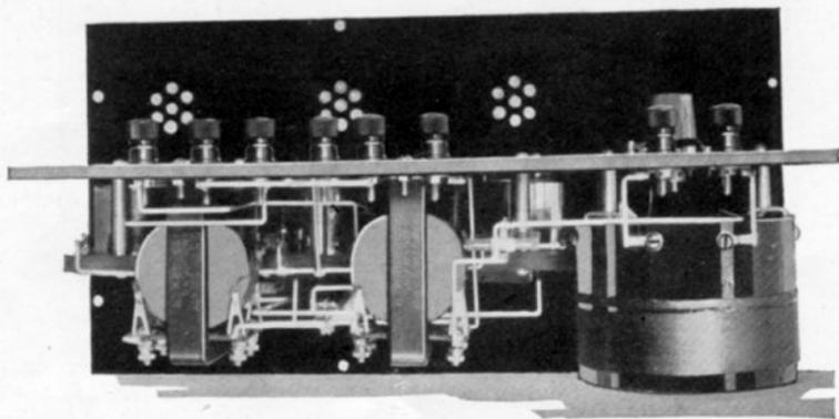
Fig. 1. The rear view illustrates the method of mounting the sockets and the arrangement of the A. F. transformers and coupler
