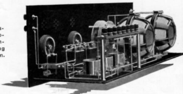
14. Connect 45 to 46. 46 is the right hand primary terminal. Connect 49 to 50, and 51 to 52. Terminals 50 and 51 are made by putting  $\frac{1}{2}$ -in. 6-32 R. H. screws through the condenser holes and fastening on soldering lugs with 6-32 nuts. Scratch the condenser plate and put a little drafting ink across the condenser terminals to serve as a leak. The exact amount can be regulated when the set is in operation. Connect 53 to 54. 54 is the secondary terminal. Connect 55 to 56 and 57 to 58.
