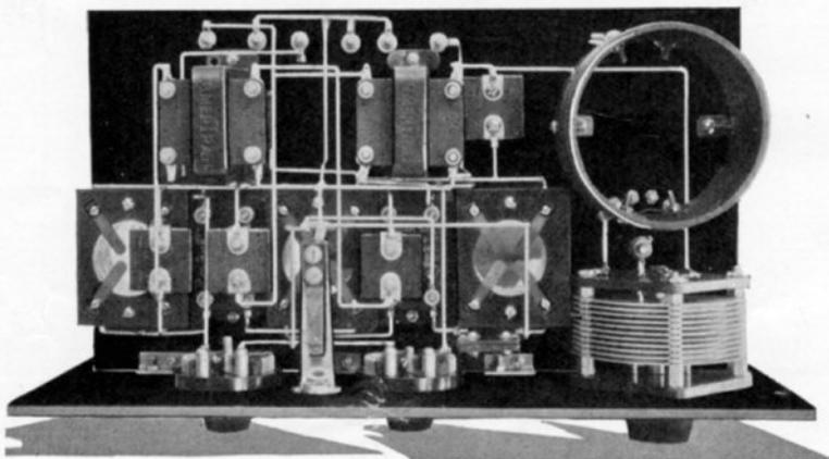
Fig. 2. Looking at the under side of the base panel. The R. F. transformers are almost hidden by the Micadons and the sockets
