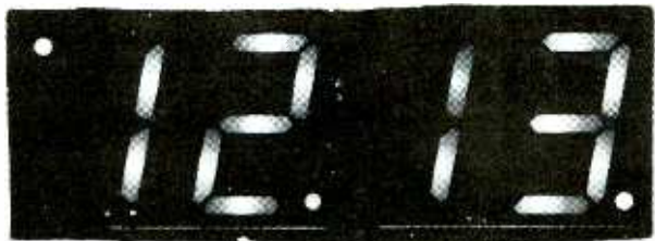
THE NUMERIC DISPLAY HAS THREE DOTS. The flashing dot in the center is the colon. The dot at the upper left indicates PM. The dot at the lower right indicates the timer is turned on (armed).
