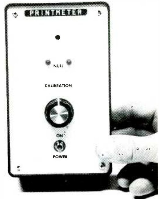
THE COMPLETED PRINTMETER. To make viewing easier a "target" cut from a white self-adhesive label can be placed around the LDR opening. Make certain, however, that no part of the opening—no matter how little—is covered by the target.
