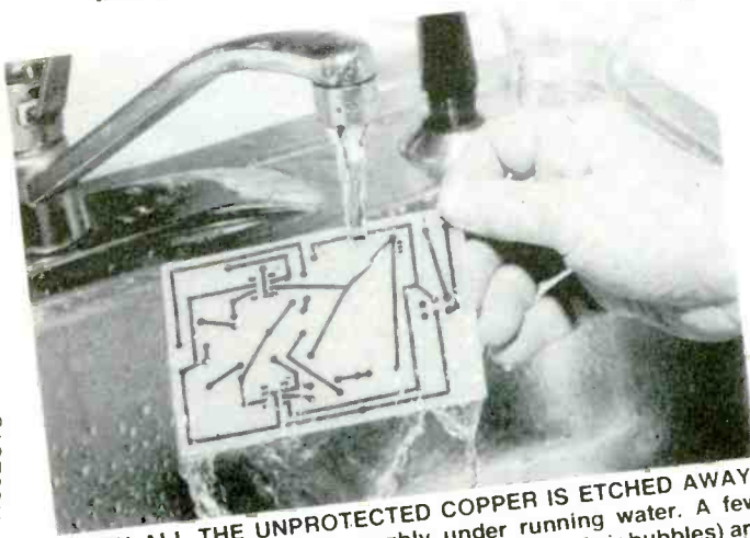
PLACE THE PCB FACE UP in a plastic or glass tray (shallow Rubbermaid drawer trays are excellent for etching) and pour the etchant to a depth of at least \frac{1}{4} inch. Agitate the tray frequently to speed etching and avoid air bubbles from isolating the etchant from the copper. The etchant splashes easily and stains badly, so do the whole thing in a sink. Some etchants are supplied in a plastic bag into which you slide the PCB. Either way is OK, though the plastic bag is neater, almost splash-free, and somewhat faster; though it's more difficult to check the board to see if the etching is completed.
