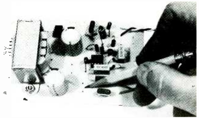
PENCIL POINTS TO THE SPACE available for two extra 500- \mu F filter capacitors. They are used only if you cannot obtain 1000- \mu F electrolytics.
