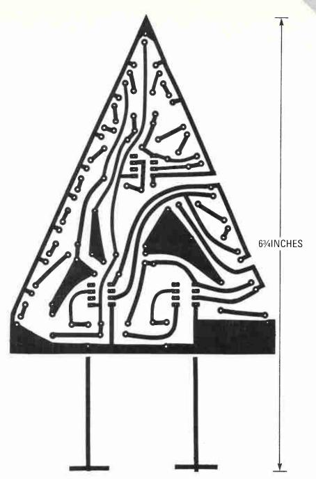
LIGHT UP THE HOLIDAYS with the electronic Xmas tree. The PC board for that project is shown here.
