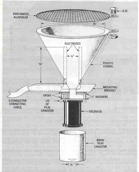
FIG. 2—TWO ¼-INCH ELECTRODES, made of copper and lead, are mounted inside the funnel, spaced ½-inch apart. A solenoid valve attached to the mouth of the funnel is used to drain it as necessary.
