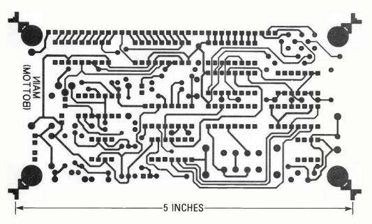
THE SOLDER SIDE of the digital tachometer is shown here.
