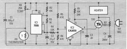
FIG 22—HEATER CONTROLLER with precision temperature regulation.
