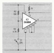
FIG 13—ALTERNATE CA3059 zero-voltage switch.
