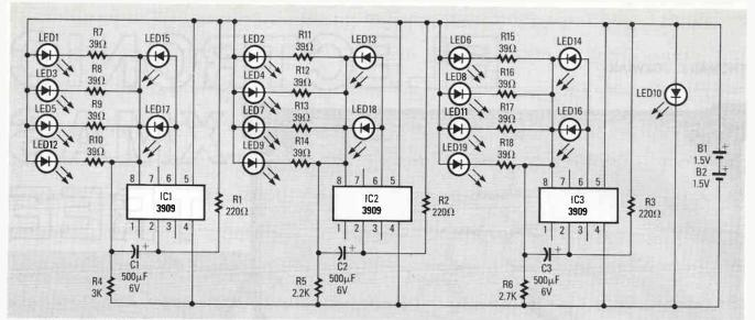
FIG. 1—THREE INDIVIDUAL FLASHER CIRCUITS having unrelated flash rates create a pseudorandown blinking of the LED's because the LED's from each individual circuit are intermixed around the edges of the tree.
