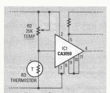
FIG 21—HEATER CONTROLLER with thermistor-regulated zero-voltage switching.
