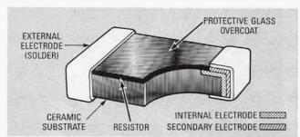
FIG. 3—INSIDE A LEADLESS CHIP RESISTOR. The construction is identical to a that of a thick-film resistor deposited directly onto a ceramic substrate.
