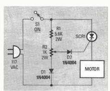
FIG 28—SELF-REGULATING UNIVERSAL MOTOR heavy-duty speed controller.
