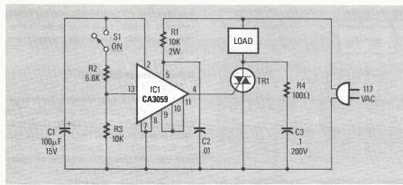
FIG 12—ZERO-VOLTAGE line switch built from the CA3059.
