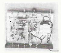
FIG.5—THE SAP BOARD MOUNTS directly onto the BTSC board. Notice the modifications (extra switch, wiring, LED, etc.) that have been made to the chassis in order to accommodate the SAP decoder.
