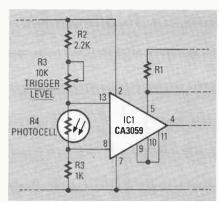
FIG 18—DARK-ACTIVATED zero-voltage switch with hysteresis.
