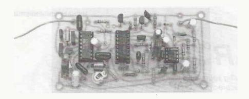
FIG. 3—THE COMPLETED SAP BOARD. Notice that only two wires have to be connected to the stereo decoder.
