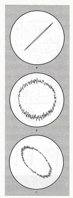
FIG. 11—OSCILLOSCOPE DISPLAYS of the decoder's left and right outputs. Shown in a is a mono signal (L+R); in b is a signal with proper left/right separation; in c is a signal with too much L-R.
