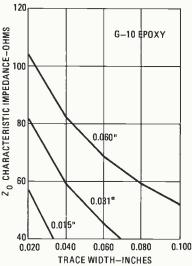
FIG. 4—USE THIS CHART to determined microstrip trace width for various impedances and thicknesses of G-10 epoxy board.
