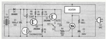
FIG 20-THERMISTOR-SWITCHED heater controller.
