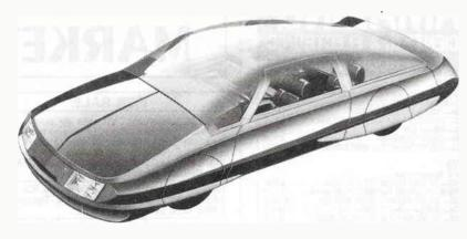
THE ALL-GLASS TOP OF FORD'S 2001 MODEL is flush with the body, giving the car execellent aerodynamic performance.
