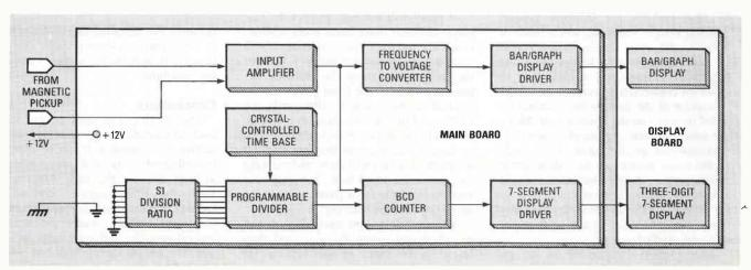
FIG. 1—BLOCK DIAGRAM OF THE SPEEDOMETER: The input amplifier conditions the signal from the magnetic pickup for processing by the counting and display circuitry.
