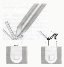
FIG. 4—A PROPERLY-SOLDERED terminal connection looks like this.
