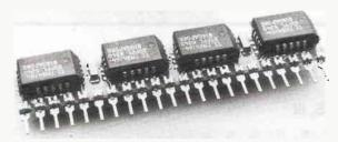
FIG. 2—SMT CAN REDUCE the area of circuit boards. This small Texas Instruments' memory module is made from four SMT 64K  $\times$  1 RAM's and four chip capacitors.
