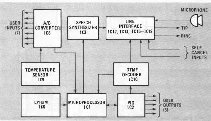
FIG. 4—BLOCK DIAGRAM OF THE CONTROLLER: an analog switch (IC14, not shown) connects the internal microphone, the speech synthesizer, or one of the self-cancel inputs to the phone line.
