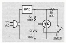
FIG 1—AC POWER SWITCH, AC triggered.
