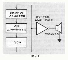
circuit consists of four parts: a binary counter, a D/A converter, a VCO, and an audio output amplifier. The speed at which the counter counts depends on the frequency of the output of the VCO, which in turn is determined by the output of the counter. That feedback loop is what gives this circuit its characteristic output.
