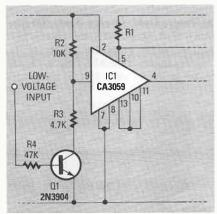
FIG 14—TRANSISTOR-CONTROLLED CA3059 switch.
