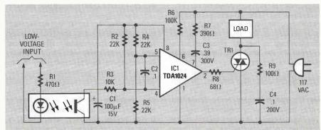
FIG 16-OPTICALLY COUPLED TDA1024-based zero-voltage switch.
