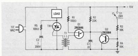
FIG 8—ISOLATED-INPUT AC power switch. The Triac turns on when S1 is open.
