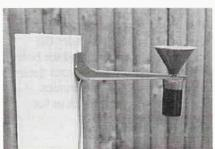
FIG. 6—THE SENSOR ASSEMBLY should be mounted on a long bracket that is screwed to a post. The post should be mounted away from overhanging eaves; and don't mount it under a tree.
