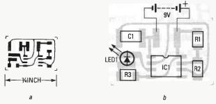
FIG. 3—USE THE PC PATTERN shown in  $\boldsymbol{a}$  to etch the board. The parts layout is shown in  $\boldsymbol{b}$ .
