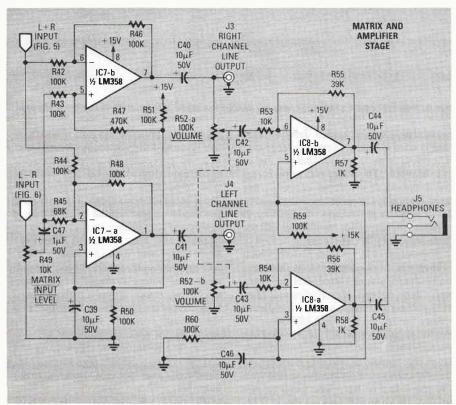
FIG. 5—THE MATRIX STAGE separates the L+R and L-R signals into the left- and right-channel components. Op-amp IC8 and associated components provide an optional headphone output. If you do not wish to drive a pair of headphones, or plan to use your amplifier's headphone jack for that purpose, all components to the right of jacks J3 and J4 can be deleted.
