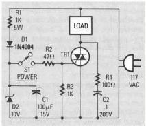
FIG 2-AC POWER SWITCH, DC triggered.
