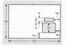
FIG. 6—BASIC DIMENSIONS for the front panel.
