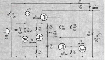
FIG 25-UJT-TRIGGERED zero-backlash lamp dimmer.
