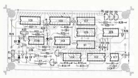
FIG. 6—STUFF THE MAIN BOARD as shown here, and, after checking both boards for errors, connect them together with 35 pieces of short bare wire. The solder sides of the board should face each other.
