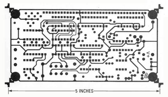
THE COMPONENT SIDE of the digital tachometer.
