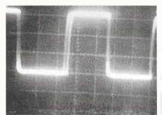
FIG. 2—FURTHER INVESTIGATION found a waveform with a timing shift during alternate leading edges.
