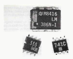
FIG. 10—TWO SO INTEGRATED CIRCUITS and a conventional 8-pin mini-DIP.
