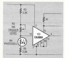
FIG 17—DARK-ACTIVATED zero-voltage switch.
