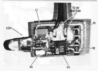
FIG. 4—THE COMPLETED CIRCUIT BOARD. The light from the superbright LED can be seen for several hundred feet.
