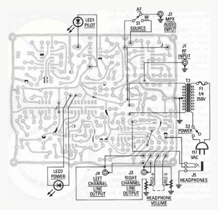
FIG. 8—THREE JUMPERS AND ALL OFF-BOARD components mount as shown here.
