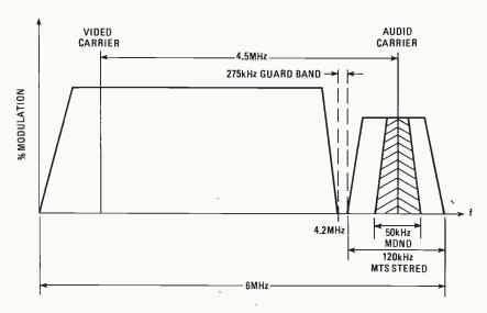
FIG. 1—STEREO-TV AUDIO requires about twice the bandwidth of a mono signal.
