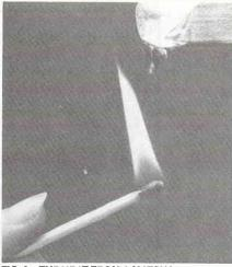
FIG. 9—THE HEAT FROM A MATCH is enough to melt a bar of inclum fusible-alloy solder.
