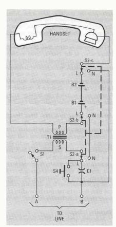
FIG. 4—A SIMPLIFIED RED BOX. Switch S2 lifts the handset from the telephone line and connects two D-cells as a local power supply. The circuit is DC-isolated from the telephone line even when hook switch S1 is closed.
