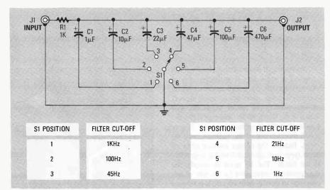
FIG. 4—GRAVITY DETECTOR OUTPUT FILTERING will limit the detectors response to certain astronomical distances. The lower cut-off frequencies of 21 Hz to 1 Hz are best for gravity sensing within our own galaxy. Most of the author's chart recordings were done using a 10 Hz filter. The filter should be placed in a RFI shielded enclosure.
