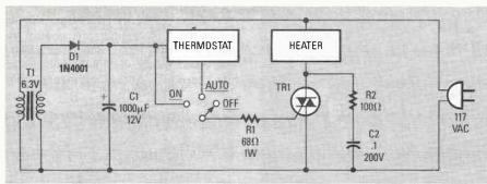
FIG 19—THERMOSTAT-SWITCHED heater controller.
