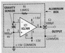
FIG. 2—THE BASIC GRAVITY DETECTOR is a current-to-voltage converter. The current through capacitor C1 is proportional to changes in the strength of the gravity field. IC1 amplifies the signal generated across capacitor C1 to drive a chart recorder or digital multimeter.
