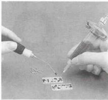
FIG. 12—IT TAKES TWO HANDS to position an SMD device on a PC-board: one for the cream dispenser, the other for the vacuum holder.
