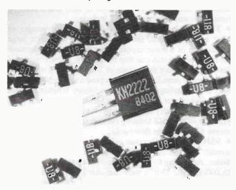
FIG. 9—A TO-92 TRANSISTOR dwarfs its SOT-23 counterparts.
