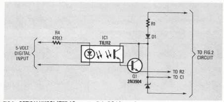
FIG 3—OPTICALLY ISOLATED AC power switch, DC triggered.
