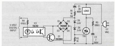
FIG 4—OPTICALLY ISOLATED AC power switch, AC triggered.
