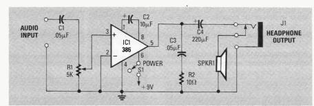
FIG. 5—A SIMPLE AUDIO AMPLIFIER can be used to listen to gravity signals that sometimes contain a musical rhythm.
