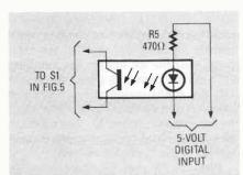
FIG 6—TRIGGER THE PREVIOUS CIRCUIT with an optocoupler.
