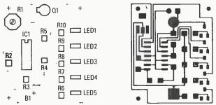
FIG. 3—USE THIS LAYOUT a when building the circuit. The PC board is shown in b.
