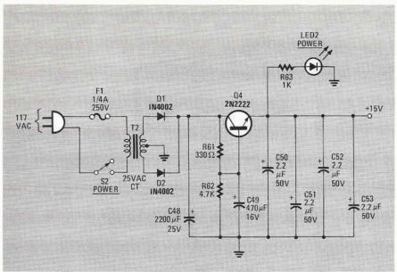
FIG. 6—THE UNREGUALTED POWER SUPPLY shown here provides extremely low ripple for the MTS decoder.
