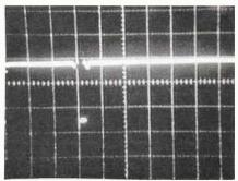
FIG. 5—A CAMERA/VCR SETUP is ideal for viewing short duration transients, such as a voltage interruption caused by a relay's contact bounce.
