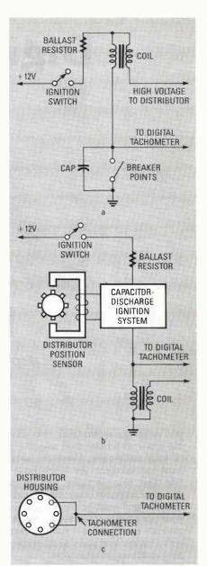
FIG. 8—TO INTERFACE THE TACHOMETER, follow one of these circuits. A conventional (Kettering) ignition system is shown in (a), a capacitor-discharge system in (b), and a General Motors hook-up in (c).
