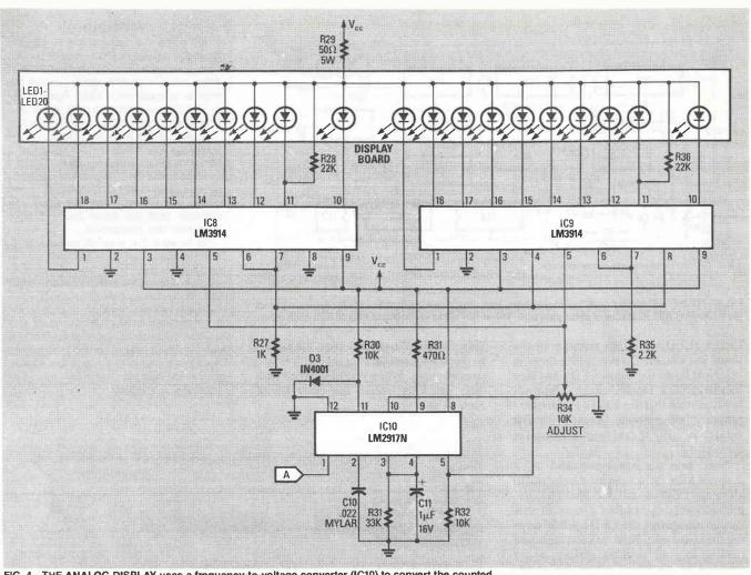
FIG. 4—THE ANALOG DISPLAY uses a frequency-to-voltage converter (IC10) to convert the counted pulses into displayable form.
