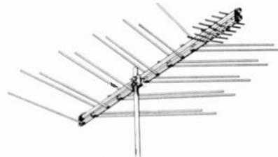
THE BLONDER-TONGUE PRISMATIC series combines several principles discussed in text. Twin booms with staggered elements at log-periodic spacing contribute smooth channel-to-channel response across vhf band. Forward sweep improves front/back ratio and forward gain. Uhf array is merely continuation of design for vhf, except that dipole elements are not swept forward into vee.
