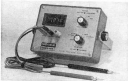
solid-state construction. Unit measures ac volts, dc volts and ohms in four ranges for each type of measurement.—**Nobex Electronics Division, Griffith Plastics Corp.**, P.O. Box 4365, Burlingame, Calif. 94010.
