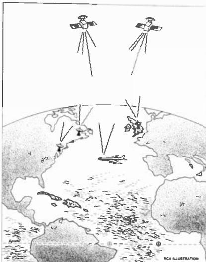
**AERONAUTICAL SATELLITE PROGRAM** would use two geostationary satellites, working with ground stations to provide exact position information on and direct communication with the aircraft during the whole transatlantic flight.
