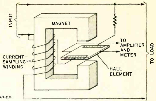
Fig. 4—Hall-effect wattmeter responds to frequencies over a wide range.
