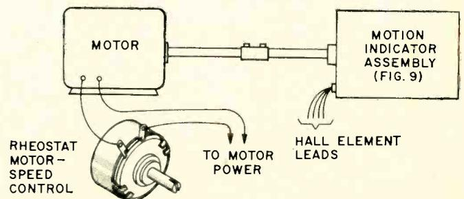
Fig. 11—Spinning shaft in Fig. 9 generates alternating voltage.
