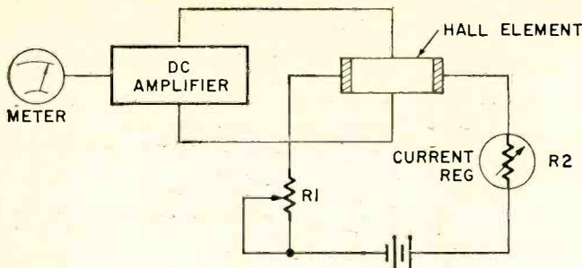
Fig. 3—Basic setup for measuring magnetic field strength with Hall device. As battery ages, R2 regulates current.
