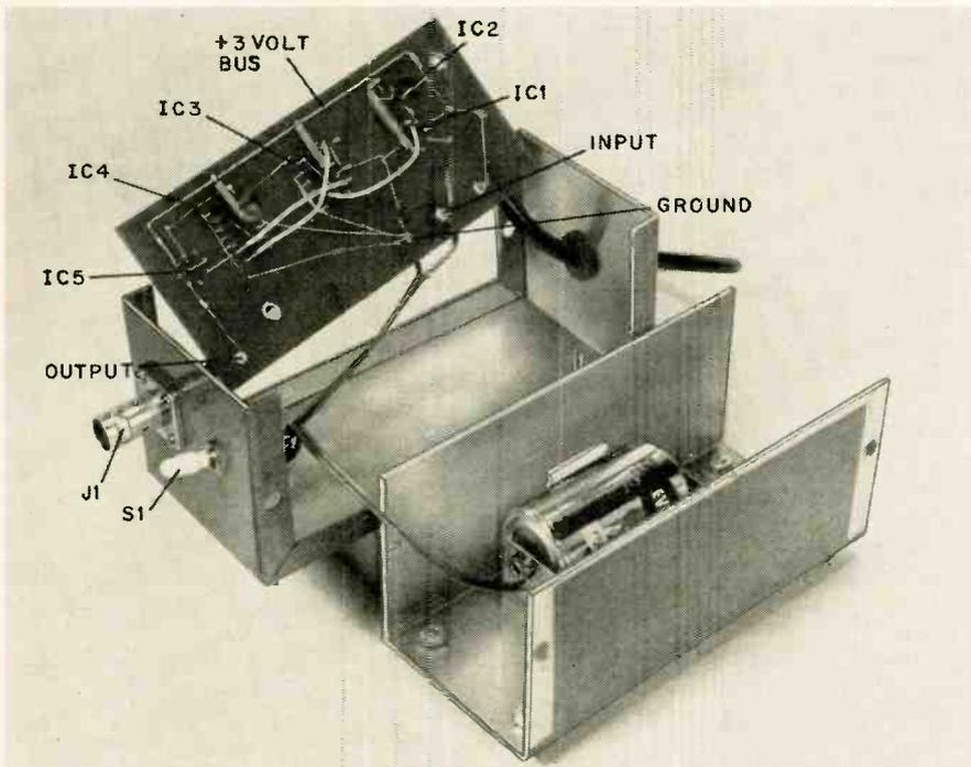
Fig. 8—An underside view of the board before final installation in the box.
