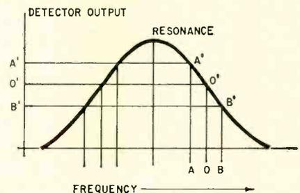
Fig. 10—In slope detection, carrier is tuned to point 0. Capacitance changes may cause carrier shift to points A or B.
