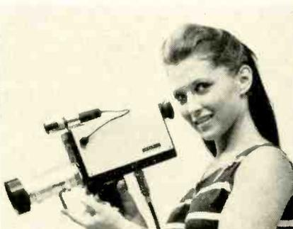
lb and operates on a self-contained battery. It records black-and-white pictures, with sound, for immediate playback on CV-2000 series video tape recorders. Device uses a 20-minute,  $\frac{1}{2}$ " tape with a 7 $\frac{1}{2}$ " ips speed. Only 2 buttons are used
