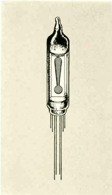
The original electron-ray indicator tube was the 2E5 with a 2.5-volt heater, and its 6.3-volt counterpart—the 6E5—shown in Fig. 1-a. The plate of one triode section (a dc amplifier) is connected internally to the ray-control electrode (grid). The plate of the second triode is known as the target.
