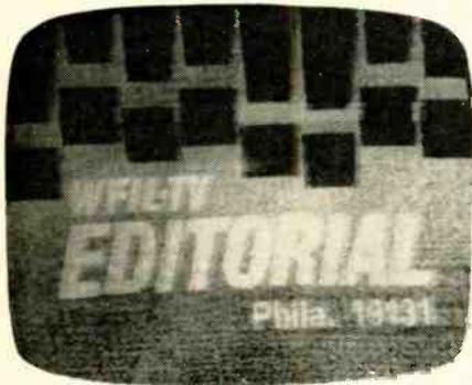
Fig. 4—TVI from upper adjacent channel results in "floating" background picture. TVI blanking produces framing lines.
