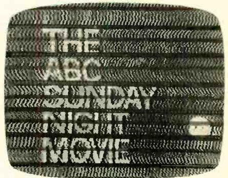
Fig. 6—Multiple interference. Herringbone pattern and horizontal bars are due to sound and lower channel traps.
