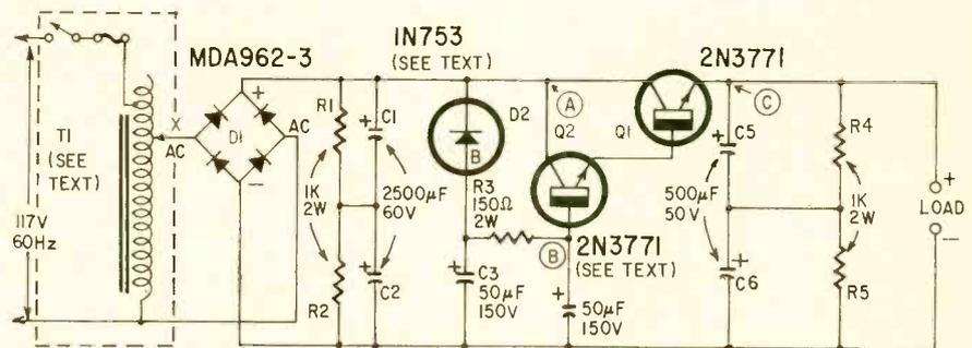
Fig. 1—High-efficiency dc supply for delivering up to 6 amps into 15-ohm load. C4, the 50- $\mu\text{F}$  electrolytic tied to Q2's base, is part of current-control network.
