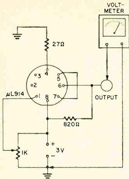
Fig. 2—External circuit connections shown will adopt  $\mu\text{L914}$  as a Schmitt trigger. Critical firing point is determined by adjusting pot while monitoring output.
