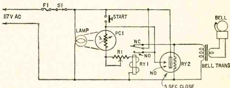
time-delay relay RY2 through the normally closed contacts of RY1. The bell will start ringing and can be turned off by pushing the START button.
