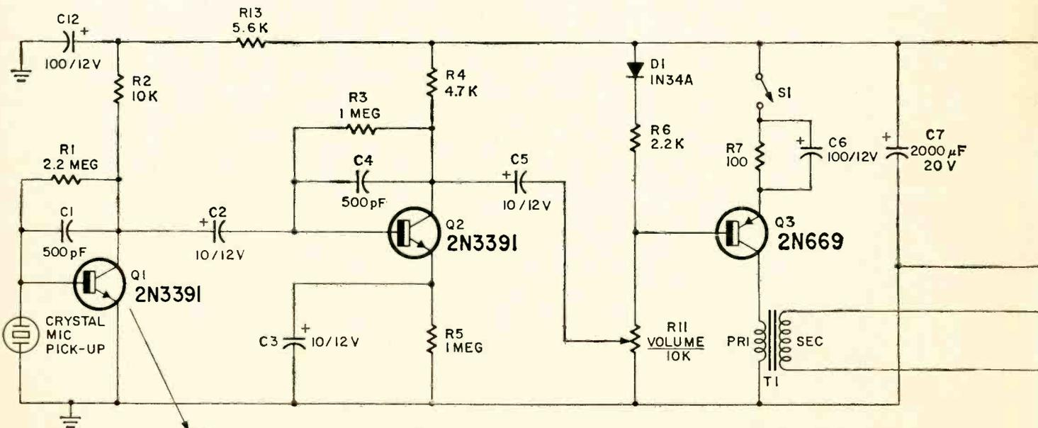
**ECB** BOTTOM VIEW OF 2N3391 Fig. 1—Transformers isolate the signal and power section's low and high voltages. Transistors Q1 and Q2 may be substituted with similar types, as stage design isn't critical.
