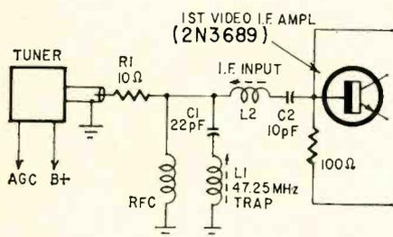
Fig. 7—i.f. input circuit of a Sylvania AO7-1 solid-state TV. Trap C1-L1 is used to reject adjacent-channel sound.
