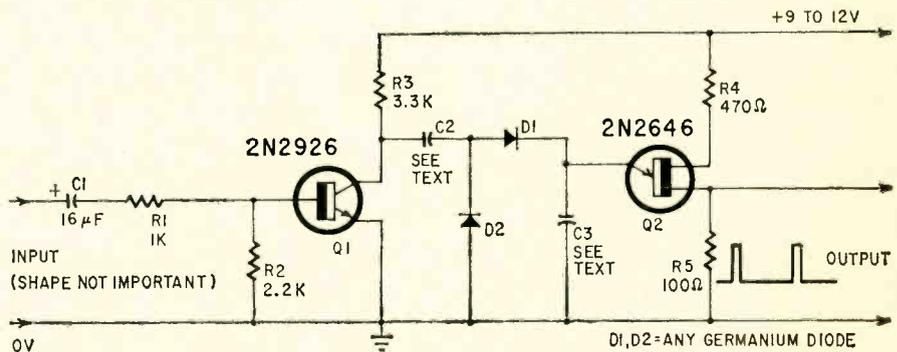
Fig. 2—Diode pump counter.
