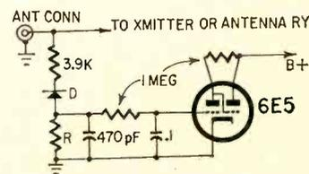
Fig. 5—Transmitter monitor: Output is rectified by the diode. Voltage across R controls 6E5 shadow width.
