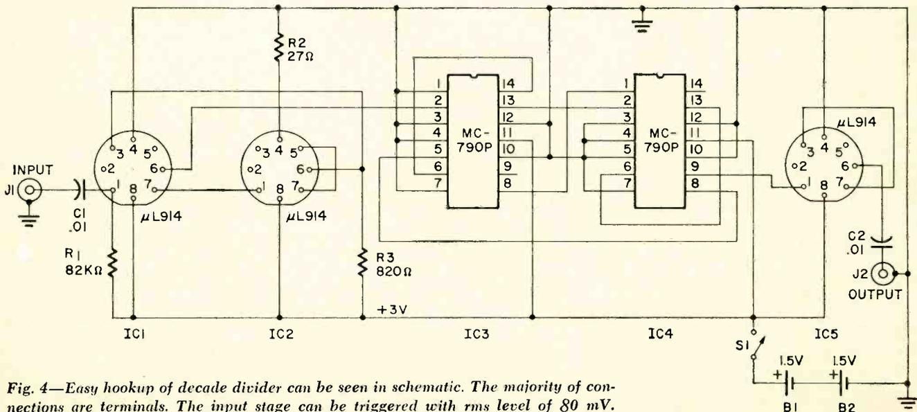
Fig. 4—Easy hookup of decade divider can be seen in schematic. The majority of connections are terminals. The input stage can be triggered with rms level of 80 mV.
