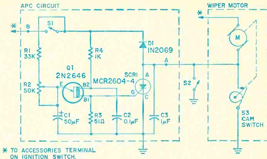
FOR 6-VOLT SYSTEM, REPLACE R4 WITH JUMPER WIRE, REDUCE R1 TO 15,000 OHMS
