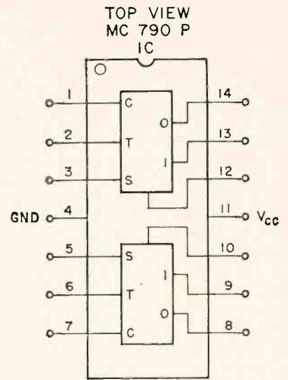
Fig. 9—Pin connections for the Motorola MC790P integrated circuits (IC3, IC4).
