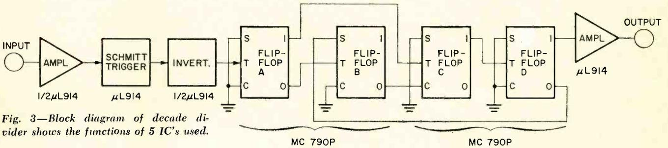
Fig. 3—Block diagram of decade divider shows the functions of 5 IC's used.
