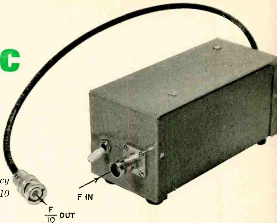
WANT TO UPGRADE THAT OLD 100-KHz electronic counter to 1 MHz? Then read on and find out how you can easily and cheaply construct a battery-powered, in-line type decade divider (semiconductor cost less than \$7.50). At the same time you will get a chance to work with a few of the many applications afforded by today's low-priced logic circuits.
