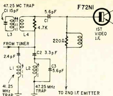
Fig. 9—The Magnavox T-908 has a series-resonant shunt trap and a parallel-resonant absorption trap to obtain better adjacent-channel signal rejection.
