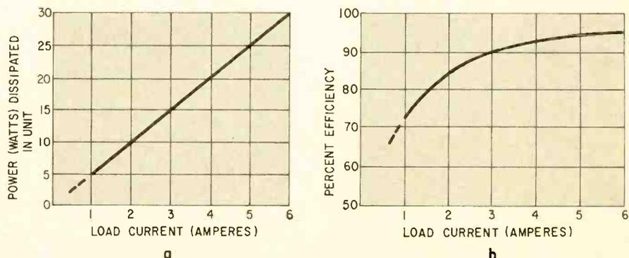
Fig. 3—Dissipation in the supply in Fig. 1 is shown in graph a; efficiency in b.
