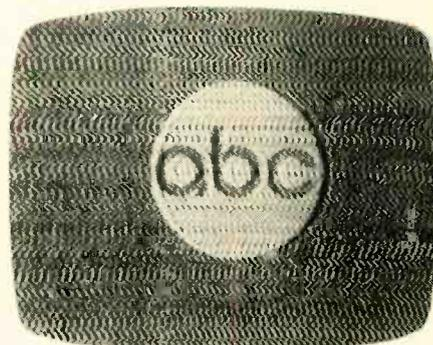
Fig. 3—Herringbone pattern superimposed on the picture is result of sound interference from the lower adjacent channel.
