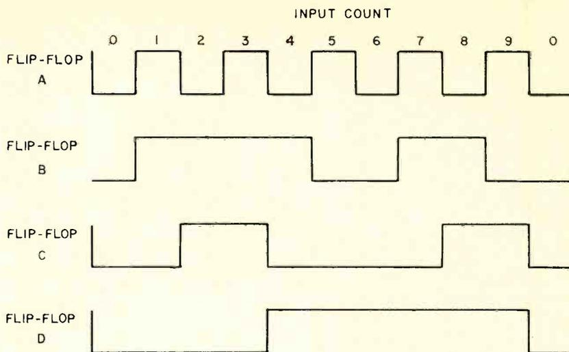
Fig. 5—Divider action is shown by these flip-flop output waveforms.
