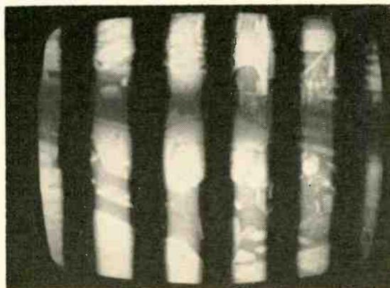
Fig. 12—Screen displays ringing bars caused by diode failure generating Fig. 11 waveform picture.
