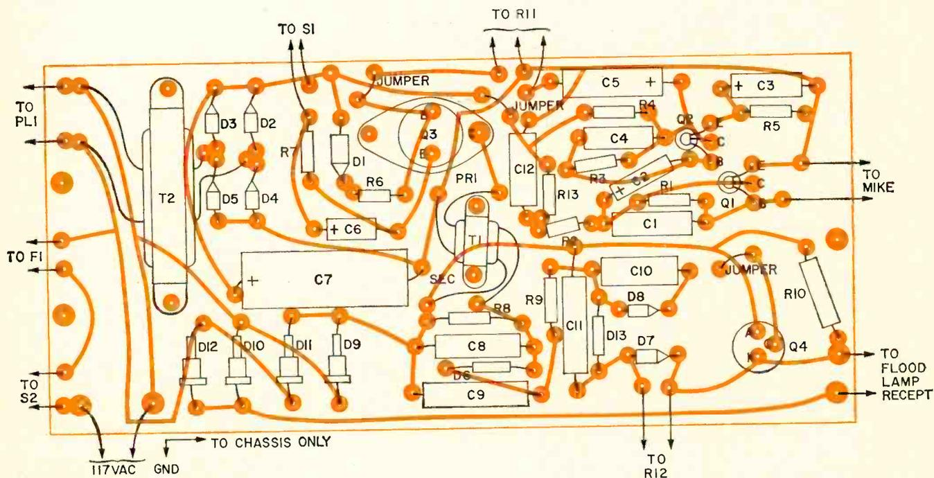
Fig. 2—Lay out parts on the board and solder carefully before mounting board to chassis. Watch electrolytic and diode polarities.
