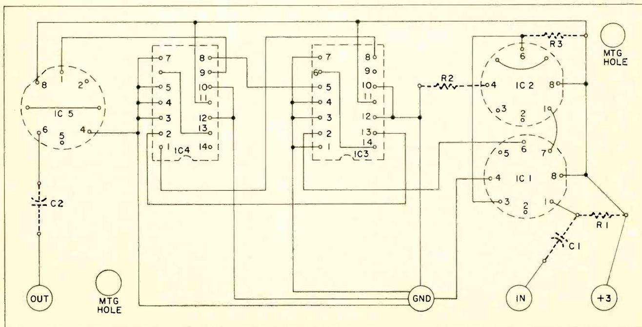
Fig. 6—Author used a glass fiber board for parts mounting; a perforated phenolic board would do just as well.
