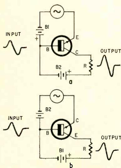
Fig. 3—An npn grounded-base transistor amplifier (a) has high power and voltage gains with slight current loss. Transposing emitter and collector and reversing bias polarities (b) results in considerable current loss, moderate voltage gain and possibly some power gain as well.
