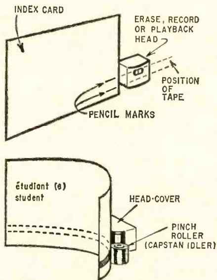
To prepare language cards, remove tape-head cover and position file card near head and flush with baseplate. Mark top and bottom of playback-head gap on card. Next, apply rubber cement to the card (where marked) and the glossy side of tape. Carefully position tape on card, removing all excess glue. Record words while feeding cards between capstan and capstan idler. Write words on card backs.
