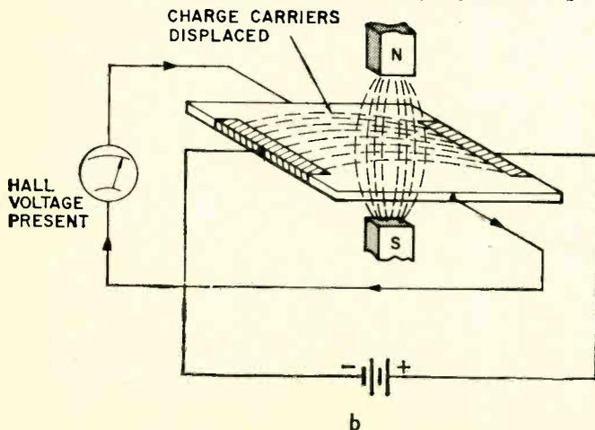
ence between opposite edges. When the magnetic poles are reversed, the polarity of voltages generated are reversed.
