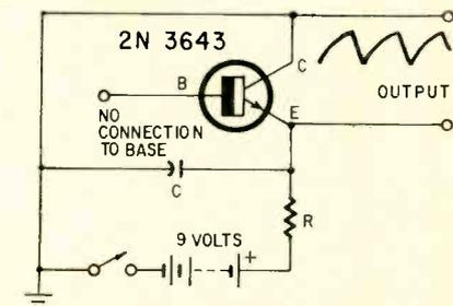
Fig. 5—Circuit of the solid-state "glow-lamp" oscillator. Pulse rates up to about 100 kHz are possible with appropriate values of R and C. Frequency is about 1 kHz when R is 1200 ohms and C is 1  $\mu$ F.
