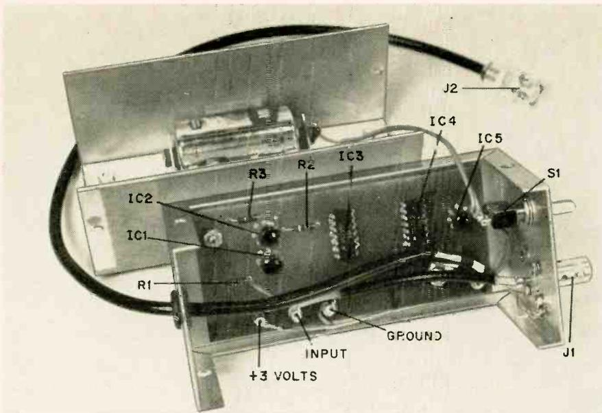
Fig. 7—Circuit board should be just a little smaller than the aluminum box you use. Mount the board on standoffs. Carefully recheck pin indentifications.
