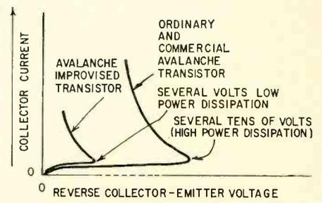
Fig. 2—Comparative  $I_C-V_{CB (rev.)}$  curves for ordinary and avalanche transistors and for the avalanche transistor adapted for use as a low-voltage oscillator. Low power dissipation aids circuit stability.
