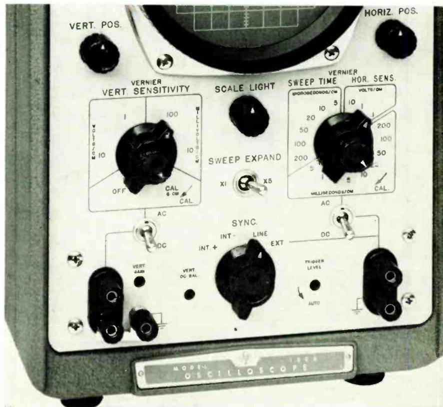
Fig. 9—Professional scope with time-calibrated sweep and attenuators.
