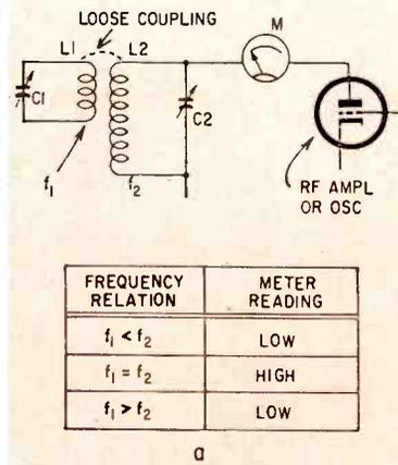
Fig. 2—Basic dip-meter principle. Meter (a) will read high as long as circuit frequencies do not coincide; when they do, meter dips.
