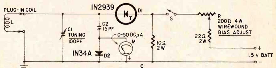
Fig. 3—Three basic dip meter circuits: a—Tube design with ac power supply; b—Transistor version, battery operated; c—Tunnel-diode type, battery operated. In all circuits, plug-in coils are wound to cover desired frequency range with capacitor used. See data in various radio handbooks.
