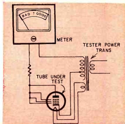
An emission tester is a useful tool, but tubes that check good on it may still work erratically or not at all in their circuits. It tests emission of tubes by tying all elements except cathode to plate and indicating relative plate current on meter.
