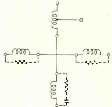
You'll have to check the schematic carefully on each set to get the horizontal coils hooked up right. Even then, you'll get odd effects on a few of them from a slight mismatch. However, the scheme *might* be made to work fairly well. You'll find a difference in sweep between the 90° and 110° sets, for it takes quite a bit more power to sweep a 110° tube. However, if you remember and don't waste time trying to find the cause of a narrow raster, it could be OK.
