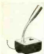
**PAGING MICROPHONE**, the *MK-3DBS*, controls as many as 4 separate circuits for paging, dispatch, PA, audio-visual work, ham operation. Dynamic, low impedance (200 ohms), response 80-10,000 cycles. Weighted base, momentary action dpdt switch, adjustable gooseneck. 12-ft shielded multiconductor cable. *MK-3BS-1* is high-impedance ceramic mike with same features as listed above. Response 80-8,000 cycles. Output level -52 db at 1 kc.—Audiophonics Corp.
