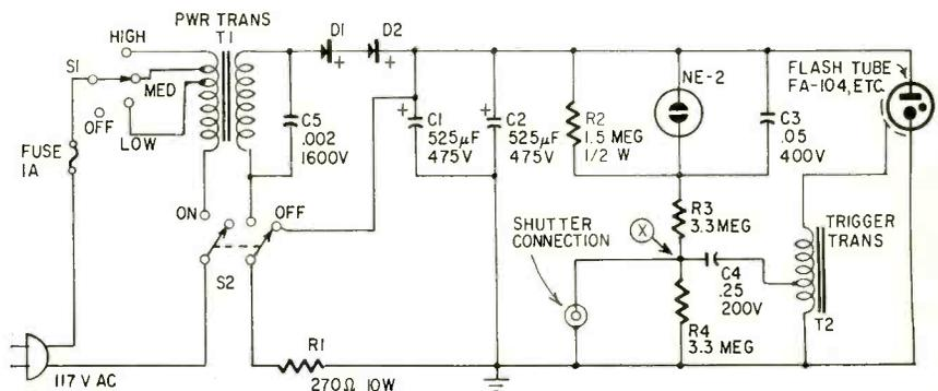
Fig. 1—Typical small electronic photoflash unit (from Sprague Electronic Flash Handbook). Direct discharge of C4 through shutter contacts for triggering can damage contacts quickly.
