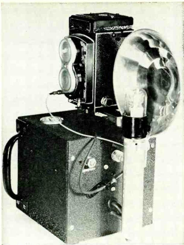
*Author's flash is built into rugged steel box. Meter is visible on top surface of box, just under flash sync wire. Sensitivity control, with locking nut, is R7 in Fig. 2.*
