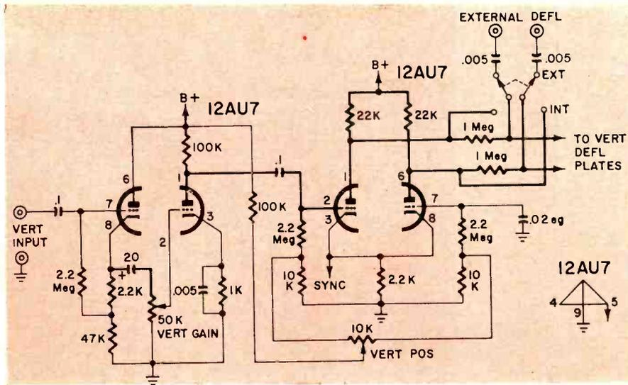
Fig. 2—Original vertical deflection amplifier in 3-inch Heath OL-1 (newer IO-21 is very similar). Wiring and parts shown as heavy lines affect bandwidth seriously.
