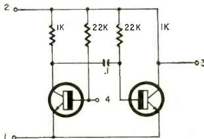
When it is oscillating, only one transistor is conducting at a time. Therefore, input current is reduced by about 50%.
