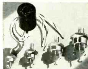
lation. Color-coded wires have solderless terminals.—Azimuth Electronics
