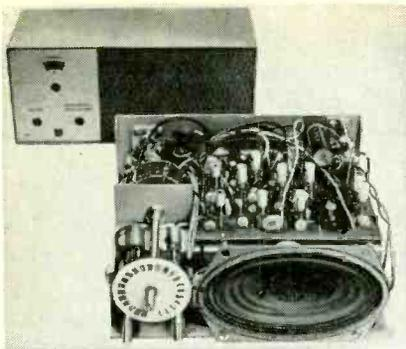
**23-CHANNEL CB TRANSCEIVER**, the 23'er, 25 silicon transistors, 6 diodes, 1 Zener diode. Ignition-noise silencer; crystal bandpass filter; 3 x 5 in. speaker; 4 watts maximum audio; PA service; power 12 volts dc, negative ground; separate 115-volt ac power supply; full 5 watts input to transmitter. 8 x 3½ x 7 in., 4 lb.—Squires-Sanders, Inc.
