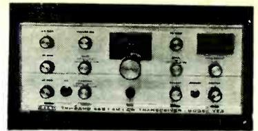
µv for 10 db signal-to-noise ratio. Selectivity from crystal lattice bandpass filter is 2.7 kc at 6 db. Receiver has offset tuning over 10-kc range. Frequency range: 3,490-4,010 kc, 6,990-7,310 kc and 13,890-14,410 kc. Flat-topping prevented by automatic level control. Available wired.—EICO Electronic Instrument Co.
