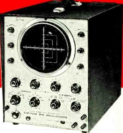
*The Jackson CRO oscilloscope was designed as a wide band scope when color TV first made its entry into the field. It is widely used by professionals who laud its stable circuitry, accuracy and extraordinary laboratory quality. It has constantly been improved upon by Jackson engineers, making the present Model CRO-3 the finest instrument of its type.*
