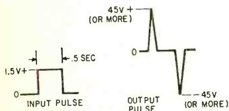
The trailing edge of the input pulse also induces a stepped-up peak voltage in the transformer secondary. This voltage raises the potential of point C and passes through NE2, raising the potential of point D. Simultaneously, point B drops in potential. When the potential difference between points D and B
