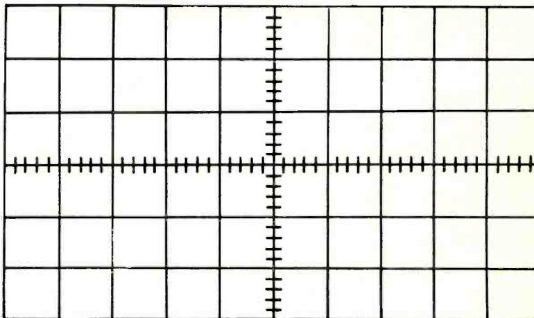
Fig. 1—Layout of a typical graduated grid for your scope. Use tape or es-cutchon to hold it in place. Divisions can be 10 to the inch for convenience.
