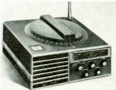
rite core loop antenna. 4 x 6 in. front-mounted speaker. Null meter, beat-frequency oscillator for coded signals. 10½ x 12½ x 4½ in., 10½ lb.—Pearce-Simpson, Inc.
