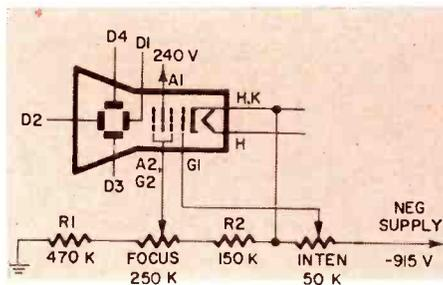
Fig. 1—How to lower focusing voltage when you change CRT type.
