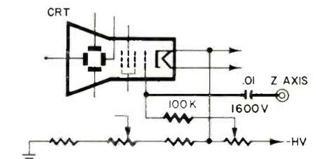
Fig. 6—How to add a Z-axis-modulation terminal to your scope.
