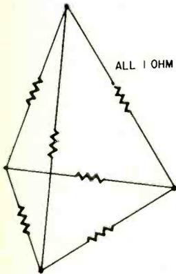
A tetrahedron (pyramid with a triangular base) is constructed, using 1-ohm resistors for the sides. What is the resistance between any two corners?—*Jack L. Shagena, Jr.*
