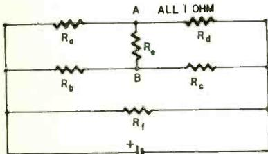
Removing  $R_e$  and solving for  $R_a$  plus  $R_d$  in parallel with  $R_b$  plus  $R_c$ , we get 1 ohm. This in turn is paralleled with  $R_r$ , yielding a result of  $\frac{1}{2}$  ohm across  $R_r$ . This  $\frac{1}{2}$  ohm is the value measured across any one of the resistors in the network.
