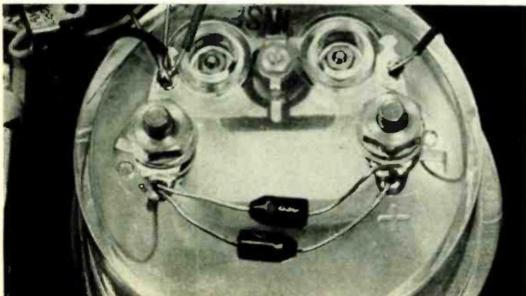
Connect diodes in parallel back-to-back right at the meter terminals.
