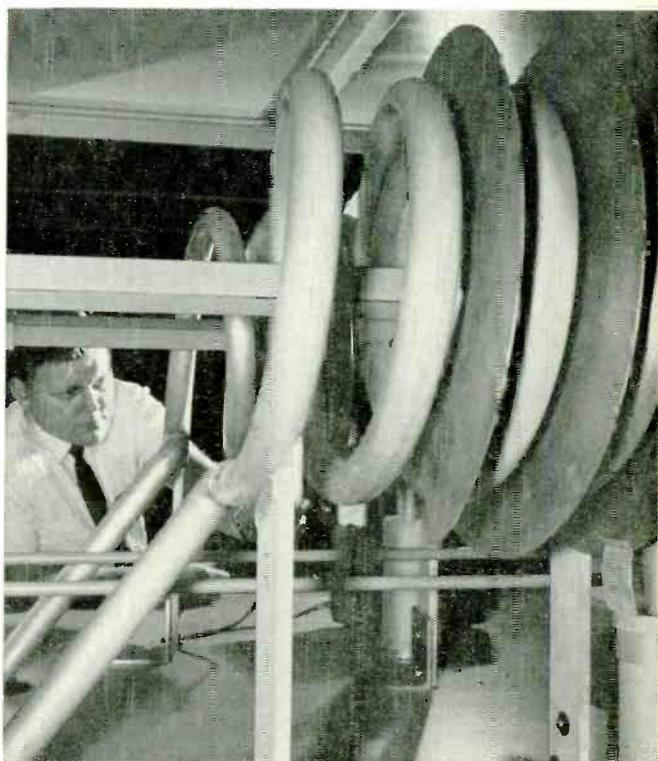
**MASSIVE FINAL COILS** are part of new Hughes-designed 250,000-watt AM short-wave transmitter for Voice of America service to Southeast Asia. To be located in Philippines, transmitter is tunable to any of 20 preset frequencies between 3.95 and 26.5 mc. Maximum tuning time is 20 seconds.
