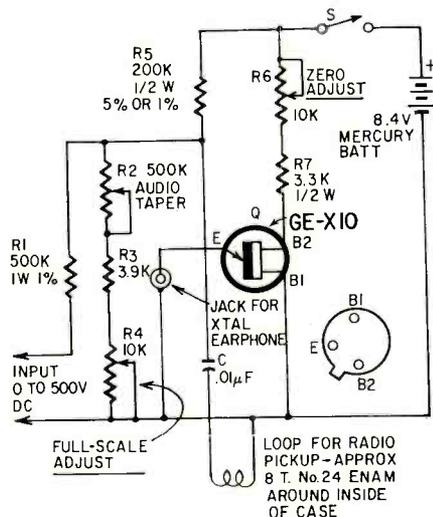
Meterless Meter works on simplified potentiometer principle.
