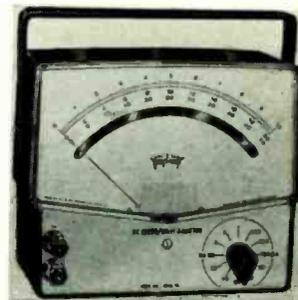
**DC PORTABLE INSTRUMENTS model 825,** feature Bar-Ring suspension movement, 6.84-in. mirror scale, knife-edge pointer, open meter front with top and side natural lighting. Accuracy ± 0.5% in horizontal position. 3 units available: dc voltmeter, dc milliammeter, dc micromilliammeter. 7½ x 6¼ x 3¼ in., with carrying handle.—Triplet Electrical Instrument Co.
