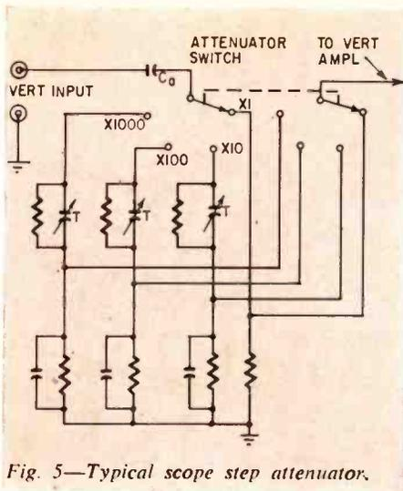
Fig. 5—Typical scope step attenuator.
