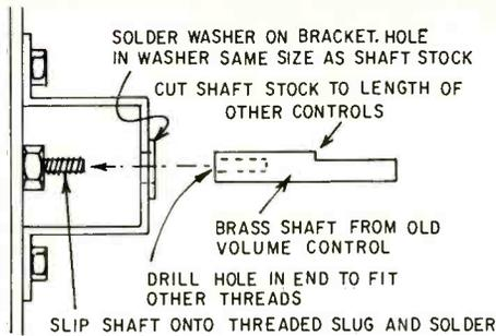
screw and solder it in place. A small bracket was used to hold the large knob in place. Use this bracket but solder a metal washer over the larger hole; choose one that the shaft will twist snugly into. Push a new brown knob over the shaft to match.—Homer L. Davidson
