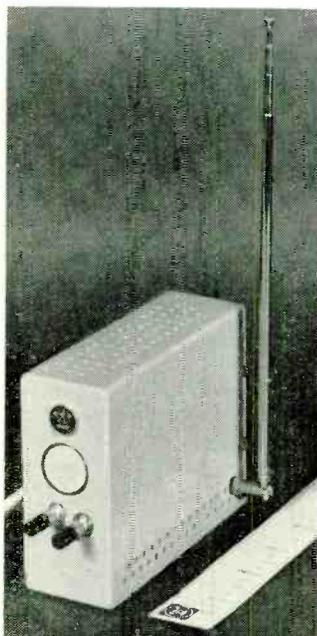
**POCKET-SIZE TV**— $3\frac{1}{2}$  in. high,  $1\frac{1}{2}$  in. wide,  $4\frac{1}{2}$  in. deep! Picture appears on 1-in. electrostatic CRT. Design is conventional intercarrier, fixed-tuned to ch 11, but all circuits except video amplifier and sweep use integrated circuitry. SCR's are used for vertical and horizontal sweep. A 20-kc inverter develops high voltage. Set is powered by rechargeable batteries. Designed by Westinghouse Defense & Space Center, tiny TV is not for sale.
