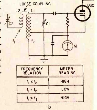
ance headphones. Switch on the dm and couple it loosely to the signal source. Determine the unknown frequency by tuning the dm to zero beat—as heard in the headphones—and reading the frequency from the dm dial. This method works best with an unmodulated signal from the hot circuit. See *Pointers 1, 2 and 3*.
