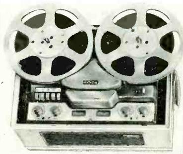
Pabst motors, solenoid-operated brakes, built-in mixing facilities, separate stereo record and play amplifiers, 2 VU meters, 3 ring-core heads, automatic end-of-tape
