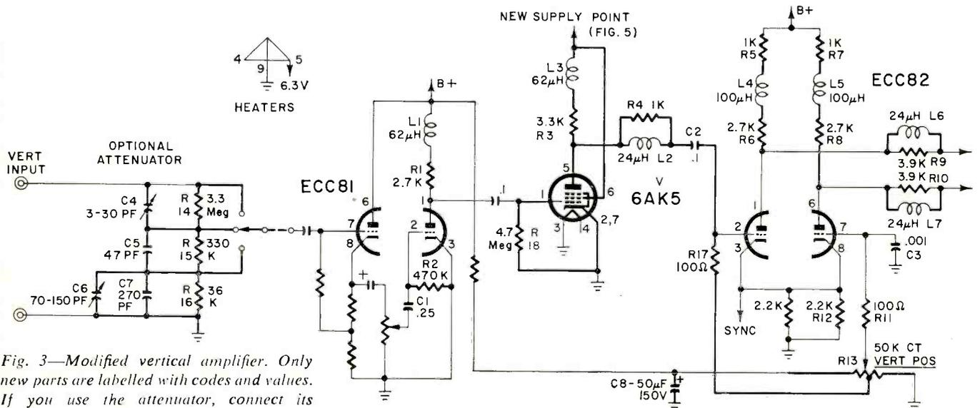
Fig. 3—Modified vertical amplifier. Only new parts are labelled with codes and values. If you use the attenuator, connect its ground to the same point as the first-stage grounded cathode resistor.
