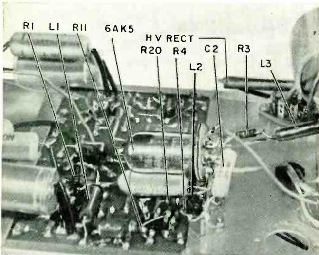
How 6AK5 socket is mounted under chassis on terminal strip right next to pc board. This keeps leads short.
