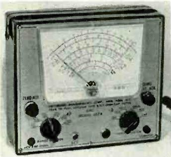
The 107A uses three test leads. DC readings are taken with a separate, shielded cable with a 1-megohm isolation resistor at the tip to minimize capacitance loading in high-frequency circuits.
