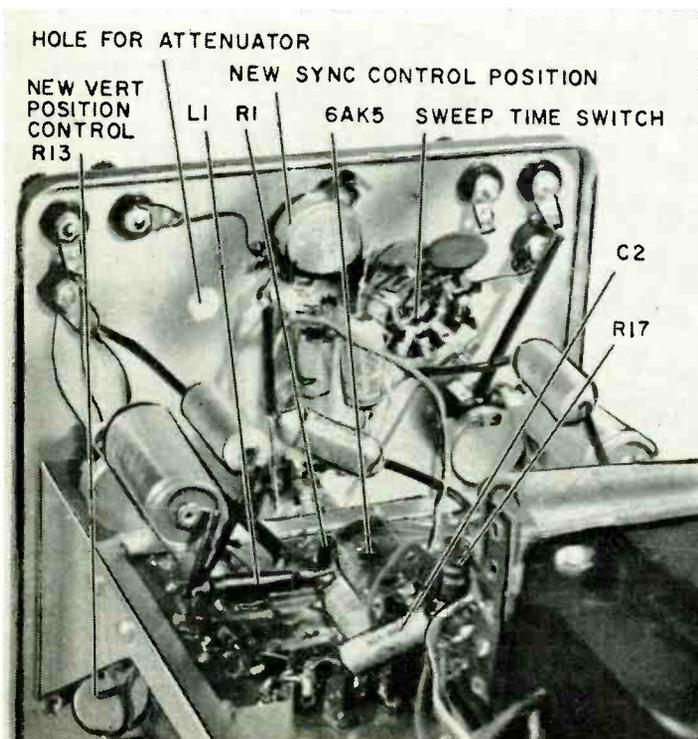
Rear view of front panel shows new location of sync control. Control was moved without disconnecting any wires. Plenty of space if you use a miniature switch for the attenuator.
