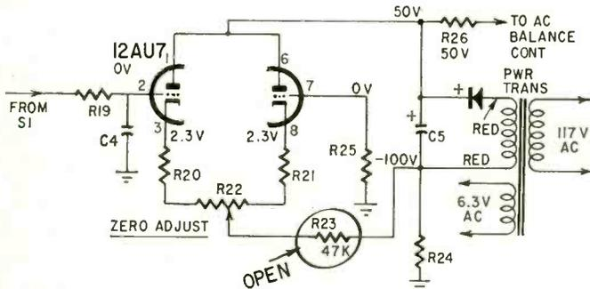
On an Eico 232 vtvm in our shop, the zero-adjust pot stopped working. We checked all tube-element and power-supply voltages, and eventually found that the 12AU7 cathode voltages were wrong. Checking resistors, we found R23, a 47,000-ohm resistor, was open. Replacing it cured the trouble.—*Pierre Cappaert*
