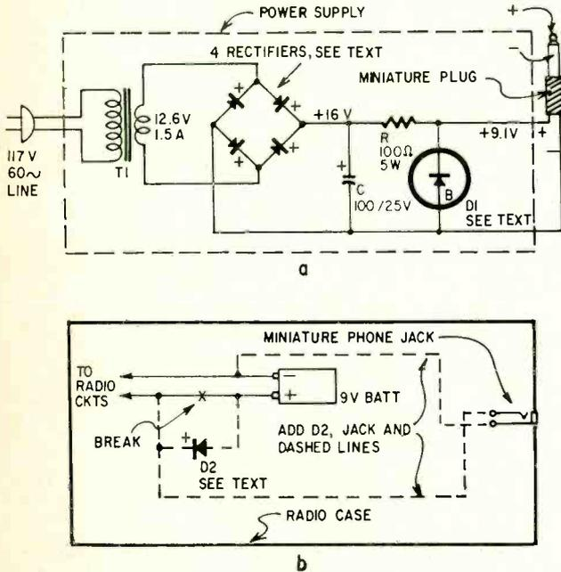
Fig. 1—This simple battery eliminator will pay for itself in less than a year, if you use your transistor portable around the house as often as most people do. With suitable changes in voltages, it'll work with any battery radio.
