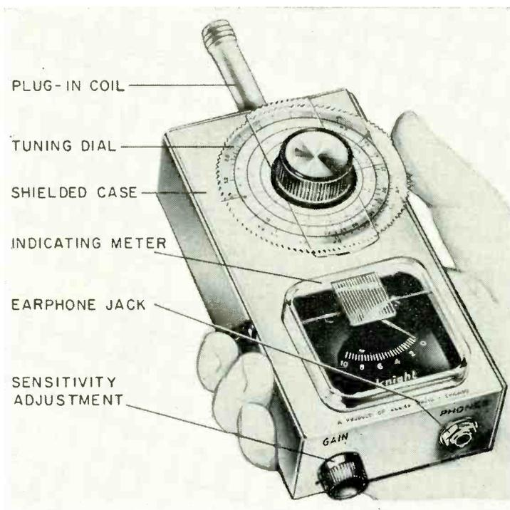
Fig. 1—Typical modern dip meter.
