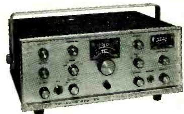
**New Model 753** — The one and only SSB/AM/CW Tri-Band Transceiver Kit. 200 watts PEP on 80, 40 and 20 meters. Receiver offset tuning, built-in VOX, high level dynamic ALC. Unequalled performance, features and appearance. Sationally priced at **\$179.95 kit, \$299.95 wired.**
