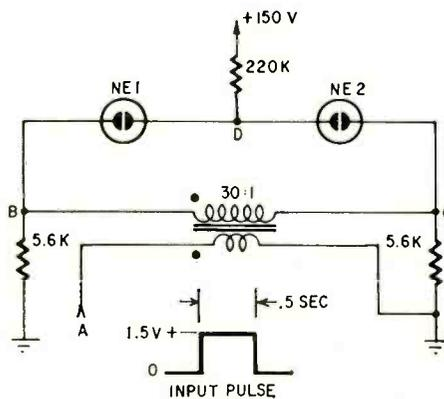
If a positive input pulse of 1.5-volt amplitude is applied to terminal A, which lamp will flop into steady conduction? Assume that, for each lamp, the extinguishing voltage equals the maintaining voltage.—*Kendall Collins*
