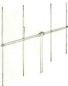
**BASE-STATION ANTENNA FOR CB**, the A-11-S from Mosley Electronics. Gain 8.7 db over ¼-wave dipole or 11.2 db compared to isotropic source. Front-to-back ratio 20 db. Wind load 80 mph EIA standard. VSWR of 1.5/1 or better over 27-mc Citizens band.—Mosley Electronics Co.
