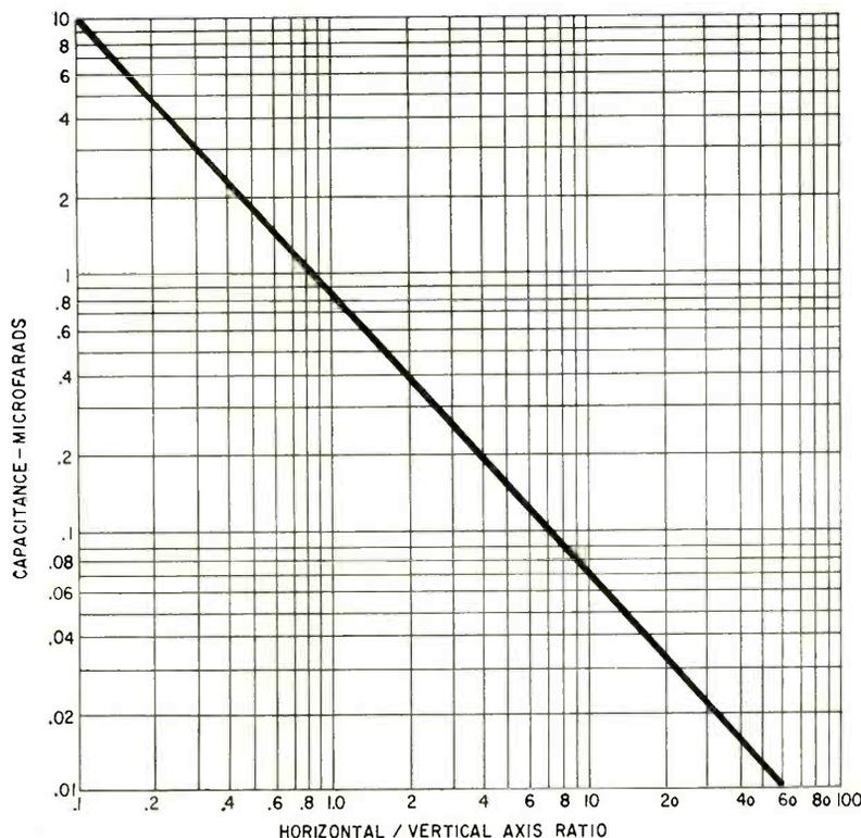
Fig. 6—Size of scope ellipse's horizontal axis, divided by size of vertical axis, is proportional to capacitance.
