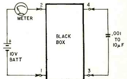
connected to a 10-volt dc supply with an ammeter (or milliammeter) in series.
