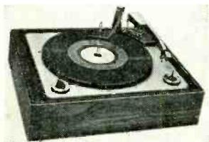
**4-SPEED AUTOMATIC RECORD CHANGER, model AC-33,** has heavy-duty 4-pole motor, heavy 11-in. balanced turntable. Intermixes up to twelve 10- and 12-in. records of same speed, stacks fourteen 7-in. discs. Ribbed rubber turntable mat. Aluminum tone arm with
