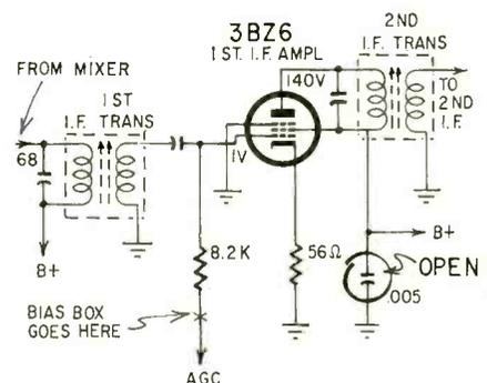
Connecting the bias box relieved all the symptoms of age trouble. But there was nothing wrong with the age! An open screen bypass caused an i.f. stage to oscillate after a few minutes; biasing the tube with the box killed the oscillation.
