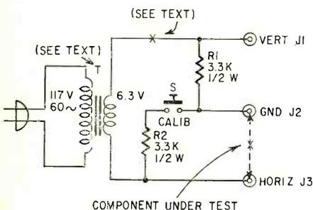
Fig. 1—Circuit of the Component Curve Tracer.
