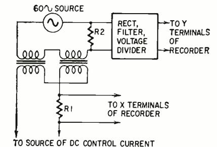
Fig. 6—X-Y recorder being used to plot characteristics of a magnetic amplifier.
