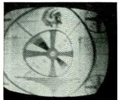
Fig. 4—Here the horizontal linearity is slightly off. Current is normal, but picture is poor.
