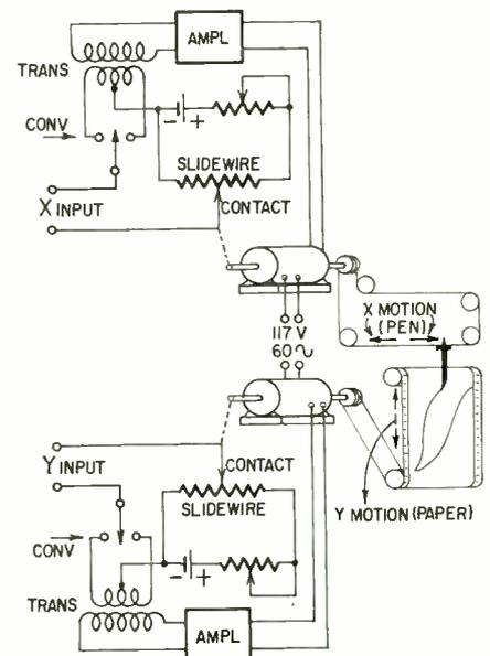
Fig. 3—Simplified functional diagram of an X-Y recorder.
