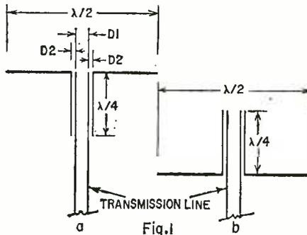
Fig. 1 shows two methods of applying an automatic impedance-matching system to an antenna. They are covered by Patent No. 2,769,169 and were developed to match almost any balanced line to antennas having high or very low radiation resistances. The system is suitable for feeding rhombics, V-beams, folded dipoles, all-channel TV antennas, stacked arrays and many other types of antennas requiring two-wire feed lines.
