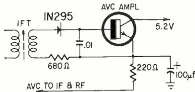
tor, it turned out, was leaky. Since the circuit is a high-resistance one, the small collector-to-base leakage had a serious effect. Replacing the transistor with a low-leakage n-p-n unit restored normal operation.—Richard Rufer
