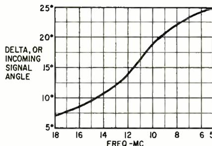
Fig. 1—Incoming vertical angle of arrival of trans-Atlantic radio signals as received on the US East Coast.
