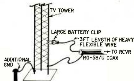
Fig. 7—Hookup for using TV tower as antenna for distance reception.
