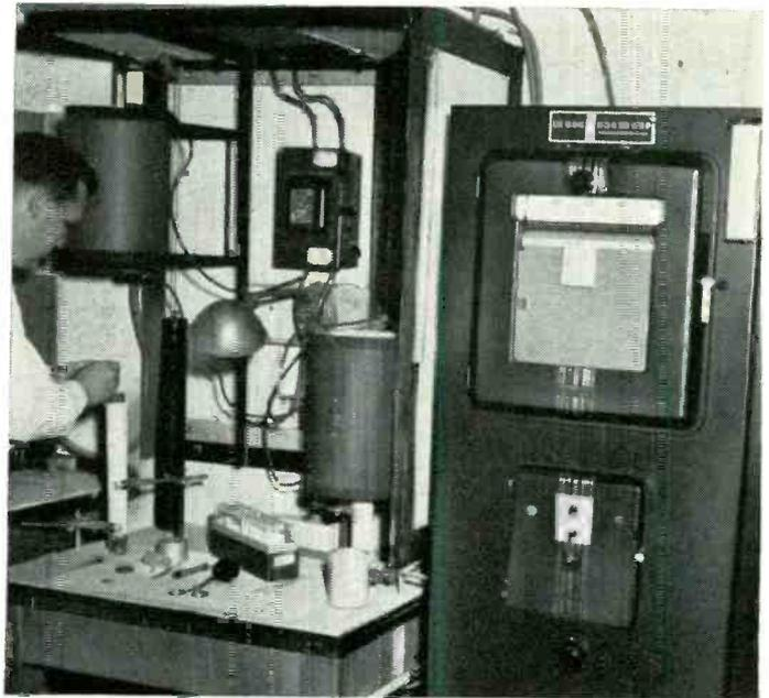
The Leeds and Northrup 69950 Speedomax (above) and (right) with its front cover open and chart assembly removed.
