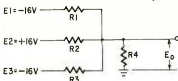
ages to the circuit, and are measured with respect to ground. What is the output voltage,  $E_o$ ?—Earl H. Rogers
