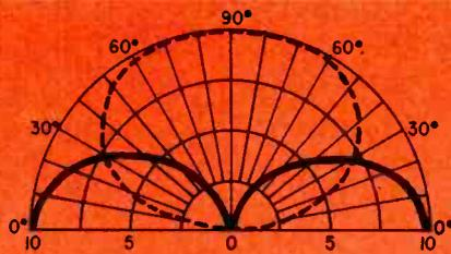
Fig. 4—The balloonlike dashed curve represents the performance of a conventional dipole. The solid curve shows the low-angular performance of the vertical of Fig. 3
