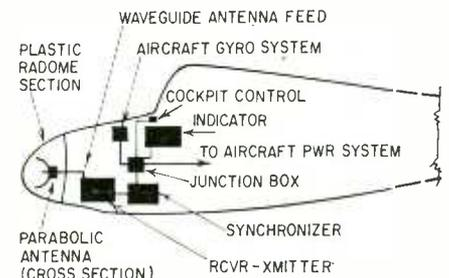
Fig. 3—Typical arrangement for mounting weather radar components in a plane. (Relative sizes of components are exaggerated for clarity.)
