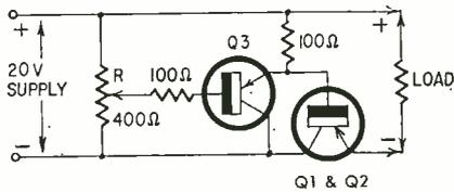
Fig. 4—Adding amplifier stage improves control.
