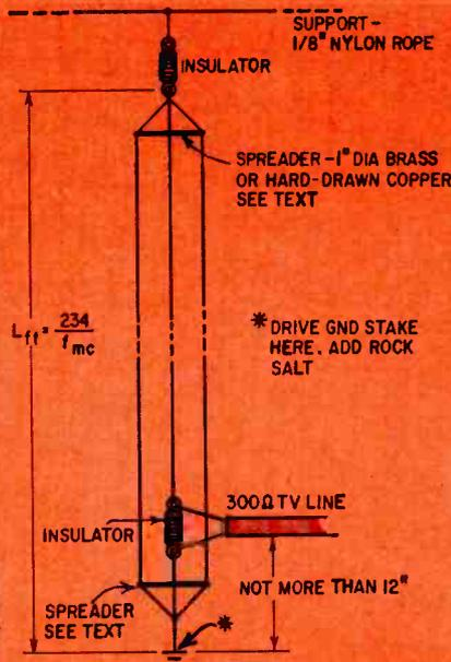
Fig. 3—This three-wire vertical has exceptional distance response.
