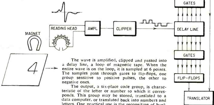
The wave is amplified, clipped and passed into a delay line, a loop of magnetic tape. When the entire wave is on the loop, it is sampled at 6 points. The samples pass through gates to flip-flops, one group sensitive to positive pulses, the other to negative ones.
