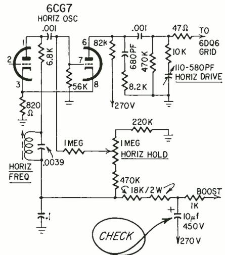
Fig. 7—Olympic GAU chassis horizontal oscillator. Bad boost filter can cause horizontal bending.
