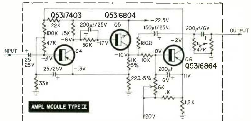
Fig. 1—One of the universal modules. This is a type II. Type III has a 200- $\mu$ f input capacitor. Type I omits the 200- $\mu$ f output capacitor and combines the two 47,000-ohm resistors into one 22,000-ohm unit.
