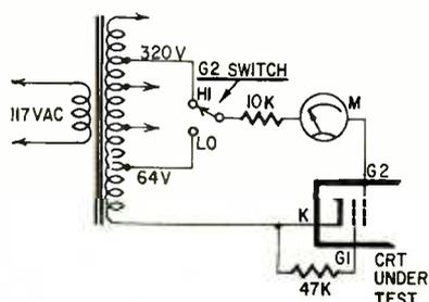
Fig. 4—Emission-test circuit of CRT tester.
