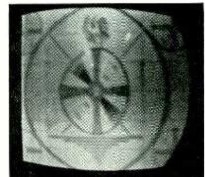
Fig. 3—What happens when drive is too high: current up, width bad, linearity poor.
