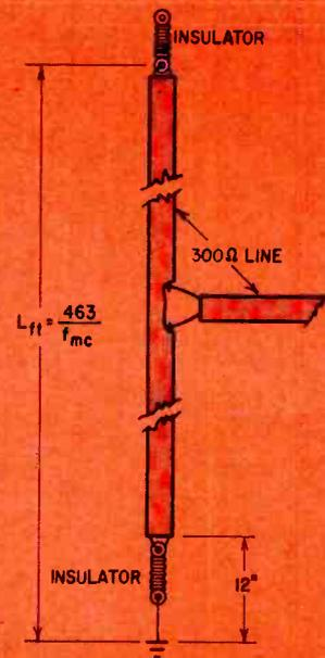
Fig. 5—Folded vertical dipole also has broad-band characteristics.
