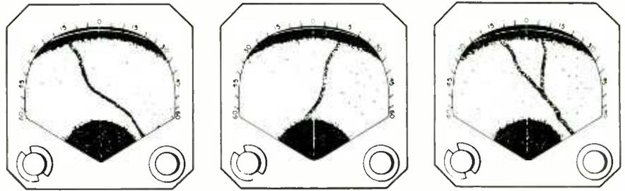
Fig. 4—Relationship between terrain below aircraft, and display, when radar is used for ground observation. (Left), "actual" river, with position of aircraft and scanned sectors. (Above), how scene appears on indicator screen.
