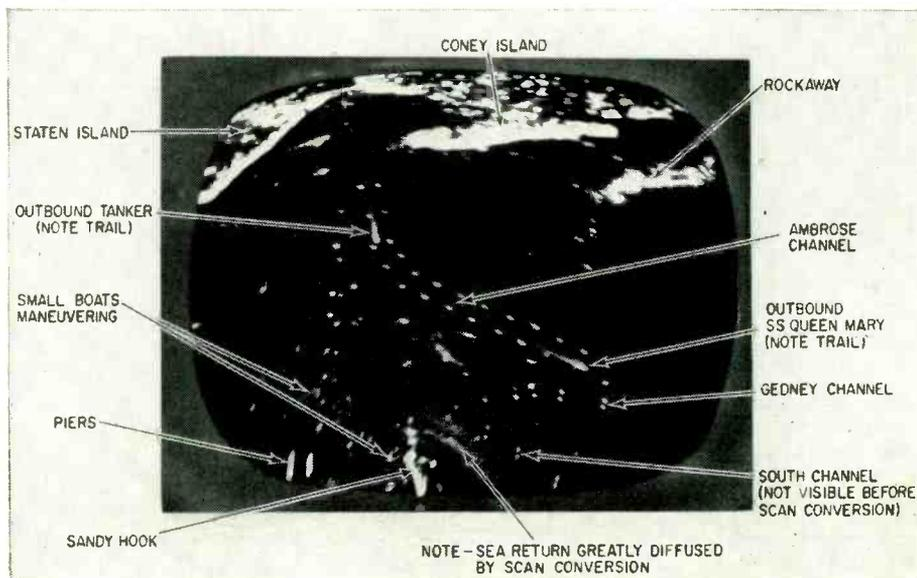
Part of New York Harbor, as seen on RATAN. Rows of double dots are channel buoys. Tadpole-like objects are moving ships.
