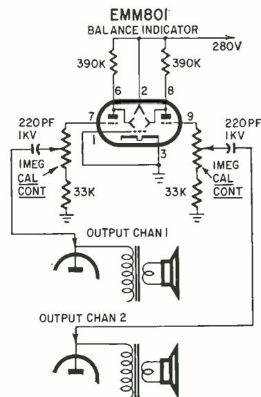
The two calibrating pots must be adjusted when the indicator is first installed. Switch the amplifier to monaural and feed in a tone from a test record or audio generator. Use a vtvm or output meter to measure the signal voltage at the output plates or across the output transformers' secondaries. Adjust the volume controls for equal signals in both channels at normal listening levels. Set the calibrating pots in the indicator grid circuits so both beams are the same length.
