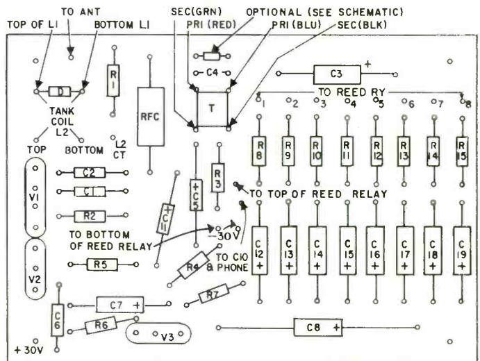
Fig. 2—The receiver circuit board reproduced exactly full size (top left). Parts are mounted on top of the board as shown (above). Receiver and relay boards mount together to form the complete receiver.
