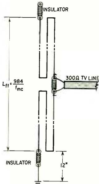
Fig. 6—An added step in distance gain—two half-waves in phase. The upper and lower halves fire together.
