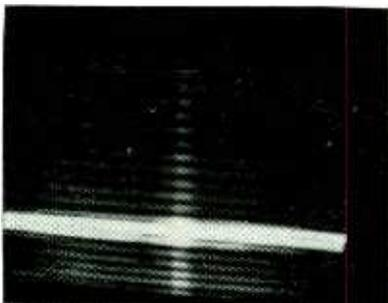
Fig. 6—Horizontal oscillator way off frequency. Amplifier is out of resonance, and current soars.
