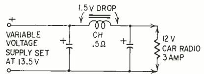
Fig. 2—Basic pi-net choke-and-capacitor filter illustrates regulation problem.
