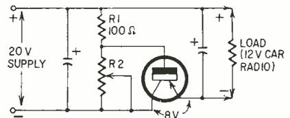
Fig. 3—Using transistor as series control element.
