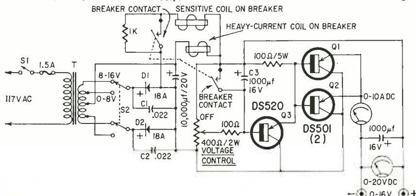
Fig. 1—Complete circuit of the regulated supply. It provides up to 5-8 amps continuous on the high- and low-voltage ranges, respectively.
