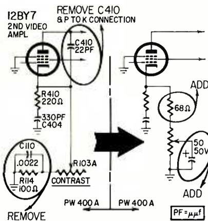
Fig. 2—Modification to reduce blooming in CTC-5 chassis.
