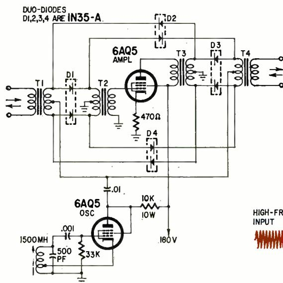
Fig. 1—Diode-switched bilateral amplifier is ideal telephone repeater amplifier. Oscillator frequency should be about 10 to 30 kc. B-supply must be well filtered.
