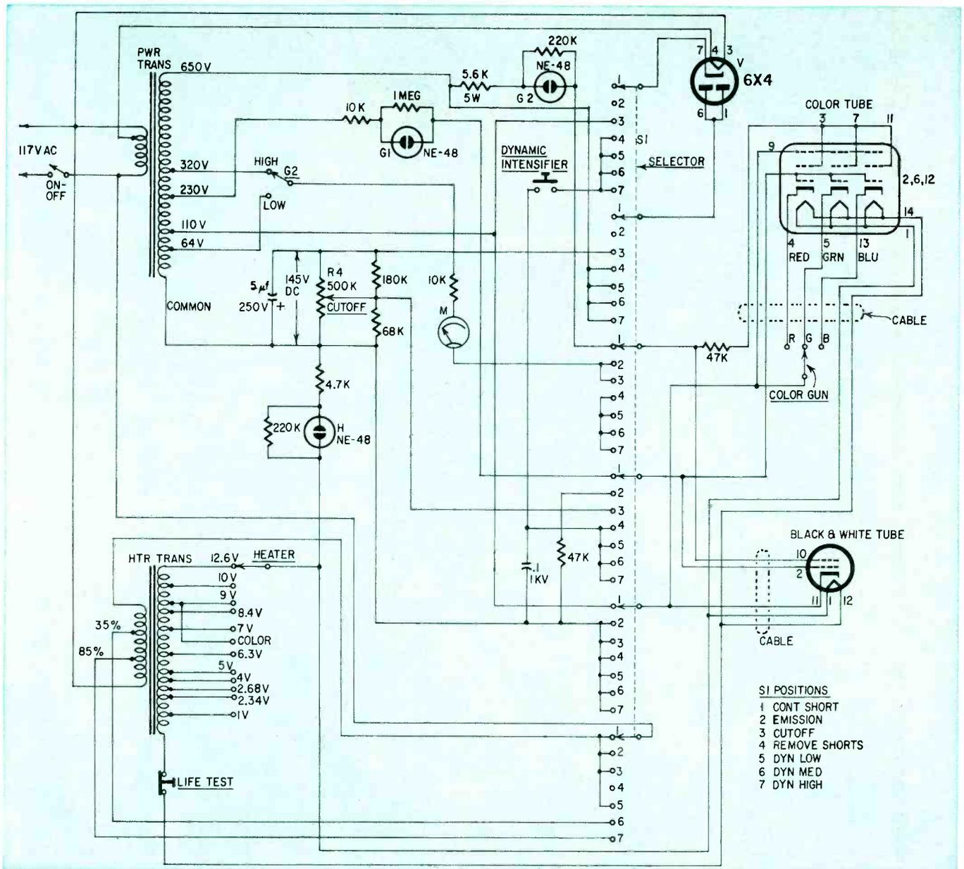
Fig. 2—Schematic of a CRT checker-rejuvenator (B & K model 440).
