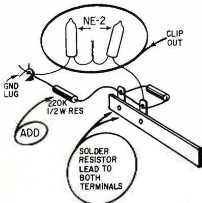
Fig. 3—Neon-lamp modification in CTC-10 and CTC-11 models.
