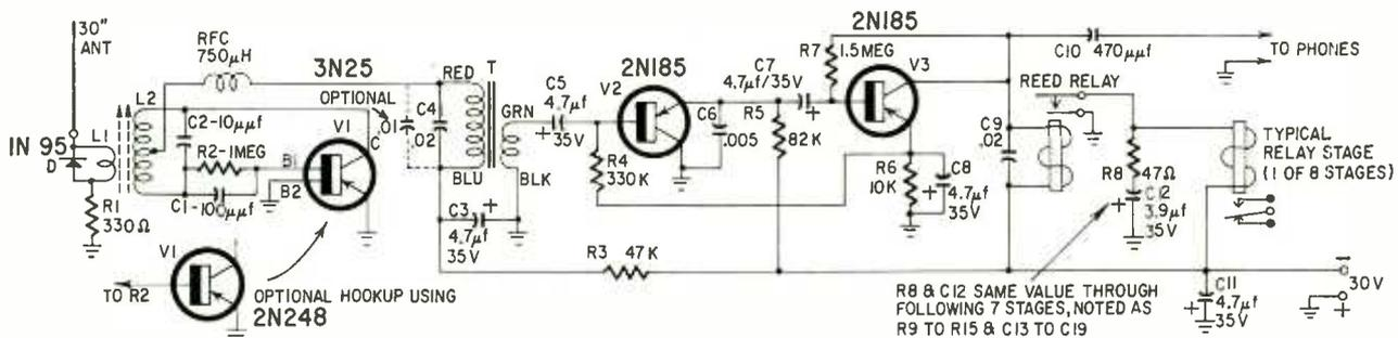
Fig. 1—Circuit of the 3-transistor receiver. Each reed of the reed relay operates at a different frequency and triggers a different control circuit.
