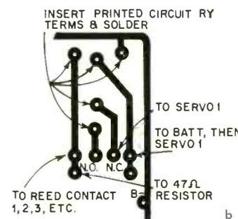
Fig. 3—The relay circuit board (a). Terminals on control relays go through board and are soldered to printed wiring on underside. Connections to relay 1 are shown (b). Other relay circuits are identical.
