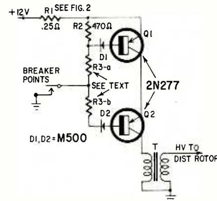
Fig. 4—Circuit of Fig. 2 revised for Mallory F-12-T coil. Except for adjustment of R3, values are same as Fig. 2.
