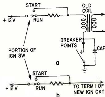
Fig. 3—How to connect the new system: (a) shows former circuit, (b) new one. Start-run feature is found in some GM cars.
