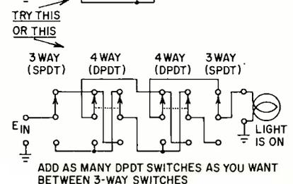
make a good puzzle (May EQ, page 34), in real life two three-way (spdt) switches and one four-way switch would be used, as shown in the sketch.
