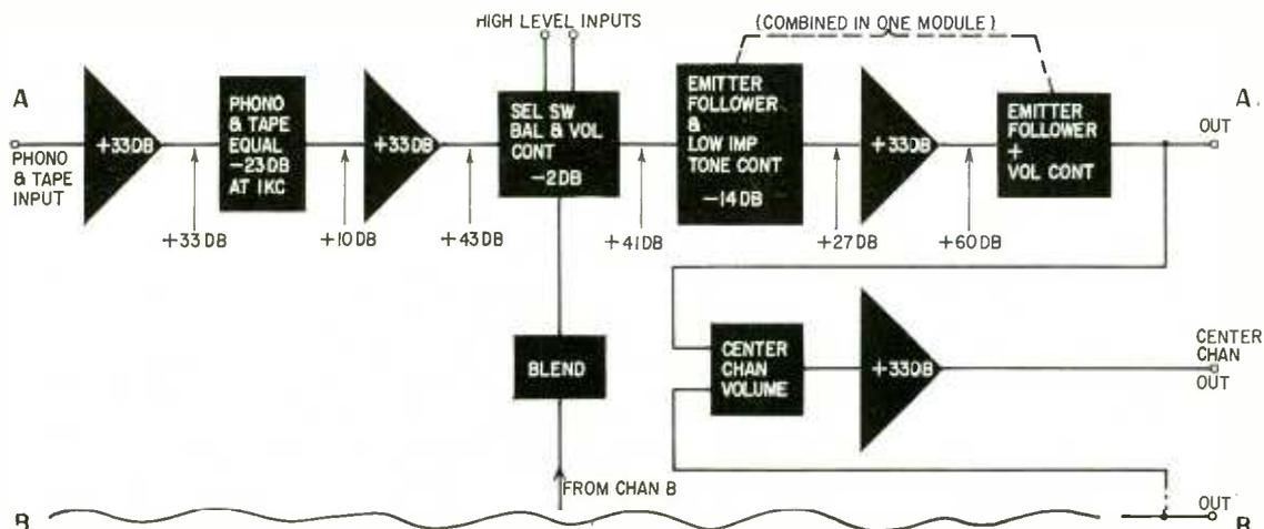
Fig. 2.—Line diagram of the Citation A control unit. Triangles are amplifiers; circuitry in the blocks adds no gain.
