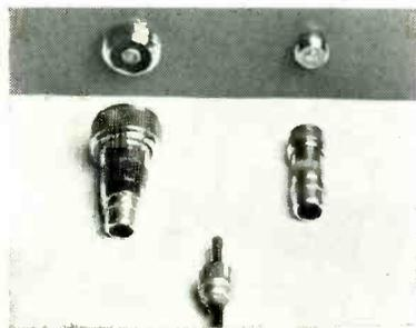
then clip off the extra wire and solder the wire into the mike connector's eyelet in the usual manner. Make the miniature adapter the same way, but file off a little of the threads on the remaining pin jack to allow it to slip into the end of the miniature mike connector.
