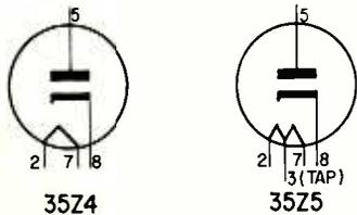
Fig. 8—Base diagrams of the 35Z4 and 35Z5. The only difference is the heater tap.
