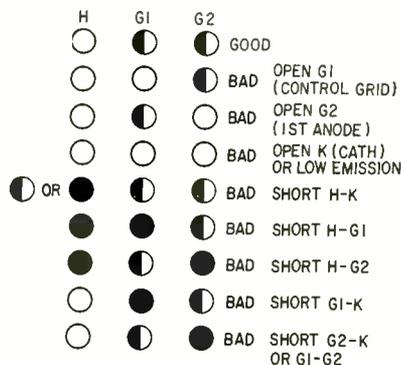
Fig. 3—Neon-lamp indications on B & K tester. Filled-in semicircle denotes lighted electrode.
