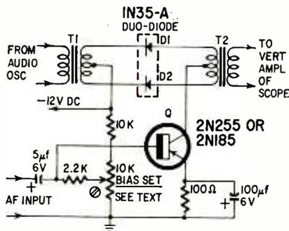
Fig. 3—Simple and practical diode modulator and driver. Circuit may be used in a number of ways. Bias set control is adjusted only once, then locked in place.
