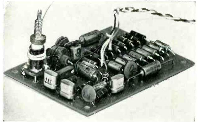
Capacitor C10 is used in series with a pair of headphones for receiver alignment. Tuning is simple. Plug in the phones and tune the tank-coil slug for maximum sound. To determine the best position of the antenna link, substitute a vtvm for the phones and adjust for maximum reading.
