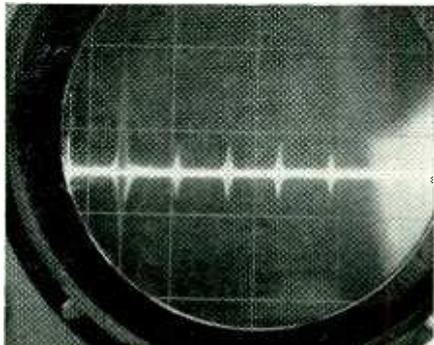
Appearance of markers when variable marker is set at 41.25 mc and 1.5-mc crystal is in use.
