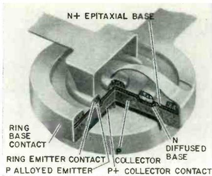
is 0.7  $\mu$ sec at 8 amps collector current. The new transistors offer a choice of three breakdown voltages (hence the three types)—50, 75 and 100. Current gain at 10 amps is 25, minimum, and typical cutoff frequency is 100 kc.
