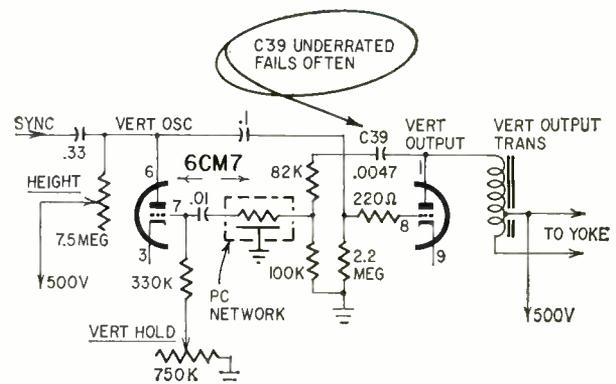
and finally complete loss of height. The original capacitor is rated at 600 volts, which is too low to withstand the high pulse voltages on the output plate. For all replacements I use buffer capacitors rated at 1,600 volts.—*Charles B. Randall*
