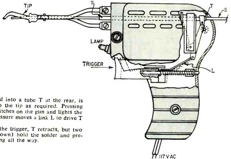
Solder S, loaded into a tube T at the rear, is automatically fed to the tip as required. Pressing the trigger lightly switches on the gun and lights the lamp. Additional pressure moves a link L to drive T forward.
