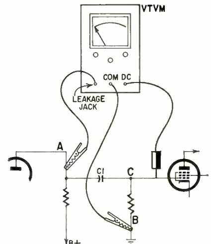
Fig. 2—Typical coupling circuit showing in-circuit leakage connections.
