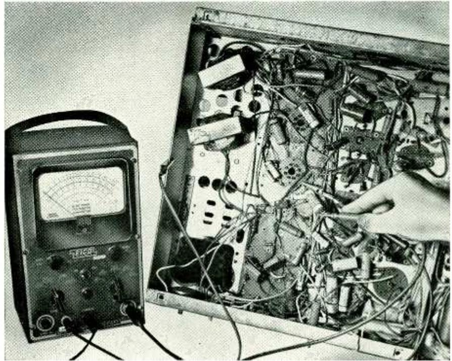
Testing for a leaky capacitor in a TV set. Zero meter reading indicates no leakage.
