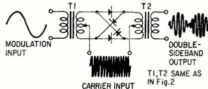
Fig. 4—Basic DSB (double sideband) modulator.
