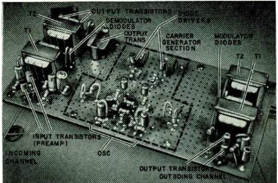
Experimental layout of speech scrambler. Ordinary radio feeds scramble generator amplifier in center of chassis.
