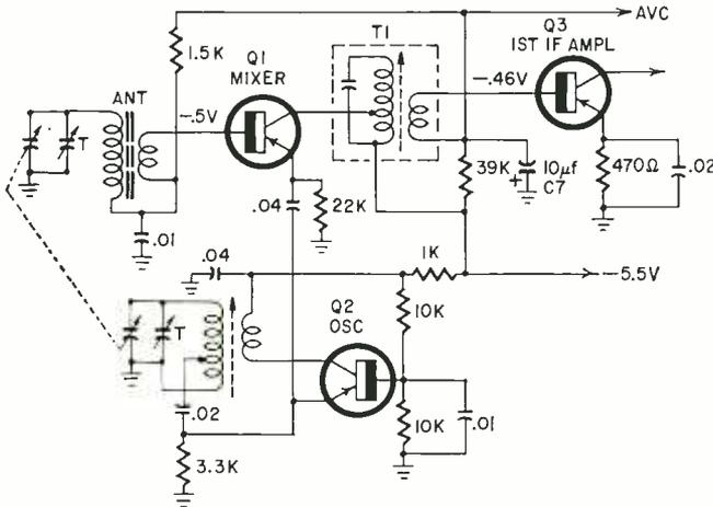
—2.4 volts instead of —0.46. Q3's emitter was also too negative. Q1's base also read —2.4 volts. C7 was good. On a hunch, I measured the resistance between primary and secondary of T1. It was 15,000 ohms instead of something near infinite! A new transformer and a realignment put the set back in shape.—CWO Laddie F. Klancher
