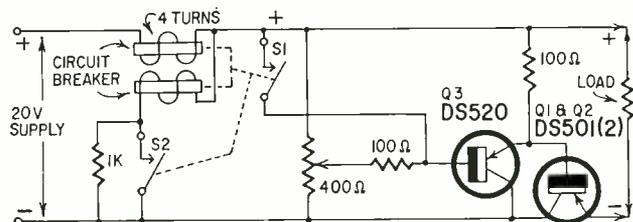
Fig. 6—Details of circuit breaker action.
