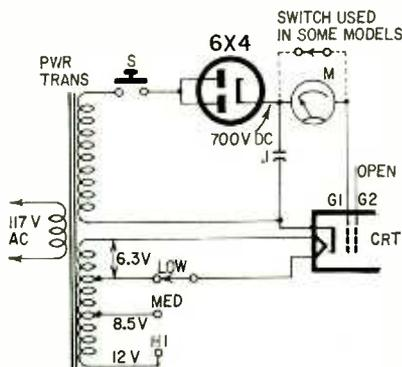
Fig. 5—Typical reactivation circuit. Meter may be in circuit or out, depending on make and model of tester.
