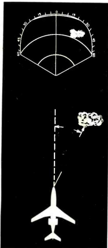
Weather information detected and presented by the weather radar system is based on *rainfall gradient*: the variation of the rate of rainfall with distance. Radar pulses are reflected by precipitation, such as rainfall, wet hail or wet snow. Variations in rainfall gradient are detected by *contouring* (Fig. 2). When the radar is set up for contouring, areas of heavier rainfall appear as *dark spots* on the indicator screen, while the *brighter* display areas indicate lighter rainfall.
