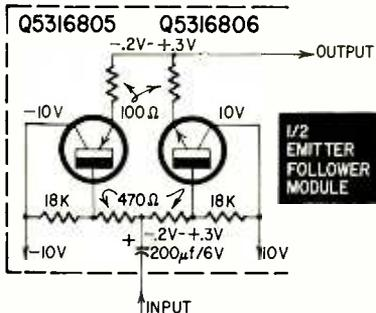
Fig. 3—First emitter follower. The second emitter follower has a 200- $\mu$ f capacitor in the output lead.
