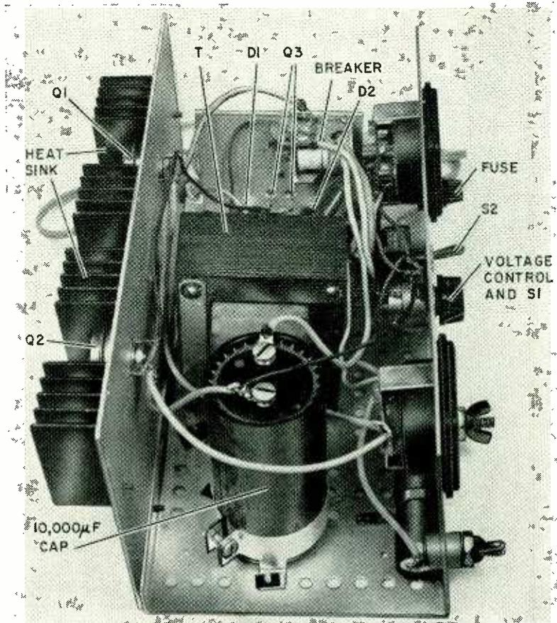
Internal layout and wiring of the P-612.
