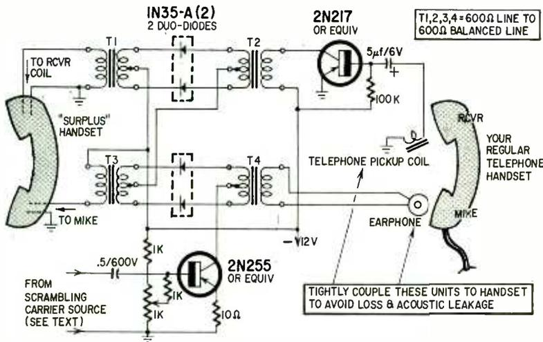
Fig. 6—One end of suggested voice scrambling system uses a diode modulator and random-scrambled carrier. Other end exact duplicate.
