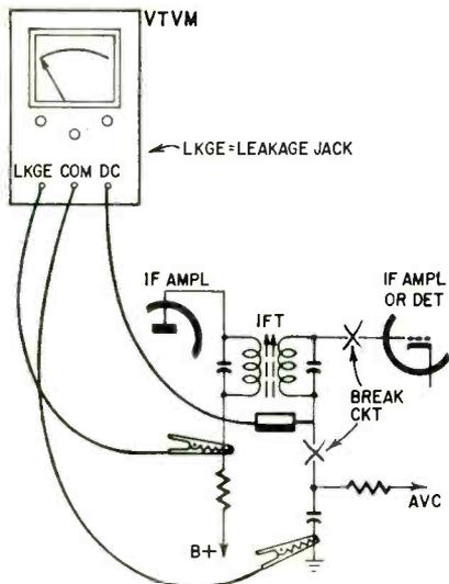
Fig. 3—Checking for leakage in a radio i.f. transformer.
