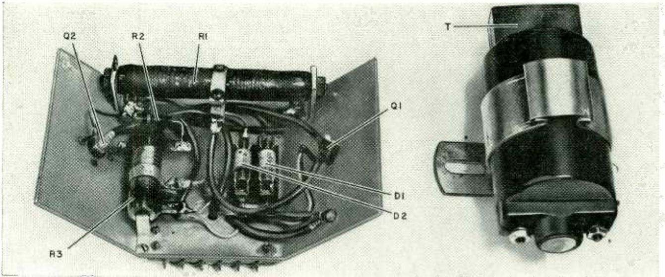
Underside of chassis. As shown here, unit has been modified (per Fig. 4) for Mallory F-12-T coil, at right.
