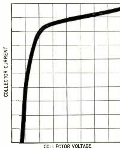
Fig. 2—How current vs voltage curve for a transistor might look.
