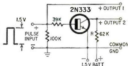
arrangement, which also gives best economy and reliability. It requires only three ½-watt resistors, one transistor and one penlight cell.
