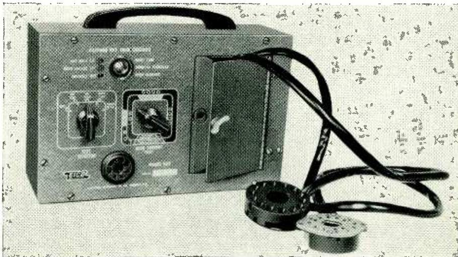
The Eico model 630 (wired) and 630-K (kit) CRT checker.
