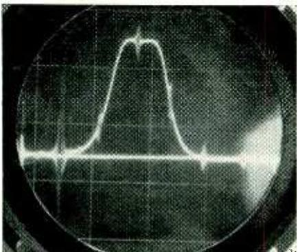
Markers as they appear on narrow-band TV if curve. Large marker is 41.25 mc, frequency at which marker oscillator dial is set. All important points of if curve are marked simultaneously.
