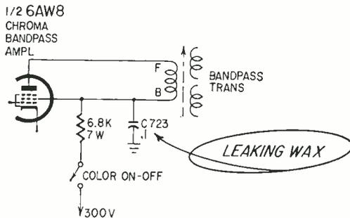
leaking wax and measured 750,000 ohms. M. L. Tortariello
