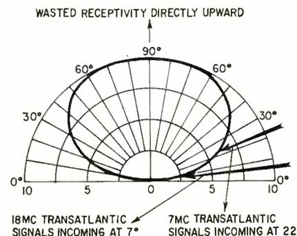
Fig. 2—Record of poor performance of a horizontal dipole one-quarter wavelength up. Note how receptivity is concentrated directly upward and is largely wasted for distance reception arriving at much lower angles.
