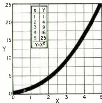
Fig. 1—Y is the dependent variable as its value depends on the value of X. X, the independent variable, can have any desired value.
