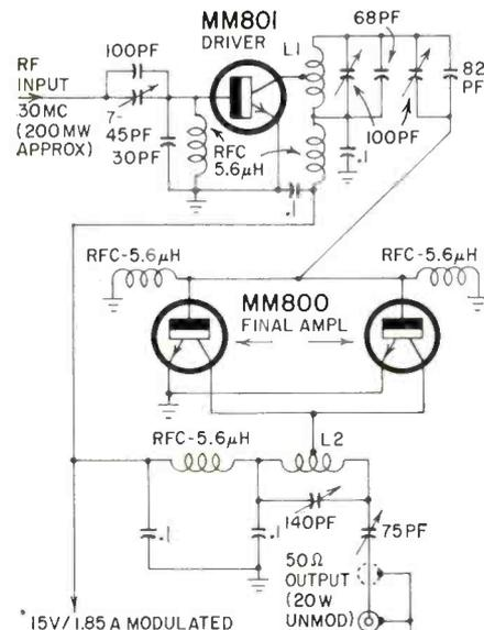
C amplifiers. All are n-p-n. Of the last two, the MM800 has the higher ratings. It is guaranteed to produce 15 watts unmodulated rf output at 50 mc with a collector voltage of 25 and a driving power of 3 watts. It functions at junc-
