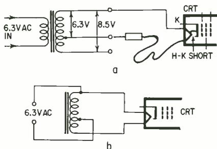
Fig. 6—(a) Transformer type brightener; used to boost heater voltage or isolate heater-cathode short. (b) Autotransformer type brightener; boosts heater voltage but does not provide isolation.
