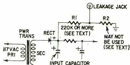
Fig. 1—Adding resistors R1, R2 and a banana jack to the vtvm power supply are the only modifications necessary.
