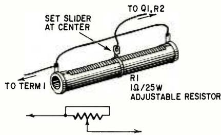
Fig. 2—Details of the 0.25-ohm 25-watt resistor. Centered slider makes two 0.5-ohm resistors, which are paralleled to give 0.25-ohm.
