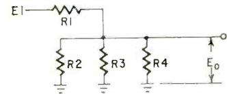
Note that R2, R3, and R4 in parallel equals  $\frac{1}{3}R$ . Therefore  $E_o = \frac{1}{4}$  the input voltage.  $E_o$ , as a result of E1, is -4 volts. When E2 is considered as the input, output 2, as a result of E2, is +4 volts. When E3 is considered as the input, output 3, as a result of E3, is -4 volts. Adding outputs 1, 2 and 3 algebraically, the actual total  $E_o$ , with all three inputs is -4 volts.
