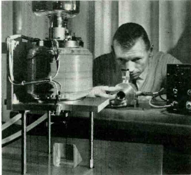
*Robert C. Duncan of RCA Labs adjusts the focus of a solid-state receiver, which detects the information-bearing laser beam generated by the device in the foreground and shot to the detector by the prism.*
