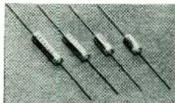
dia. x 1½-in. long case, 500  $\mu$ f at 5 volts, 17  $\mu$ f at 150 volts.—**Sprague Electric Co.**, 125 Marshall St., North Adams, Mass.
