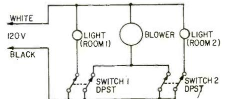
Two double-pole single-throw switches, connected as shown, do the job.
