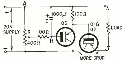
Fig. 5—How ripple is eliminated
