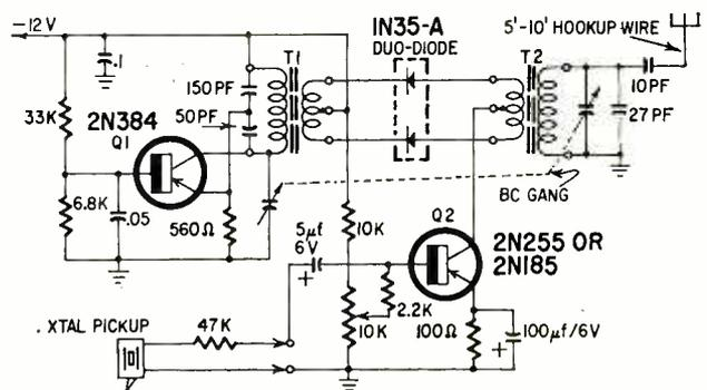
Fig. 5—Balanced diodes modulate wireless phono oscillator. Orient coils T1 and T2 at right angles to each other.
