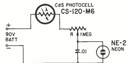
posed to bright light, the resistance drops to less than 1,000 ohms. This resistance change provides a large range of oscillation—so large, in fact, that the additional resistance of potentiometer R has been added to permit slowing the blinking rate to an easily countable figure.
