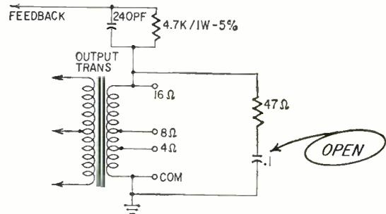
of the output transformer to present a low-impedance load to the amplifier at these damaging high frequencies. The trouble was traced to the 0.1- $\mu$ f capacitor—it was open.—*Barry Atwood*
