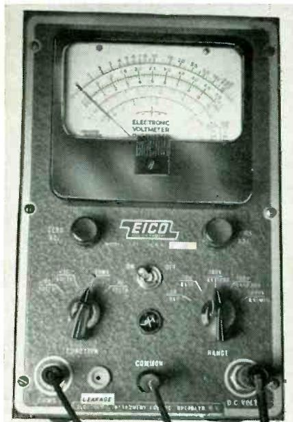
Leakage jack installed on my vtm for testing capacitors in and out of circuit.
