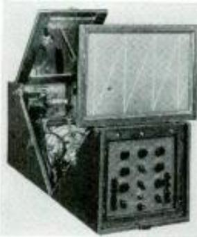
All the usual oscilloscope controls are present. Sensitivity is 60 mv per inch vertically and 0.65 volt per inch horizontally. Vertical amplifier response is good to 50 kc and usable to 100 kc. Horizontal sawtooth sweeps are good to 2 kc and usable to 5 kc.
