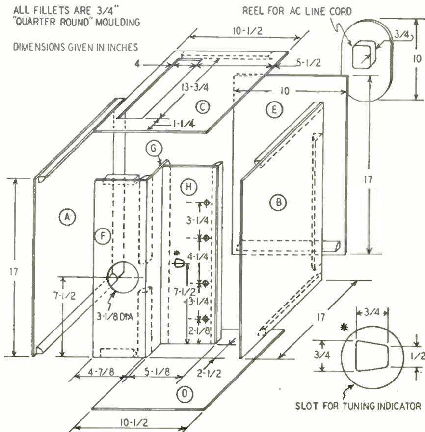
Fig. 2—This completely dimensioned drawing may be used to duplicate case made by author.
