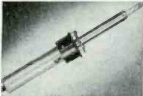
The iron works directly from the 117-volt line, using no transformer either in the tool or independent of it. Weight is under 1/2 pound. In the specimen tested, wire solder was melted in 12 seconds from the time the switch was operated.
