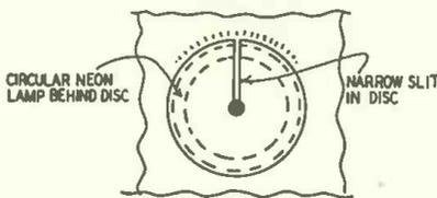
A masking disc rotates in front of the lamp. When the lamp glows, light is observed at one point (through a narrow slit in the disc). The disc and the loop are synchronized, both being operated by synchronous motors.
