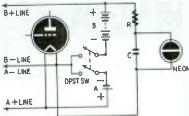
Fig. 3—How blinker is added to the receiver.
