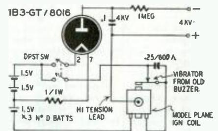
Fig. 1—Miniature high-voltage power supply.
