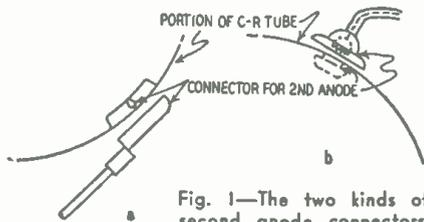
Fig. 1—The two kinds of second anode connectors.
