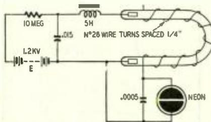
The diagram shows a flasher operated from a high-voltage dry battery. The .015- $\mu$ f capacitor is charged through the high resistance; and when a critical potential is reached, the U-shaped neon lamp flashes. Then static accumulates on its glass envelope.
