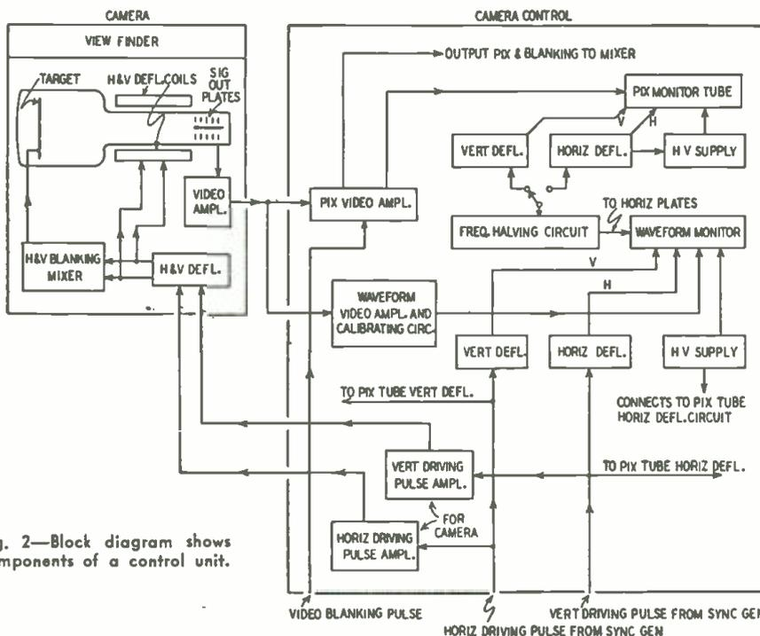
Fig. 2—Block diagram shows components of a control unit.
