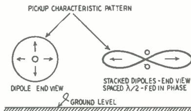
Fig. 2—Fields of single and stacked dipoles.
