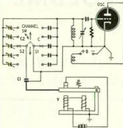
Less series capacitance is used in series with C1 at the upper channels to reduce the relative frequency deviation.
