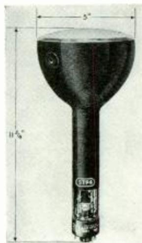
At left is the high-voltage 3NP4 used in Philips projection receivers; center, the Philco TP-400A, another high-voltage projection tube; and above, the RCA 5TP4. In spite of their general similarity, they are not interchangeable.
