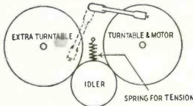
her-rimmed idler wheel will touch both turntables. Mount the idler on a slotted center so a tension spring will hold it firmly against both turntables.
