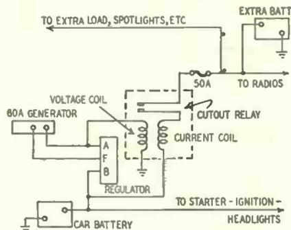
regular battery. A standard 60-ampere generator is adequate for charging both.
