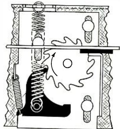
When drum is pressed, white plate moves down, carrying ratchet, which then engages with the next tooth on gear wheel. Upon release, the spring (which is broken in drawing to show the action), draws the plate and ratchet upward, thereby turning wheel one tooth or setting.
