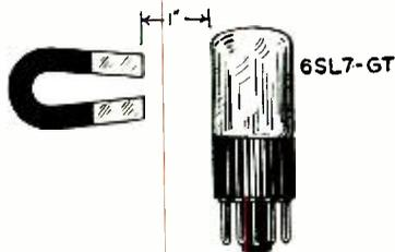
Heater-current hum (an induction effect) can often be cured by placing a small permanent magnet near the tube, but bringing the magnet right up to the tube and then withdrawing it makes the hum become much worse and remain so. After concluding that this was caused by the magnetizing of the tube elements, the three engineers tried demagnetizing tubes in a decreasing a.c. field with a procedure somewhat similar to that used in demagnetizing watches.
