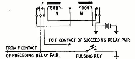
One pair of relays operates with each pulse.
