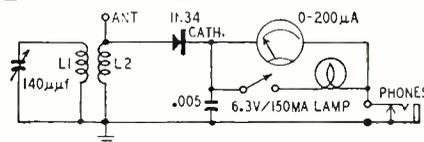
post. The switch places a pilot lamp across the meter so the meter will not burn out with high r.f. input.
