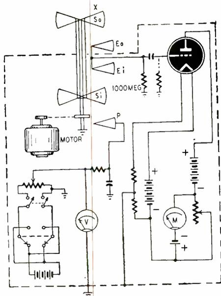
A motor rotates a shaft having two similar shutters or shields S0 and S1. The first is outside the main electrometer shield (dashed box) and the other is inside. Two stationary electrodes E0 and E1 are connected to the control grid of a triode through a capacitor. Another fixed electrode P is connected to a source of d.c. through a potentiometer. Its potential to ground may be adjusted. The voltmeter V measures this potential.
