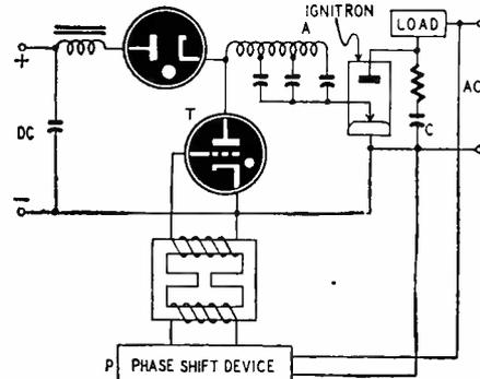
During each alternate half-cycle of a.c., condenser C places a positive potential on both the ignitron anode and the thyatron grid. When the latter exceeds the critical value, the thyatron discharges a momentary square wave of current through the mercury pool of the ignitron. This fires the ignitron through the load.
