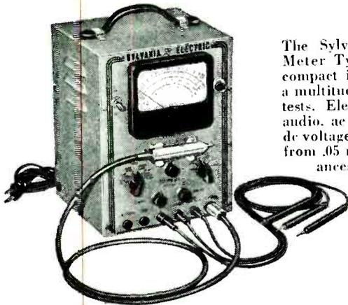
The Sylvania Poly (MULTI-PURPOSE) Meter Type 134Z provides, in a single compact instrument, the means of making a multitude of electrical measurements and tests. Electrical values measured include audio, ac and rf voltages (up to 300 mc); dc voltages from 0.1 to 1,000; direct currents from .05 milliamperes to 10 amperes; resistances from ½ ohm to 1,000 megohms. Instrument is compactly built, attractively styled, includes all essential accessories. Priced at only \$89.50.
