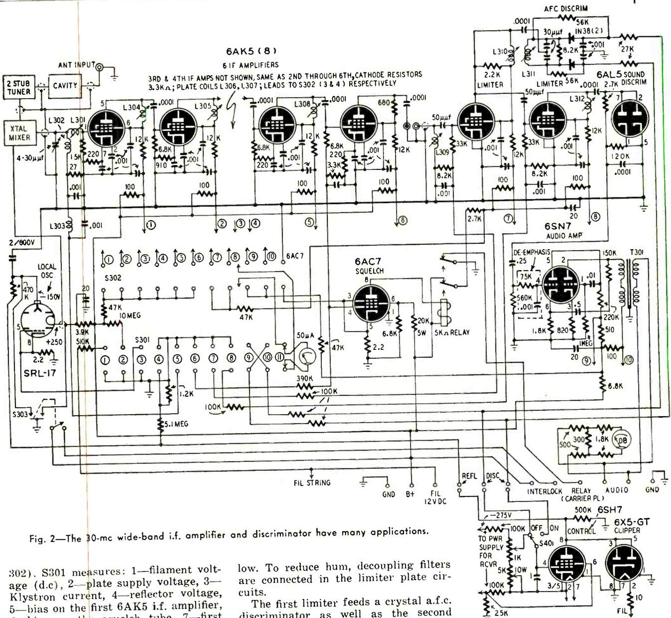
Fig. 2—The 30-mc wide-band i.f. amplifier and discriminator have many applications.
