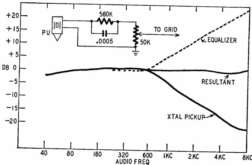
Fig. 1—Typical response curve of a crystal cartridge with and without h.f. equalization.
