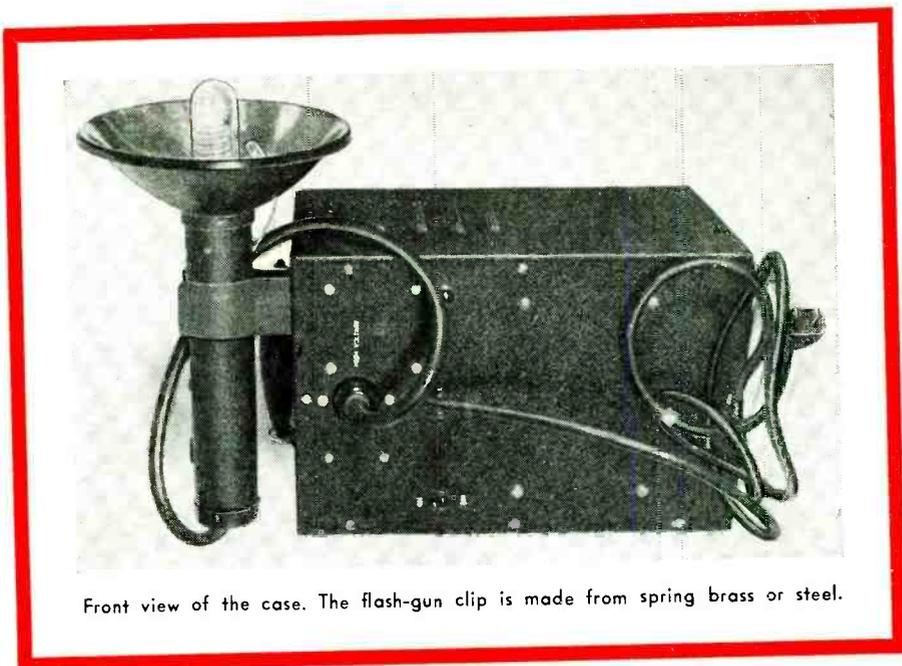
Front view of the case. The flash-gun clip is made from spring brass or steel.
