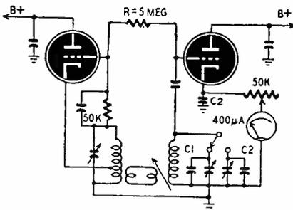
The first tube is an r.f. oscillator which supplies voltage through a link to the second tube which operates as a v.t.v.m. To measure or compare two condensers, for example C1 and C2 as shown, the switch is thrown to C1. The trimmer is adjusted for resonance and the maximum reading is noted on the meter. Now the switch is thrown to connect C2 and its trimmer. As before, the trimmer is resonated and the reading taken. The meter readings are proportional to the circuit Q in each case.
