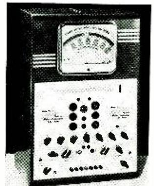
the customer to see the condition of his tube. A mutual-conductance tester, the unit shows transconductance up to 15,000 micromhos. A test is provided for gas and low voltage is available for diodes. The tester measures 26 3/4 x 17 x 11 inches. Flexibility has been provided in the selector switches to take care of unusual tube basing arrangements. Data is given on a roll-type chart.
