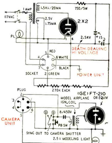
Well-insulated cable connects the two units.
