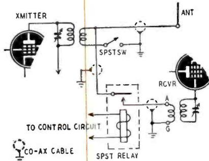
Simply place the relay contacts in series with the lead to the receiver. Wire the control circuits so that operating the transmitter switch opens the relay. (The relay may be normally open or normally closed, depending on the control circuits.) The transmitter is still connected during receiving periods, but the receiver level is not affected.
