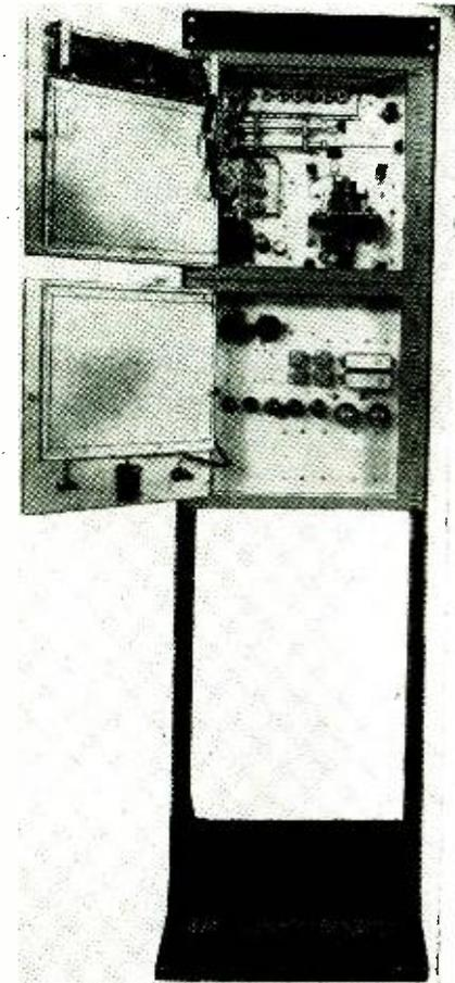
The rack-mounted receiver and power supply.
