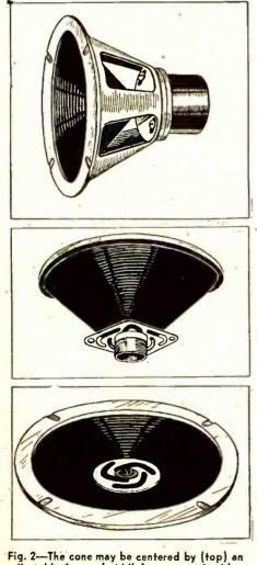
Fig. 2—The cone may be centered by (top) an adjustable frame, (middle) an external spider, or (bottom) a spider centered on the magnet core. Small types may be non-adjustable. By FRED
