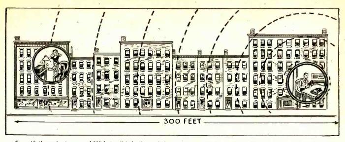
Even with the moderate range of 300 feet, a "wireless" record player may create interference in a radio several doors down the street.
