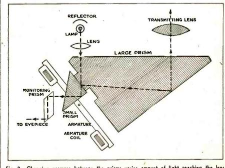
Fig. 2.—Changing pressure between the prisms varies amount of light reaching the lens. RADIO-CRAFT for DECEMBER, 1943
