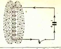
Fig. 3-The simplest type of oscillating circuit.
