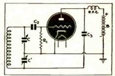
Fig. 9.—The Colpitts circuit, an inside-out Hartley.
