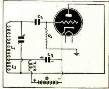
Fig. 6—The Hartley oscillator, a famous circuit.
