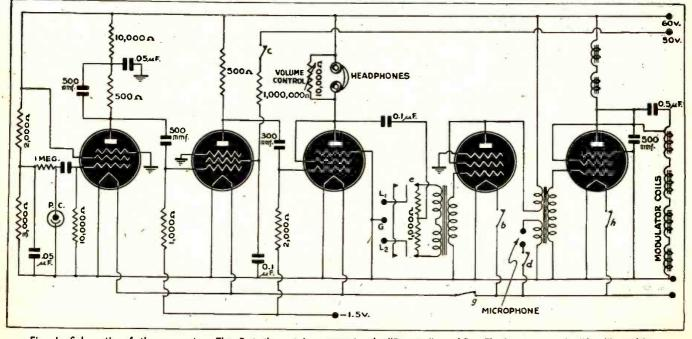
Fig. I-Schematic of the apparatus. The first three tubes comprise the "Receive" amplifier. The last two are the "Send" amplifier. RADIO-CRAFT DECEMBER. for 1943
