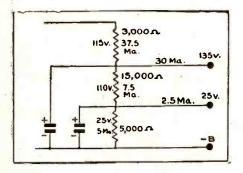
2 R.F. tubes and output pentode take 30 Ma. at 135 volts, we start as shown in the diagram.
