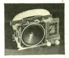
Circuit includes many outstanding fea-tures such as oscillator biased R.F. and tures such as oscillator biased R.P. and I.F. stages, contact-potential biased audio stage, inverse feedback, automatic volume control, high capacity filtering, self-con-tained antenna and others.—*Radio-Craft*.
