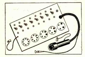
sockets, then a lead from each is run to one of the pin jacks in the inside row, through the switch and past the outside pin jack of the same row. The corresponding lead of the analyzer cable is attached to the same outside pin jack.
