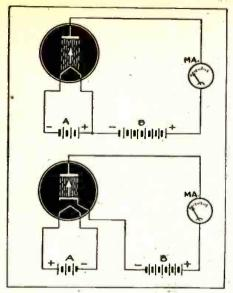
Fig. I (top), and 1-a (bottom)—Electron flow from filament to plate in a vacuum tube, and the same action in an indirectly-heated "cathode-type" tube a later development.
