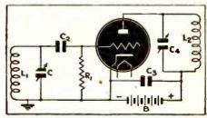
Fig. 8-a.—The tuned-grid-tuned-plate oscillator.
