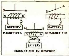
Fig. 4.-How we can change the poles of a magnet.
