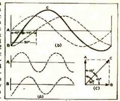
Fig. 5. Effect of adding two out-of-phase currents.
