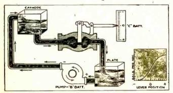
Fig. 2-b—Hydraulic analogy of the electron tube, showing effect of grid. Fig. 2-c—(Graph in corner.) A hydraulic application of the Fig. 2-b graph, with gallons of water per second instead of milliamperes.
