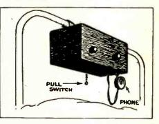
A canopy pull chain switch is mounted in the bottom of the cabinet as it is more convenient to operate while lying down than a turn or toggle type. The switch can be taken from an old lighting fixture or bought at an electrical supply store.
