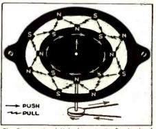
Fig. 7.—Arrowhead N is drawn to the S-pole ahead and is pushed forward by the N-pole behind it.
