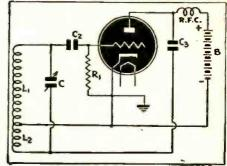
Fig. 7.—Shunt-fed Hartley, another standard circuit.
