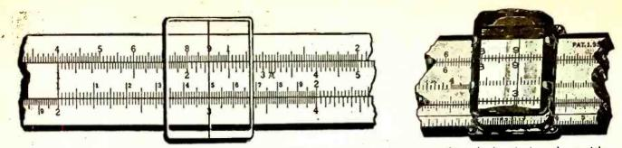
A magnifier makes it easier to read accurately. The rule is now set up to multiply 2 by 1.5, to divide 3 by 1.5, or to obtain the square root of 9.
