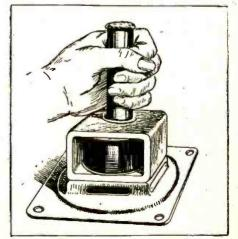
Fig. 5—How to remove some speaker coils.
