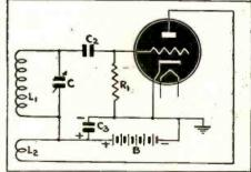
Fig. 5-a—The grid leak may go from grid to cathode, sometimes with an R.F. choke in series.
