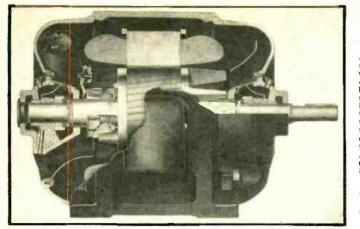
Another type of motor much used in radio work is the single-phase alternator illustrated here. Working on the same principle as the D.C. motor described; the manner of opera-tion is different, to suit the different type of current used. A de-tailed description of A.C. motor principles may appear in a later issue of RADIO-CRAFT.
