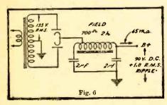
voltage on the power transformer with resulting increase in copper. The ultimate desirability of choke input may be determined by considering the availability and costs of copper and steel vs. the materials for paper or electrolytic capacitors.
