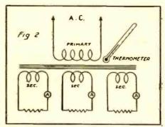
because in actual operation the transformer is usually inside a closed cabinet and the cooling will not be so effective. When conducting tests, a piece of plasticine should be used to bed the thermometer on to the windings. If the test is run for a considerable time the temperature of the core can be measured. The tests should be taken with full-load currents in all windings,
