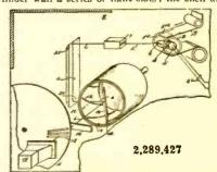
the barrel being relatively movable and the slots of one part being angular as to the slot of the other and cooperating therewith to form a travelling light aperture for light from said source to the exterior of the shell.
