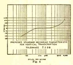
that this is the final recorded characteristic and, consequently, must absorb the various irregularities in the entire recording channel. The particular pre-emphasis as shown in this case is a 100-microsecond curve for the treble section. The curve is essentially constant amplitude below 500 cps and in addition there is a slight amount of pre-emphasis below 100 cps.
