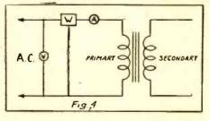
the V.A. (Volts-Amps) of the primary and the wattmeter gives the actual watts consumed. Except for unity power factor these values will not be equal and when measured give an approximation of the
