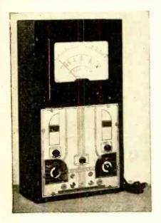
of 40,000,000 to 1. In designing this multi-purpose instrument, RCP engineers elim-inated danger of shock on low-capacity measurements. There are no test leads to short, and no resetting is necessary when changing ranges. The meter cannot be damaged by accidental connection across a live resistor or by using a low range on high readings. Error due to line voltage fluctuation is eliminated by a VR105-30 regulator tube and associated circuits.
