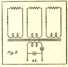
plied in this case should be very much less than the normal line voltage so that the current flowing in the secondary is limited to its normal full-load value (which can be measured with a meter in series with the winding). Alternatively, the primary voltage can be arranged to give the calculated primary current on full load.
