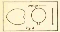
This cardioid pattern principle makes it possible to employ a simple scheme for di-rection finding purposes. A loop can be in-stalled in aircraft with the loop plane set at right angles to the fuselage or parallel with the wings. Then, when the pilot is flying the ship in the direction of an incident wave or station, a minimum bearing will be obtained. It is necessary that he swing the nose of the ship slightly off course to left or right from time to time in order that the bearing be checked.
