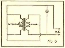
mined, if the primary and secondary are connected in series and placed across the A-C supply as shown in Fig. 3. The voltage across the secondary will be smaller than the line voltage when the windings are of the same polarity. When the polarities are reversed, the secondary voltage will be greater than the line voltage.
