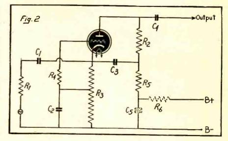
ground potential by the same amount, less the amount of grid bias required for normal operation. This is most conveniently done by connecting the lower end of the grid leak to a tapping on  $R_3$ . The grid condenser  $C_2$  and the grid leak  $R_4$  can have normal values.
