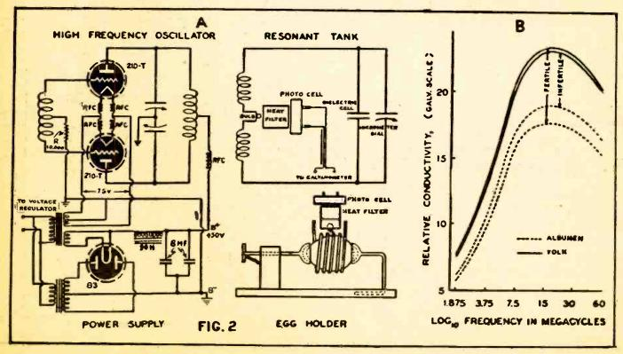
worm drive and dial permitting settings of the condenser capacity to an accuracy of ±0.002µµf. In the center of the tank coil was mounted a small 2.3-volt flashlight bulb above which was a photronic cell protected by a copper sulphate heat filter. A galvanometer shunted to critical damping registered the intensity of the light from the bulb.
