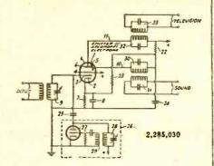
loosely coupled to the control grid for impressing a heterodyne frequency thereon, and a pair of impedances each included respectively in the cir-cuit of the auxiliary cathode and in that of the anode and each having respectively a high value for one of the intermediate frequencies resulting from the interaction between the heterodyne frequency and each of the signal-modulated carrier frequencies.
