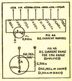
scale meter deflection requires 50µa. or .125 volts, we know that a voltage drop of .25 takes place across the meter-resistor (Continued on page 58)
