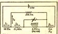
FIG. 6A. RX10 RANGE REARRANGED FOR CAL-CULATING VALUE OF ZERO-SET RESISTOR
