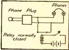
The keying is very clean therefore and is easily readable, being very sharp. Be sure you have the right type of relay for this circuit, one that is normally closed.—Frank-lin Williams, Woule. Glendale, Calif.
