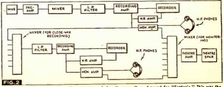
Fig. 2. Block diagram of the equipment set-up during the recording of sound for "Fantasia." This was the arrangement of the apparatus at the Academy of Music, in Philadelphia, Pa. Items L.P. are low-pass filters; N.R. Amp., noise-reduction amplifier; H.F. Phones, high-fidelity phones.
