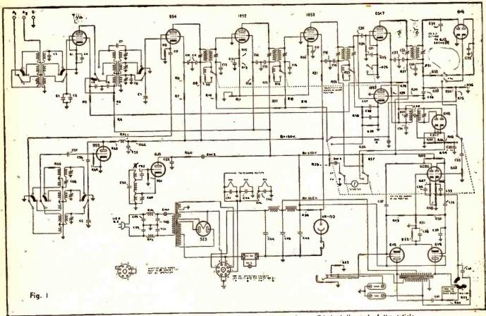
Schematic diagram of the S-27 receiver. All values of circuit components are listed at the end of the article.
