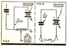
TO SAVE time when adding phonograph pickups to radio receivers, place the pickup across the volume control, as shown at A in the illustration above.
