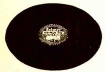
METAL-BASE, acetate-coated, blank recording disc which has a patented stroboscopic label which gives an instantaneous check on the turntable speed each time the record is played. The label permits the speed to be checked at 78 r.p.m. under a 60-cycle light. Available in 6 in. and 10 in. sizes.—Radio-Craft
