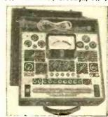
SERIES 954 is a combination dynamic mutual conductance tube tester and a 37-range A.C.-D.C. set tester. Designed for use with both F.M. and A.M. receivers as well as with television receivers. Its single meter is of the 20,000 ohms/volt type with ranges of 6,000 volts A.C.-D.C.; 60 microamperes; 12 amperes; and, 60 megohms. Available in counter type, panel as well as portable and rack mounting models.—Radio-Craft
