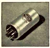
NEW series of dry electrolytic condensers in metal cans which may be plugged into a socket as easily as a radio tube. Known as Type DO, they can be easily removed for both testing and replacing. To insure rigidity of mounting for marine and aviation service, straps are available for holding the condensers in their sockets.—
