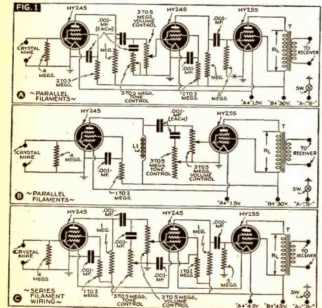
Fig. 1. Typical circuits for use with the new tiny pentodes, both series- and parellel-filament connections are shown in these audio-frequency amplifier circuits, which are especially suitable for use in hearing-aids. Output transformer T must be designed to match whatever earphone is selected. In Fig. 1, 67 45 V. Bis cell at X. In Fig. 2, choke Ch. measures 200 to 300 henries. In Figs. 1 and 2, R-L equals 50,000 ohms; in Fig. 3, 40,000 ohms.
