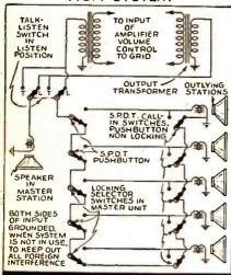
THE main feature of this circuit is a quiet, noise-free master station, if the amplifier used is constructed for minimum hum. Shielded wire is not used on the outlying station runs as both sides of the primary of the input transformer are grounded when the system is not in use. When an outlying station calls in or is selected at the master station, the ground circuit, in series with all selector and call-in switches, is broken.
