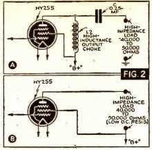
Fig. 2. Optional-circuits. Circuit A is recommended for use with high-impedance crystal (or magnetic) receivers. Condenser C isolates the "+" potential from the receiver circuit. Diagram B is for use only with low-impedance magnetic receivers.
