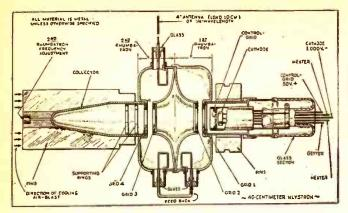
Cross-section of the 40-centimeter Klystron. The Klystron is composed of 2 Rhumbatrons. The 1st Rhumbatron "bunches" the electrons and passes them to the 2nd Rhumbarton, the "catcher," which transforms the electrons into radio energy at ultra-high frequencies.
