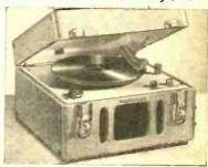
A all-electric record player, complete in itself, comprises phono turntable, pick-up, built-in amplifier and loudspeaker—all in a single carrying case. Motor is 78 r.p.m.; table is rini-driven. Player has record compartment for eight 10-in. records. Designed for 110-120 volts, 60 cycles, A.C. only. Weight, approx. 14 lbs. Power output, 2 watts.—Radio-Craft
