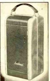
Sentinel camera-type portable receiver. Overall cabinet dimensions, 4 7/16 x 4 x 8 13/16 ins.; weight, complete with batteries, 4/2 lbs. Since the loop antenna is built into the receiver, it is necessary to rotate entire set for maximum signal pick-up.
