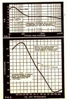
on the higher frequencies inherent in F.M. transmission. This is accomplished by a resistance - capacity combination in the discriminator load circuit where it is switched out automatically when the receiver is switched to the A.M. position.
