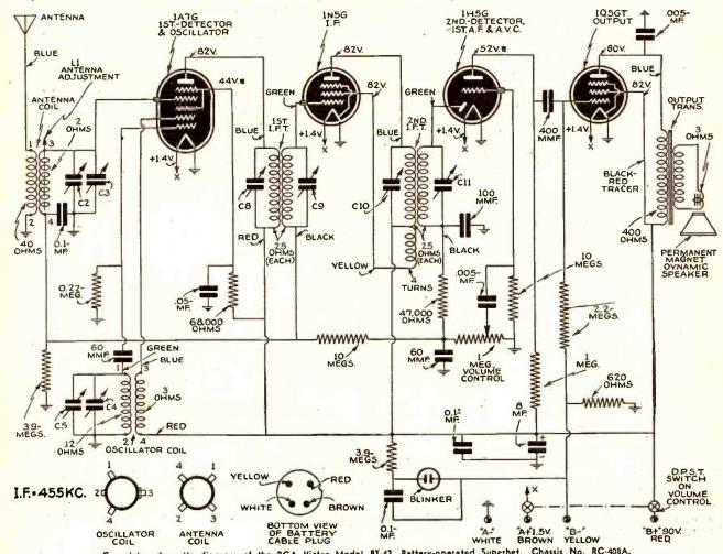
Complete schematic diagram of the RCA Victor Model BT-42, Battery-operated Superhet., Chassis No. RC-408A.
