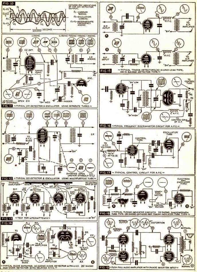
Typical circuit details of modern radio receivers which the Serviceman is called upon to diagnose and repair. The visual dynamic analyzer by enabling the Serviceman to actually SEE the signal cuts the time necessary to localize the receiver faults. The oscilloscopic patterns shown in the diagrams are pictures of the signal as it appears in various sections of a receiver circuit.
