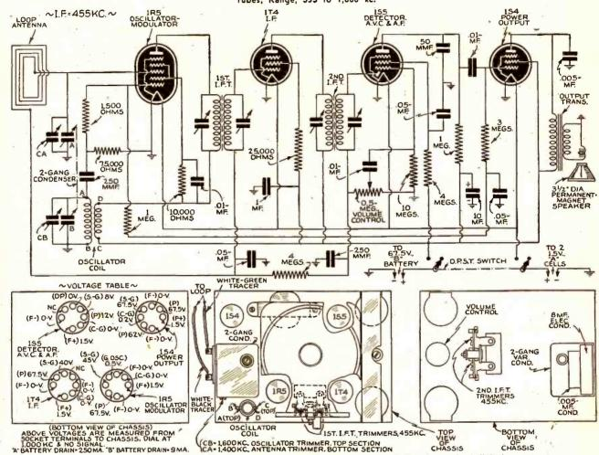
Complete schematic diagram of the Sentinel "Lightweight Portable" camera-type, 1.4-V. Battery set with built-in loop antenna.
