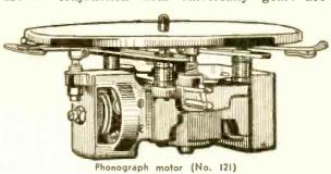
THIS motor was designed to meet the powered public-address systems, operating from either a six-volt storage battery or 110 volts A.C. A small D.P.D.T. snap switch makes quick changeover The current drain is 2.8 possible. amperes.
