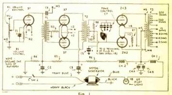
Schematic circuit of the amplifier. The "C" bias for the two 2A3 tubes are obtained from a separate power unit to insure fixed bias when the input signal is large. The tone control is a single unit, and each of its fixed condensers may have a capacity of approximately .001-mf.
