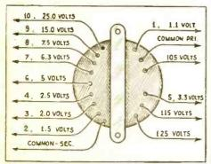
Fig. 3 Details of the transformer leads.
