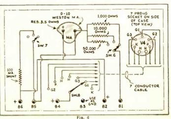
Schematic of the voltmeter-milliammeter section.
