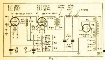
Circuit of a direct-coupled amplifier using a 27 (or 56) feeding a 47.
