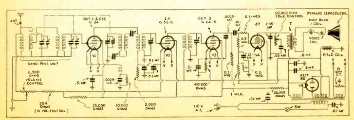
Fig. 1 Schematic circuit of the Majestic IS before the Change.
