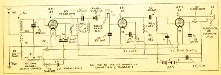
Schematic circuit of the receiver. See Fig. A for layout.
