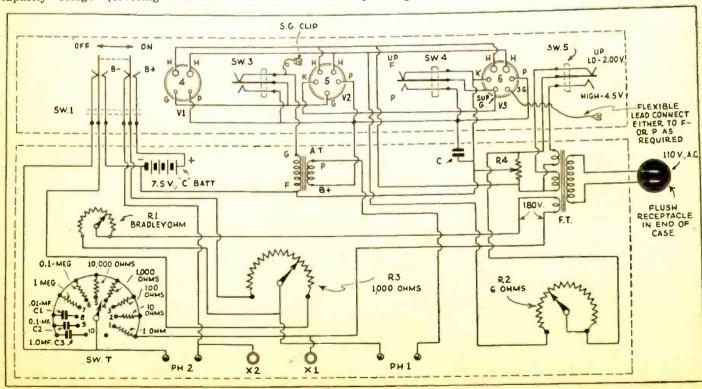
Fig. Schematic circuit of the tester. See Fig. 4 for details of the volt-milliammeter.
