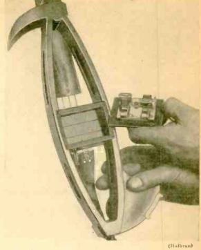
The works: vibrations from a special bridge induce an E.M.F. Ir the coils of the winding which, in turn, are amplified.
