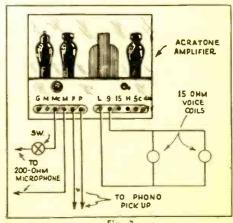
A detail drawing showing the connection of the binding posts.
