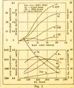
Fig. 2 Characteristics of the 12A5 for a 200-volt "B" supply.
