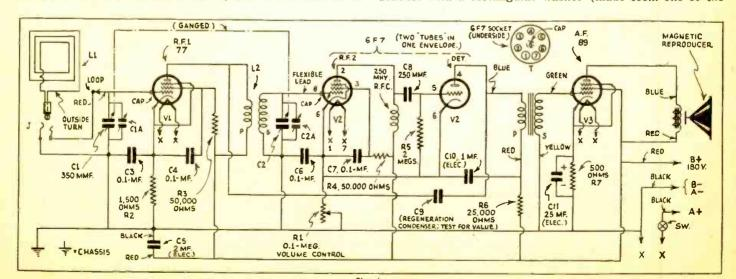
Schematic circuit of the RADIO-CRAFT Loop-Portable Receiver. After completely assembling and testing the set, it is a good plan to experimentally determine whether any of the component values may be changed to advantage, in accordance with the characteristics of individual tubes, R.F. transformers, etc.
