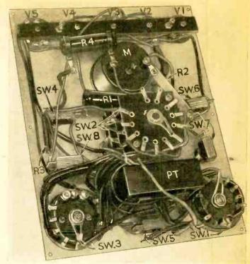
Fig. B. Rear view illustrating the location of the parts. See Fig. I.
