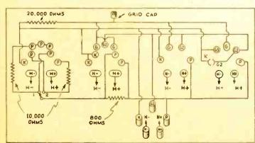
Fig. Q. 205A Schematic circuit of the Na-Ald type 950-XYL adapter.
