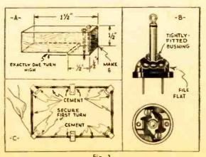
Details of construction. At B, the assembly of the plugadapter; A, loop-wire blocks; C, loop winding procedure.
