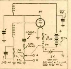
Schematic diagram of the oscillator
