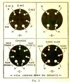
At A, socket connections of the I2A5; at B, connections for the I-V rectifier; at C, connections for the 53, class B tube; and at D, connections for the 25-S.
