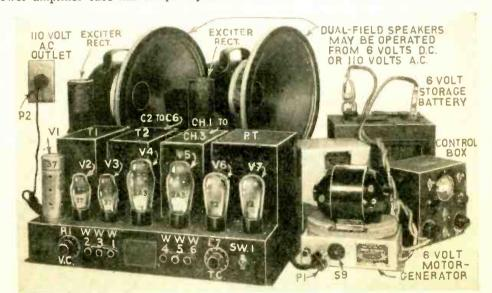
Front view of the Coast-To-Coast 20-watt amplifier showing the amplifier, special speakers, motor-generator unit, control box, and storage battery.
