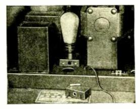
Here RCA Victor adds line-coltage controls to its sets. The case of installation is well illustrated in the sketch below.
