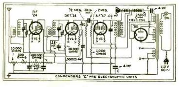
Fig. 2 Schematic circuit of the Peter Pan Model 84 Midget Set,
