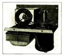
Fig. C The "Autoverter," showing step-up transformer, filter, and motor-driven interrupter.
