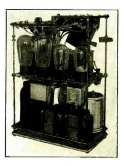
Fig. B Interior view of the amplifier cabinet of the portuble sound recorder.
