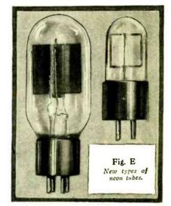
free illumination is obtained by generous spacing between the electrodes and by proper gas pressure. The tube draws 25 to 30 ma. at 200 volts; its impedance is 15,000 ohms. One tube has a cathode  $1\frac{1}{2}$ in. sq.; the other, 1 in. sq.
