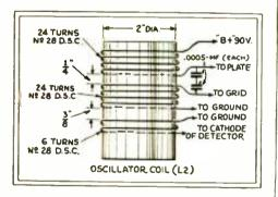
Fig. 2 Oscillator details. All coils are wound in the same direction.
