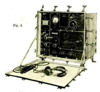
Lifeboat Model ET 3677 Radio Transmitter-Receiver.
