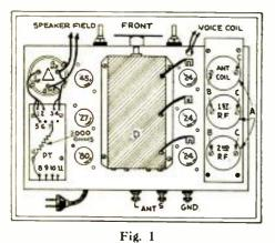
Top view showing parts layout of the Remler "14". The P.T. connections have also been indicated.
