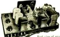
Back view of seven tube screen grid tuned Radio frequency receiver -only one of many circuits you can build.
