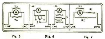
Left. The shunt R2 is connected directly across the ammeter. Center. At A and B are shown two methods of connecting several shunts. Right. The resistor R1 is inserted in series with the meter to increase the size of shunt required.
