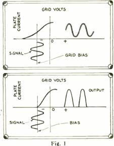
Above. Graph of push-pull operation. Fig. 2 Below. Push-push represented by graph.
