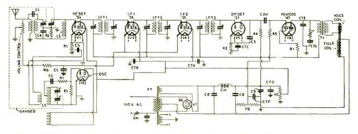
Schematic circuit of the General Motors receiver most commonly referred to as the Little General: the same chassis, however, is used in a number of other models, as indicated at the head of this Data Sheet. Decreasing the effective resistance across the primary of the input R.F. transformer by moving the contact arm toward the antenna, results in an increase of the resistance in the eathode circuits of V3 and V4, thus increasing the control-grid bias of these tubes.
