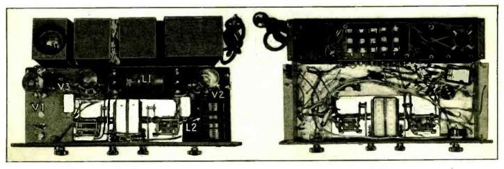
Fig. B Top view of the receiver. Note the excellent arrangement of the parts and the right-angle positions of L1 and L2.
