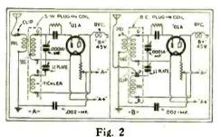
At A, a standard short-wave connection. At B, circuit changes for longer wave reception.
