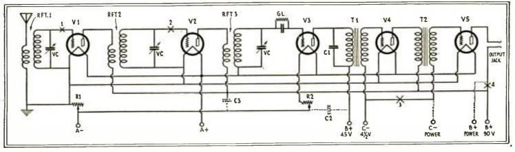
(Q. 43) Schematic circuit of a standard 5-tube radio set of early wintage. Improvements in this circuit design are described in the accompanying text and Xs indicate the points of alteration.
