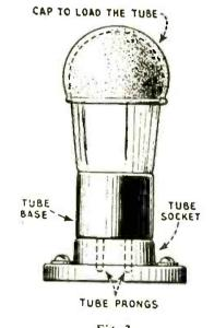
Fig. 3 The "boxel arrestor" used with a microphonic tube simply keeps it from vibrating freely, and thus shaking its loose elements.
