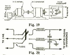
The motor-generator combination will require a filter on each side, as shown above. The three-wire system is grounded in the center, but even here a choke coil may be helpful.
