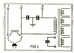
Line-connections of the Colonial "31.4C": 1 (maroon) and 8 (blue-white) lead to set switch; 7 is yellow.
