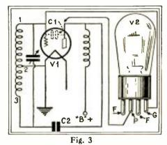
The burnt-out tube at the right has the same capacity as 1'1, and therefore is an ideal neutralizing condenser.
