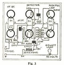
The filter circuit used to suppress generator ripple in the D.C. receiver. An old trans-former secondary will serve as the choke.
