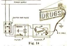
A flashing sign, operated by a thermostatic switch, will require a filter of greater currentcarrying capacity than a small motor. cause interference because their operation depends upon the "make and break" of the circuit by means of contacts.
