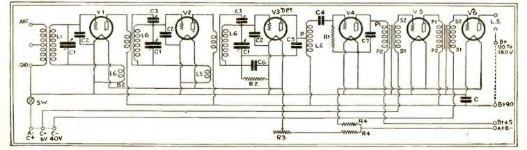
(Q. 42.4) Schematic circuit of the Crosley "RFL-90" receiver mentioned by Mr. Garriott; note the system of neutralization,
