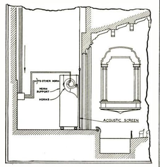
The general layout for sound motion pictures in a modern theater is represented here, and in the upper right corner of the next page, representing the relative positions of projection room and screen. The connections between the two are represented by arrows. The horns must be placed with regard to the acoustics of the theater.
