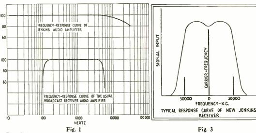
The efficiency of the new Jenkins' amplifier for television, compared on a logarithmic scale with that of a receiver good enough for all andible reception,
