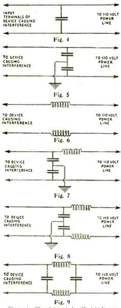
These six filter types deal with interference of increasing degrees of difficulty. In each case, the problem is finding a capacity which will by-pass the R.F. current generated by the device served, because of the impedance on either side of it. In Fig. 6, the inductances may cause the self-capacity of the device itself to act as a sufficient by-pass.
