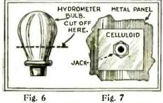
At the left, a simple means of obtaining a tube-cap to stop microphonic noises. Right, a hawdy means of insulating parts from a metal panel.
