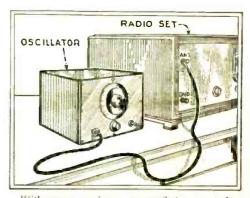
With some receivers, an oscilutor must be coupled directly to the circuit, as shown. It is sometimes possible to obtain a sufficient signal, for balancing and testing, by inductive pick-up.
