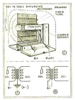
In place of grounding the core of an A.F. transformer, as at A, Mr. Link connects it to "B+" as ut B. In a transformer which he dissected, electrolysis was apparent from primary to core. as at C.
