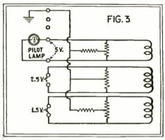
Center-tap, biasing and pilot-light connections of the "Radiola 18AC."
