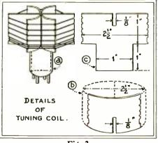
Fig. 3 Mr. Auble's home-made coils, of which the smallest is shown here, are wound on a form "turned inside out?" to give love losses, as described elsewhere.
