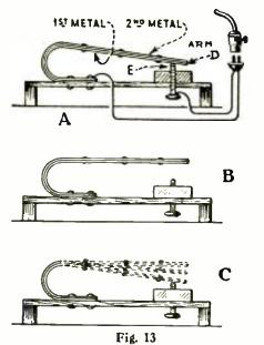
The alternate heating and cooling of a thermostatic contact may set up rapid vibrations which cause very troublesome interference.
