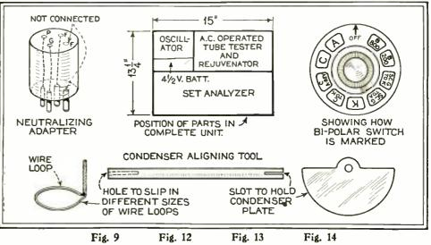
Fig. 9 (upper right). The markings on the bi-polar switch. Fig. 12 (upper left). Adapter to be used when neutralizing. Fig. 13 (lower half). Aligning tool for balancing variable condensers. Fig. 14 (upper center). Placement of the electrical equipment of the tester.
