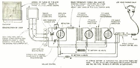
Fig. 25 The schematic circuit shown above is that of a loop-operated regenerative receiver, well adapted to the location of interference. The constants are given in the sketch. Such a receiver should be completely shielded; it may be constructed very compactly and lightly for the work described.
