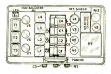
schematic circuit. Magnetic, and other makes of dynamic, reproducers connect, as shown, from plate to plate of the power tubes. At a line voltage of 110, the primary of T should receive about 88 volts. When making any changes in the receiver connec-tions or parts, it is well to watch the regu-lator R12. If it heats to a visible red, the plug should be pulled and circuit checked. anno
