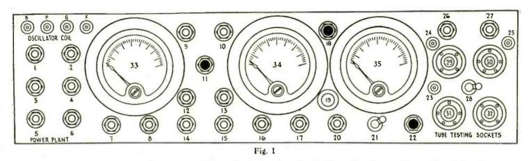
Layout of pauel of the "instrument tray." One pair of sockets test tubes directly, and the others permit use of the adapter plug.
