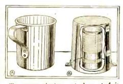
The common aluminum cup shown at A is transformed quickly into the R.F. coil shield at B. A "tin" cup, being made of iron, is not so well suited for this purpose.
