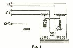
How a single resistor biases five tubes in the Bosch "28" and "29."
