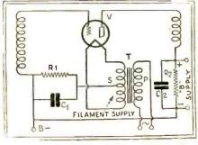
The elements of the voltage supplies of an A.C. filament tube; check first speaker; then, tubes voltages, and receiver circuits, says Mr. Myers.
