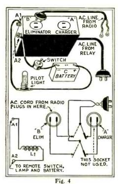
There are many old set-charger relays, discarded by owners of electric sets, which are well adapted to provide remote-control devices for turning the set on and off.
