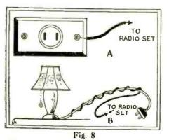
The pick-up from the light-line, obtained in either of the coupling methods shown above, will often give excellent reception and obviate the trouble and expense of an aerial.
