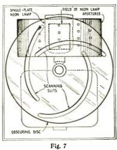
The mechanism of the new Jenkins visual reproducer, shown from the rear in Figs. B and C.
