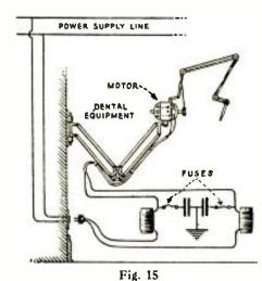
A dental motor, of a type which can be very annoying, is shown with a filter of the type of Fig. 8. The chokes may be home-made.
