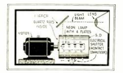
Fig. 6 A reflecting system, indicated here schematic-ally, was needed with the older quartz-rod drum.
