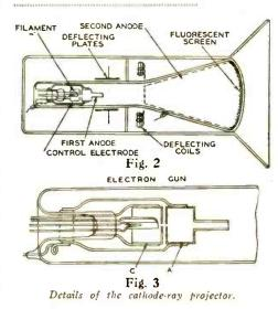
in his television receiver; while the variations of the intensity of the ray—with the voltage on its controlling element—affect the brilliancy of the light on its screen, and produce the bright and dark contrasts necessary in a television image.
