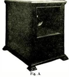
The radiovisor in its plain cabinet; the image is formed at the end of the "shadow box."
