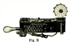
The "instrument tray," protective lamp, oscillator "spiderweb" coil, etc., are shown here. The tip-jack layout is on the front.
