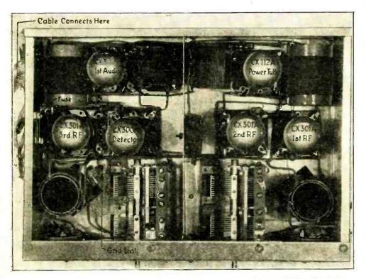
Internal appearance of the compact, completely-shielded chassis of a practical automobile radio receiver. It is mounted, in an inverted position, under the instrument board shown above; and all its leads are carefully protected against ignition interference.
