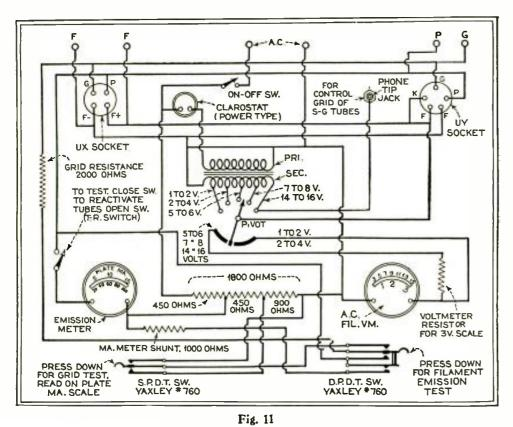
Schematic circuit of the tube rejuvenator and tester. Panel size is 61/4x11 inches.
