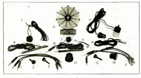
Fig. D The numerous accessories required to complete the equipment comprised in the "Diagnometer"; most of them are known to the experienced Service Man but a few are special.
