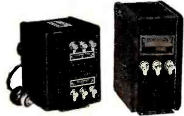
Here is a power unit that will satisfy the ever increasing demand for improved quality of reception. A split secondary 550 volts either side of center, makes possible full wave rectification, using two 216-B or two 281 tubes. Current capacity, 130 milli-amperes. The low voltage secondary, 7 1/2 volts, will supply two UX-210 power tubes, enabling the use of push-pull amplification in the last audio stage.
