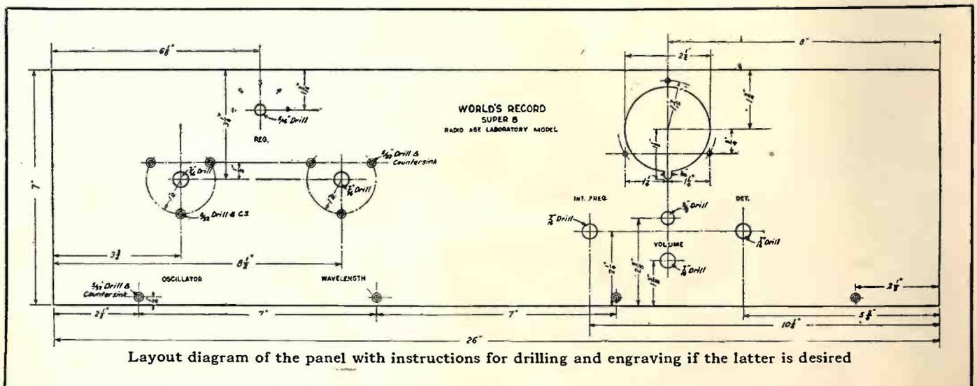
Layout diagram of the panel with instructions for drilling and engraving if the latter is desired
