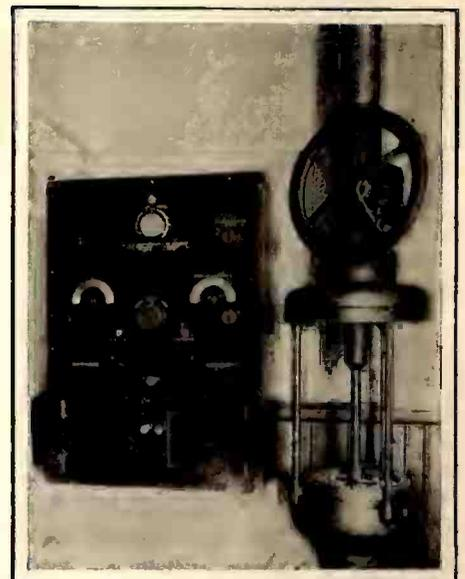
Rotation control of the radio compass loop and the receiver used for picking up directional signals.
