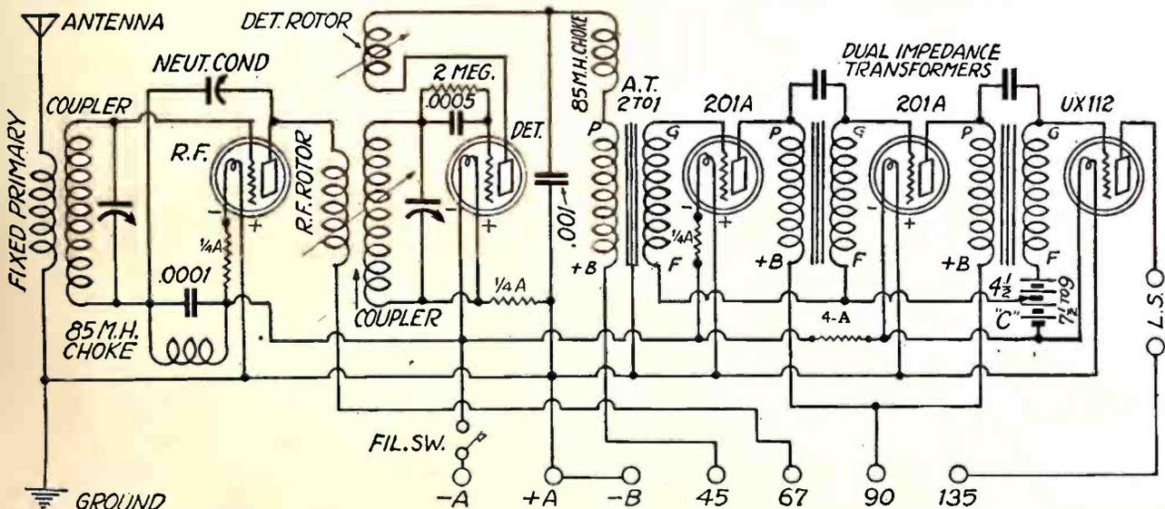
Schematic circuit of the Dual TC receiver from which the set may also be wired
