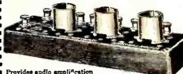
Provides audio amplification with minimum distortion. Bradlevmit molded resistors used in the Bradley-Amplifier do not vary with age and are not affected by atmospheric conditions. Can be used to replace transformer amplifiers in standard radio sets with decided increase in tone quality.
