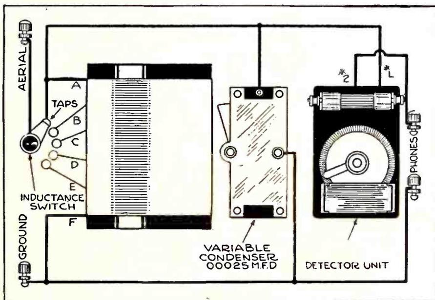
In order to show the extreme simplicity of the crystal set, we are reprinting the diagram above which shows the coil, condenser and detector unit. Taps are shown on the coil, although they are not absolutely necessary—a honeycomb coil of 50 turns, or 50 turns of bell wire on a 3 inch form, will suffice. Full details of this simple crystal receiver appeared in the August issue of Radio Age (1926) page 17
