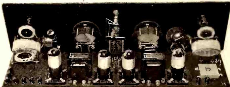
Rear panel view shows the two Micro-couplers, sockets, and all other parts used in this set
