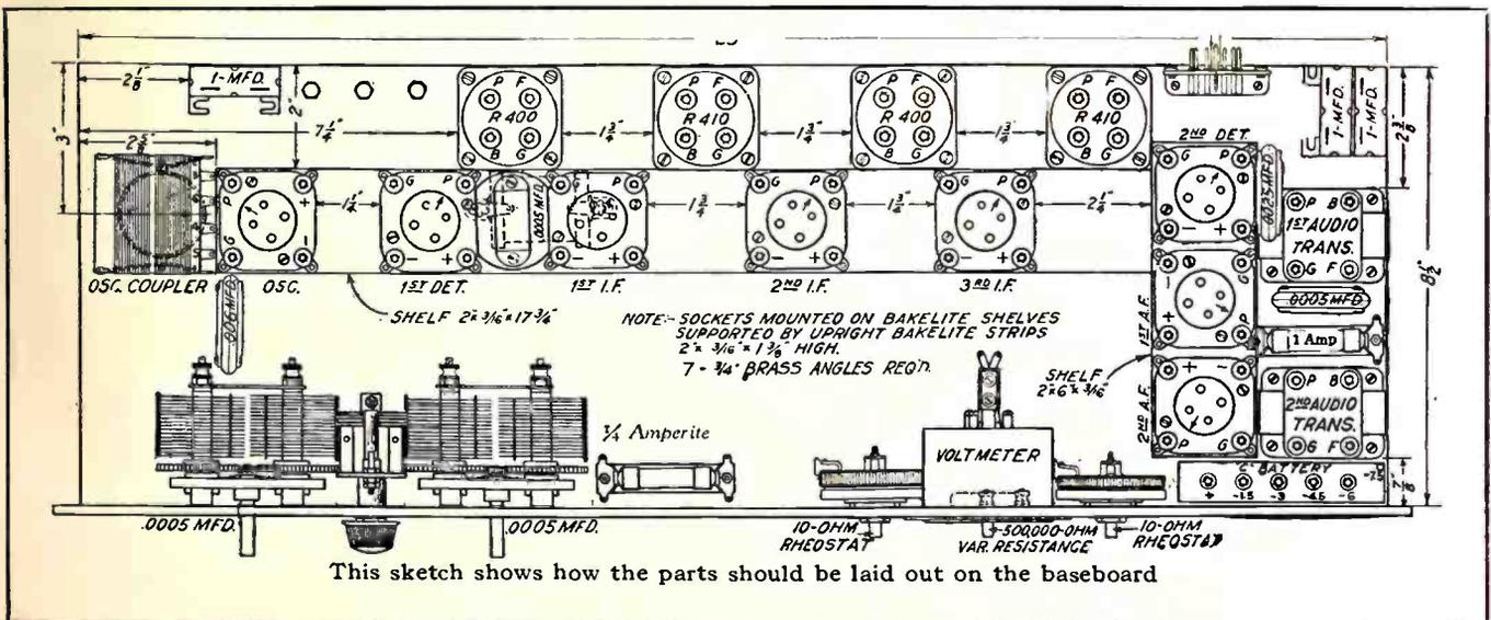
This sketch shows how the parts should be laid out on the baseboard
