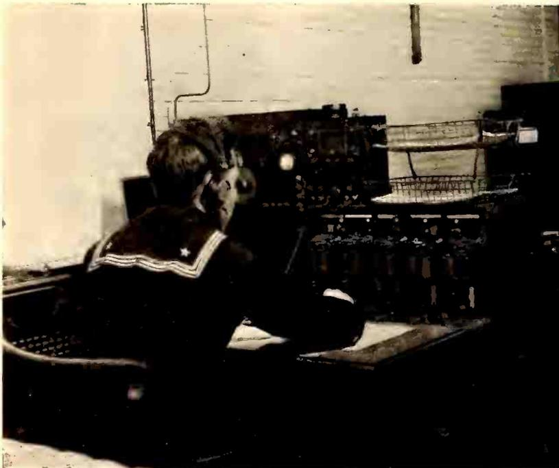
This operator is located at the control station which receives bearings by land wire from compass stations, plots these results and sends the correct bearing to the vessel requesting such service
